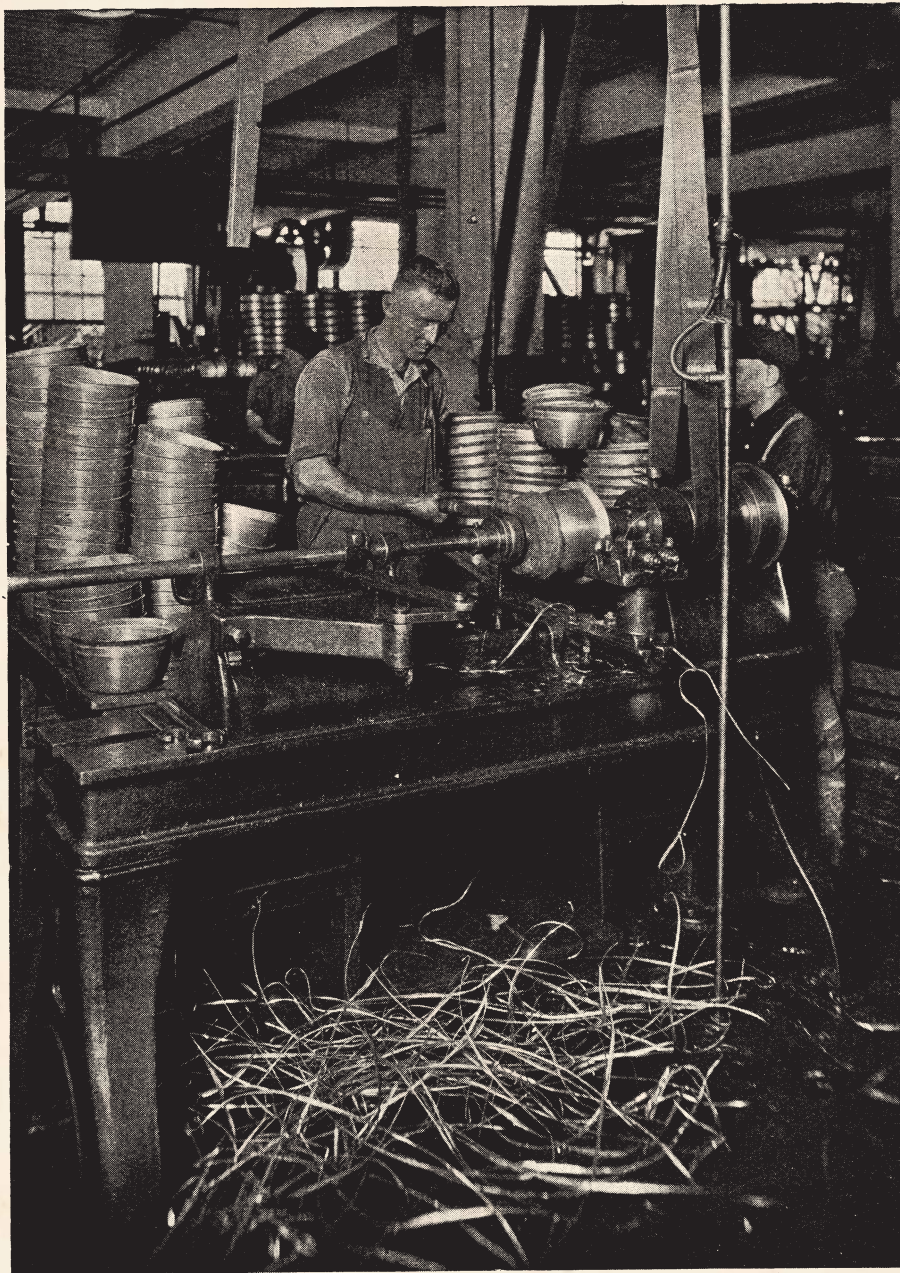
Fig. 1.—OPERATING TRIMMING AND BEADING TOOLS ON ALUMINIUM SAUCEPAN
