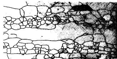
Highly magnified crystalline structure of ferritic stainless steel
