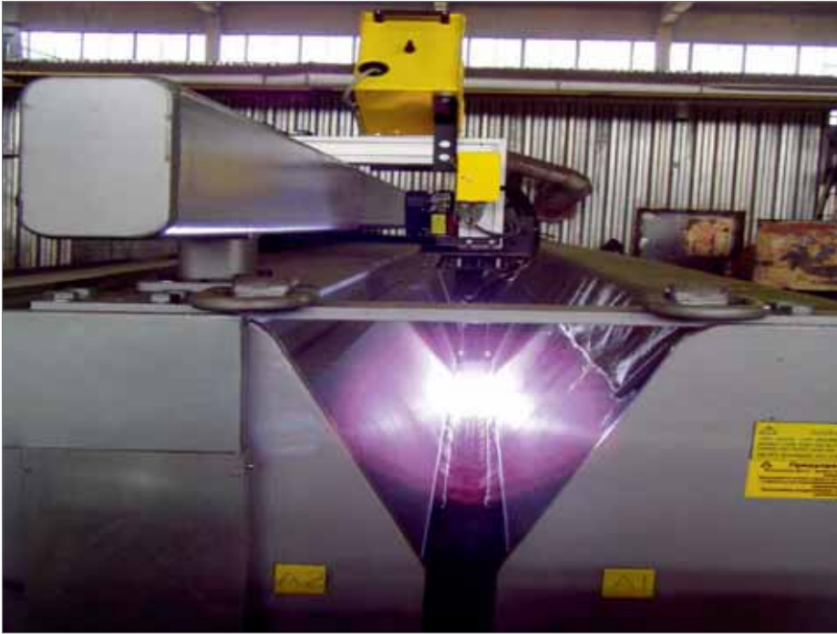
Figure 2. Process plasma welding of plates with the ESAB FD60HP Plate Seamer.
