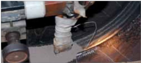
Figure 5. Narrow gap SAW.
