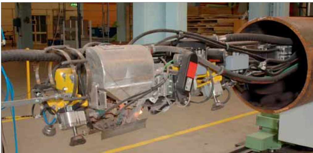
Figure 3. Internal longitudinal welding head (4 wires) in test phase, with 4 voltage pick up brushes with pneumatic cylinders in front and behind the welding head.
