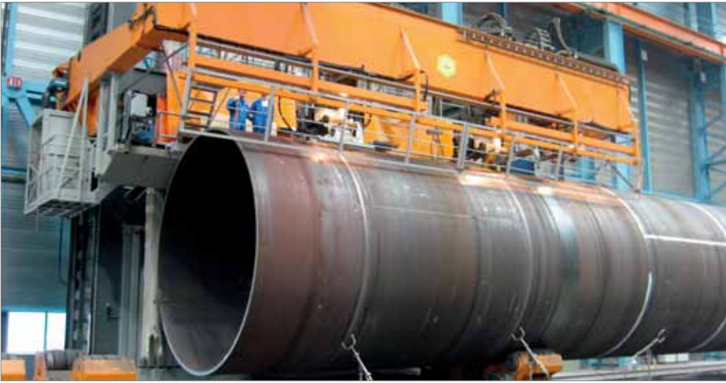
Figuur 8. Portal welder for circumferential welding, in operation.
