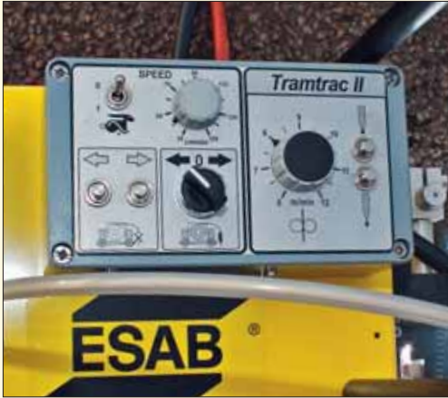
The control box features clearly marked symbols for wire feed speed, travel speed and start and stop welding functions, as well as wire inching.
