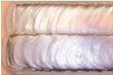
OK Band 7018, 90x0.5mm, 1000A/30V/13cm/min.
