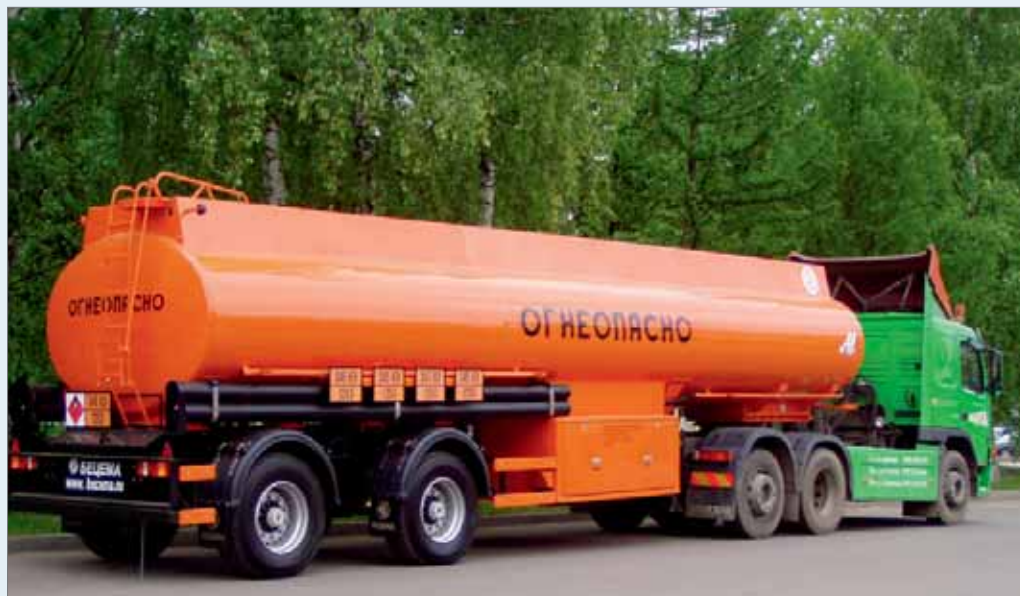
Figure 1. AlMg5 tank truck with a volume of 32.5 m 3 produced by ZAO BECEMA.
