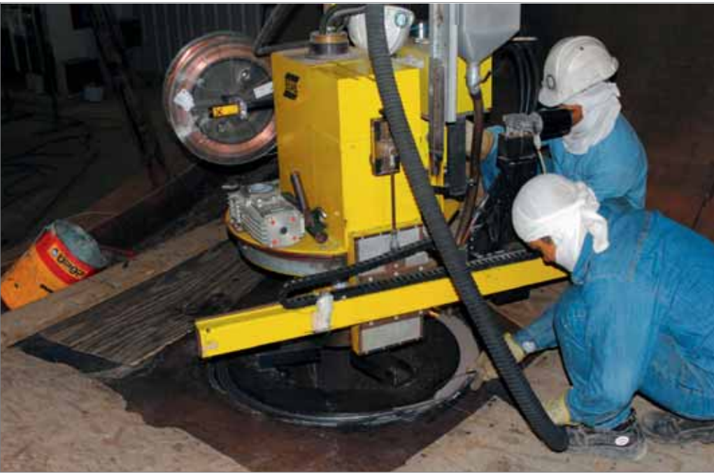
Figure 6. The A6-MHW automatic SAW welder for the welding of manholes and nozzles on cylindrical vessels.
