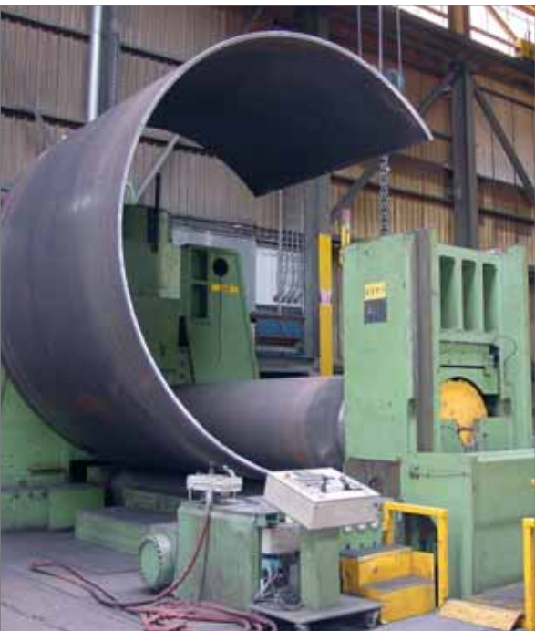
Figure 4. Rolling plates to shells; the first fabrication step in the production of monopiles.
