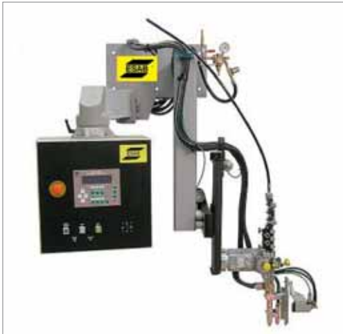
Figure 1. GMAW tack welding head, including PEH Control on swivelling arm and laser tracking system.
