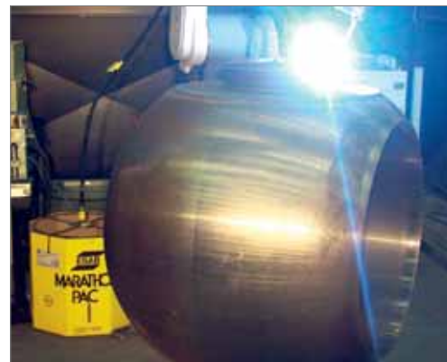
Figure 2. Robotic MIG cladding with ESAB's matt stainless wire fed from mini Marathon Pac.
