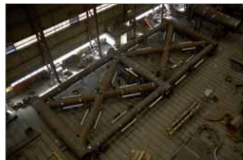
Figure 6. Lay-out of a row on the factory floor before welding – a precision job.
