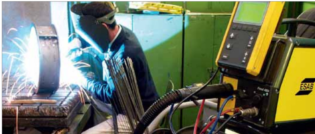
Figure 5. Flux-cored arc welding of an outlet ring, using FILARC PZ6166 and the AristoMig 500 inverter power source.
