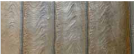
OK Band NiCu7, 60 x 0.5 mm, 800 A /29 V / 13 cm/min.
