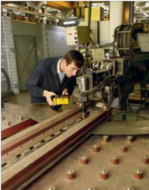
Figure. 2. Welding with one of the automatic TIG stations.
