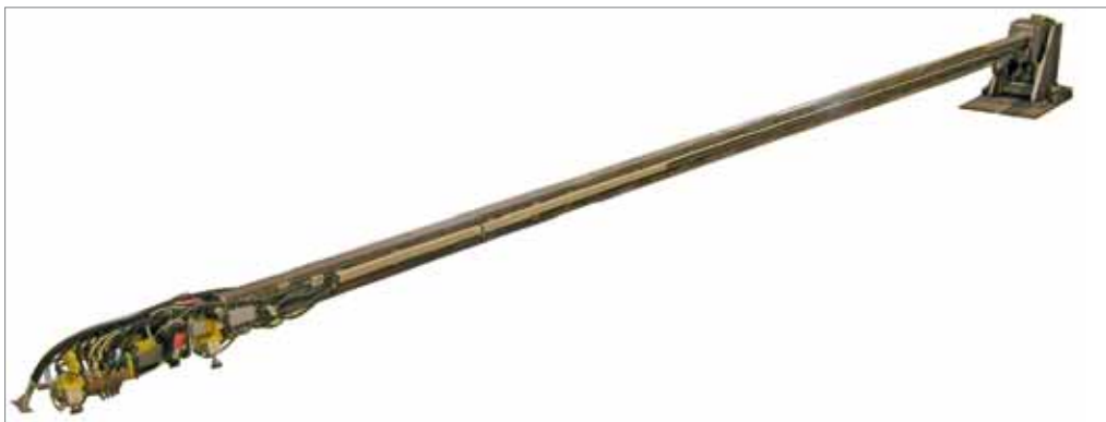
Figure 2. Internal boom (18m) with welding head for longitudinal pipe welding.
