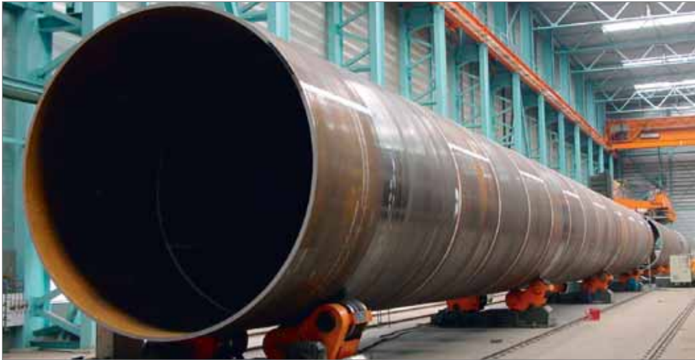
Figure 3. Monopile under construction. Note the longitudinal en circumferential welds.
