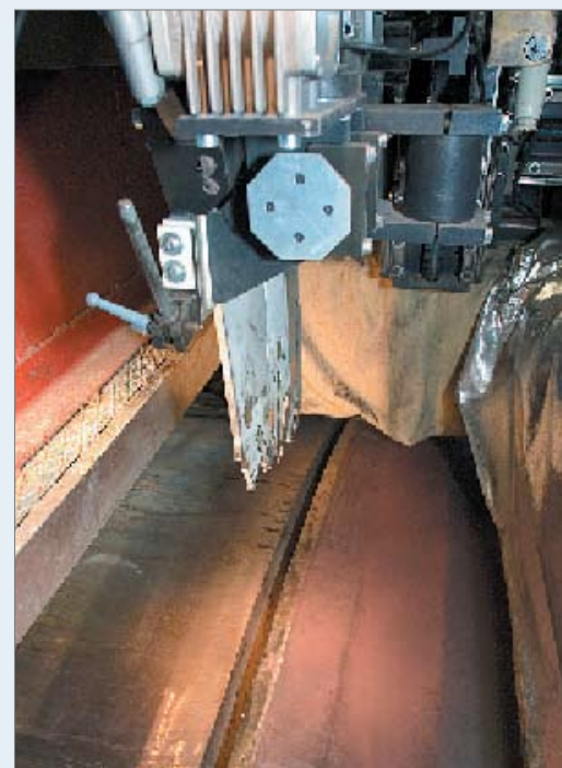
Figure 7. Narrow-gap welding of a circumferential joint. Welding wire is fed from 280kg drums to avoid costly downtime for spool exchange.
