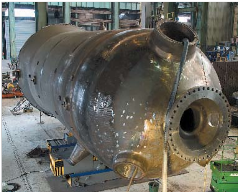
Figure 9. Completed heat exchanger.
