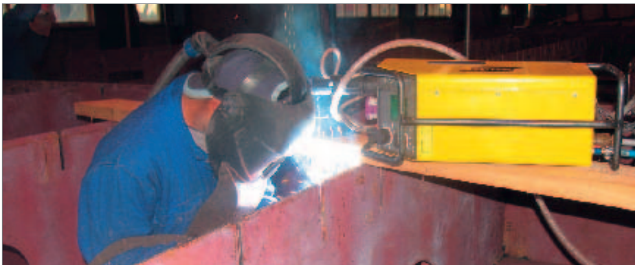
Figure 1. Origo Yardfeed 200 in use at Ferus Smit Shipyard.
