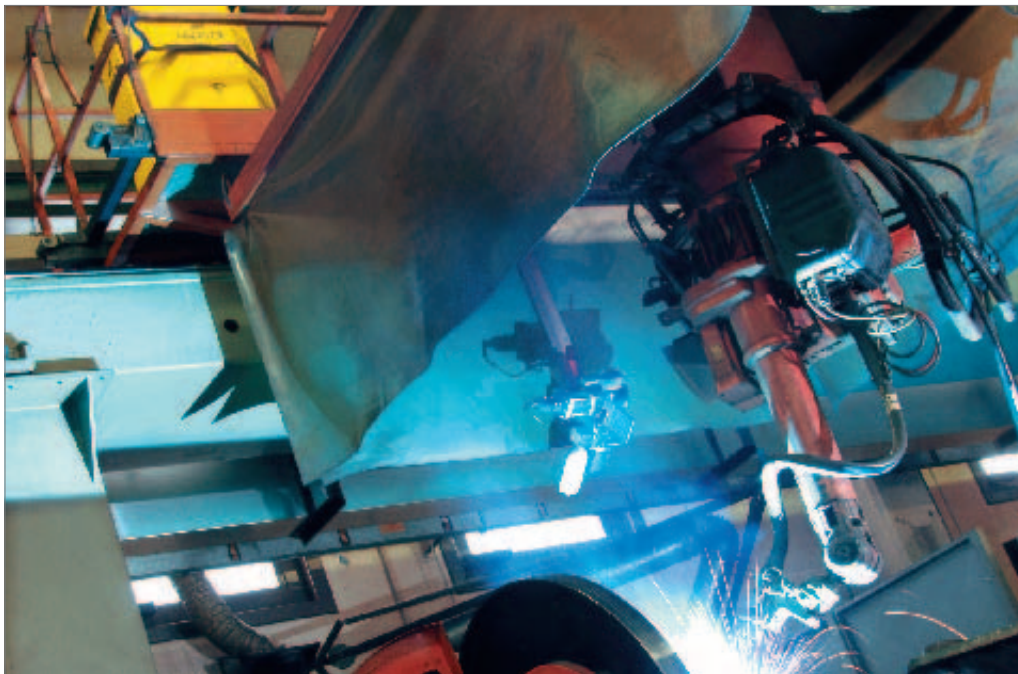
Figure 3. Production of crane front parts with a gantry robot, using OK AristoRod 12.50. The Marathon Pac is placed on a scaffold – the relatively long liner not standing in the way of problem-free feeding and a stable arc.
