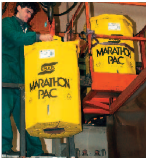
Figure 4. Lifting of a Marathon Pac by overhead crane utilising the certified lifting yoke.
