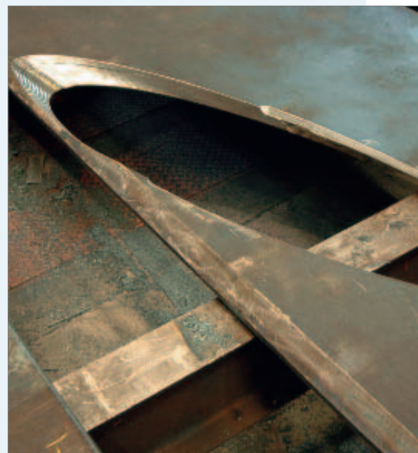
Figure 2. The oval orifices and their bevels; a challenging cutting job.
