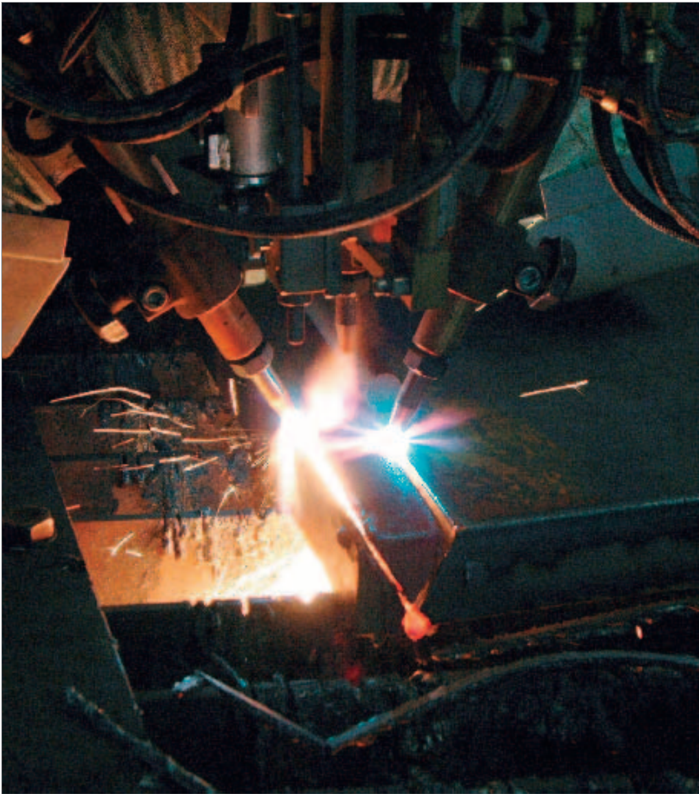
Figure 4. An infinitely rotating three-head oxyfuel burner unit suited for K-, Y- and V-joint preparations.
