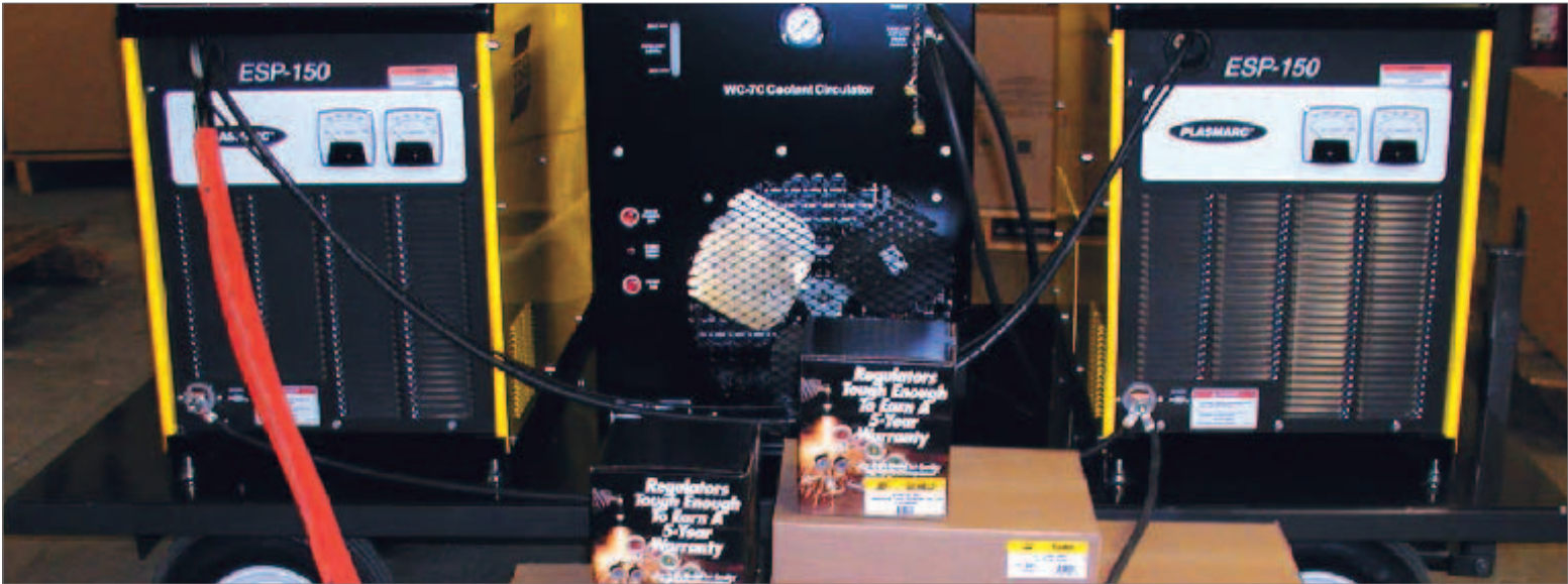
The Duce Pac ESP-150/PT-26. The system can be equipped as two independent 150A gouging systems or connected as one 300A gouging system.
