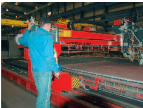
Figure 3. The SUPRAREX installation suited for material thicknesses up to 150 mm.
