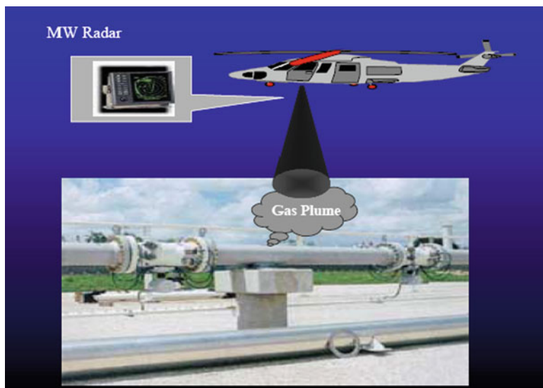
Fig. 12 Microwave radar for leakage location from reference [12]
