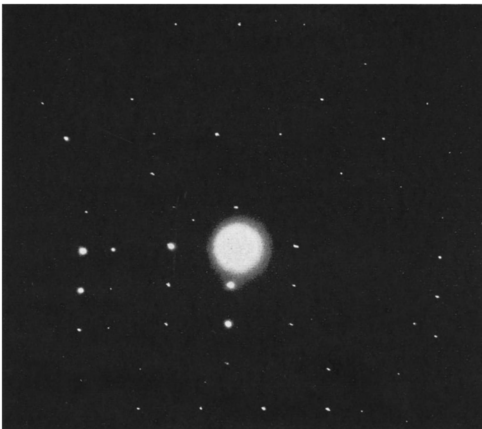
PLATE 4. Electron diffraction pattern from M_6C .
