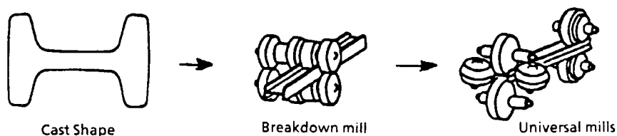
Figure 5.7 Process route for the rolling of cast beam blanks.
