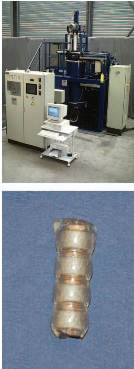
Figure 4.8 Medium-size hot isostatic press, used for production of diamond-impregnated beads and segments; and glass-encapsulated wire saw beads prior to final consolidation by HIP. (Courtesy of EPSI N.V.)
