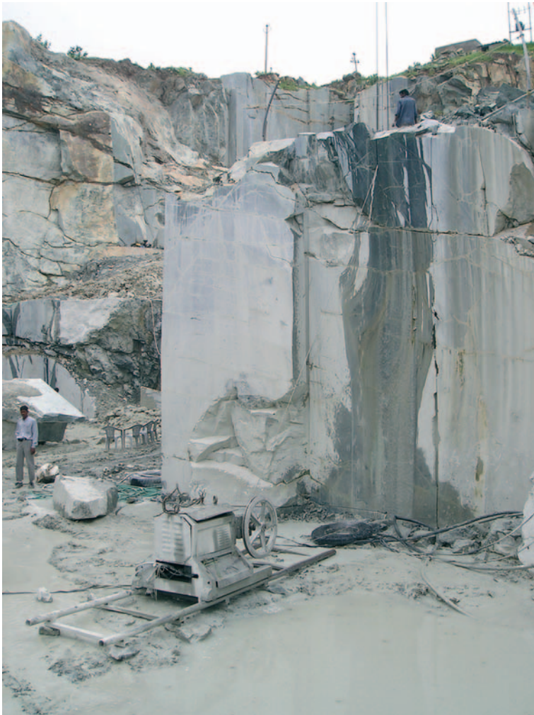
Figure 8.7 Cutting a large block from the rock face. (Courtesy of EHWA Diamond Ind. Co. Ltd., Osan, Korea)
