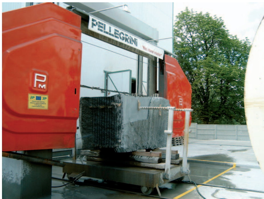
Figure 8.8 Stationary diamond wire saw for squaring stone blocks. (Courtesy of MC DIAM Sp. z o.o.)
