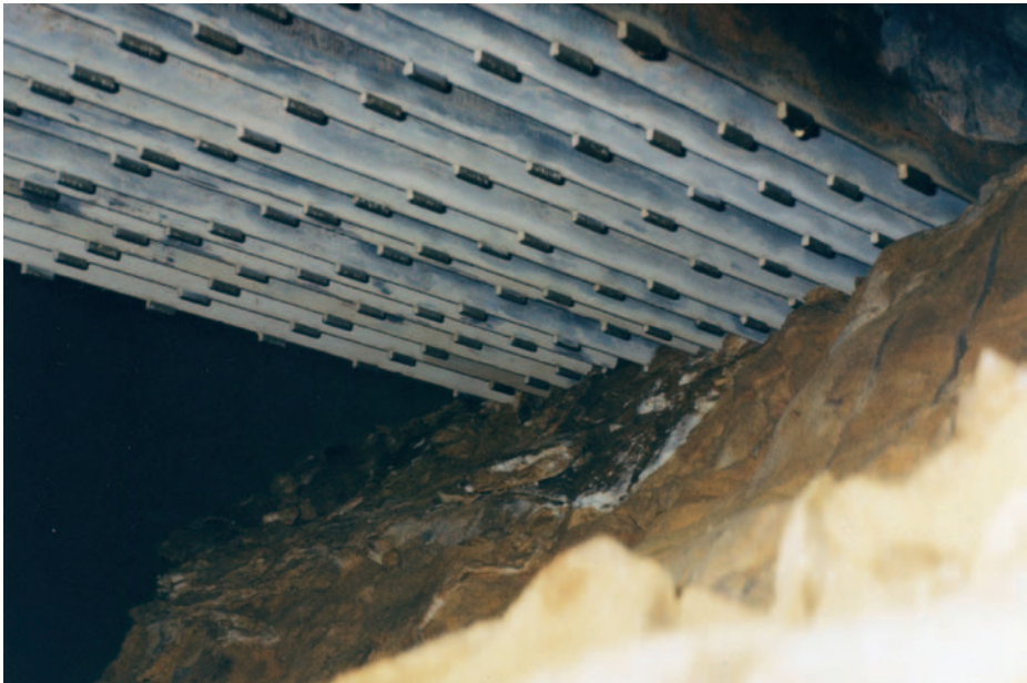
Figure 8.6 Frame saw, fitted with multiple diamond blades, in action.
