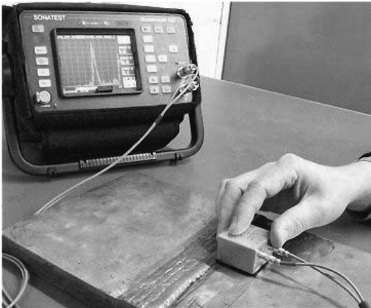
Fig. 5.29 Ultrasonic inspection of a weldment
