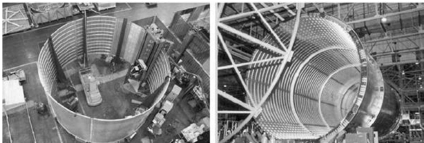
Fig. 6.21 Friction stir weld process development tool at the Marshall Space Flight Center shown with an 8.2 m (27 ft) diameter barrel segment of the 2195 Al-Li external tank for the Space Shuttle at the National Aeronautics and Space Administration (NASA) Michoud Assembly Facility in New Orleans. Courtesy of NASA's Marshall Space Flight Center. Source: Ref 6.10, p 298
