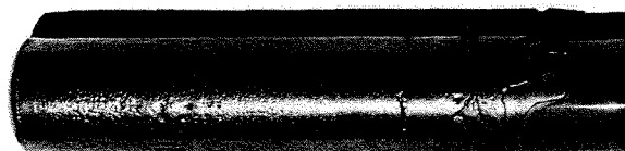
Fig. 6.4. Cylindrical ingot of a Ti-Ni alloy prepared by the plasma melting method. (After Suzuki et al. 6 )
