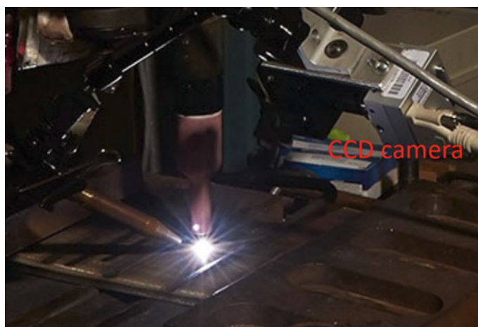
Fig. 3.2 Passive vision weld pool image acquisition system
