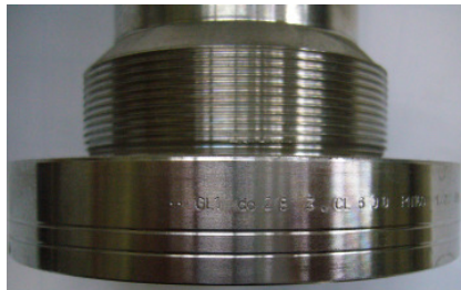
Figure 12.7.4-1: Markings of nozzle
