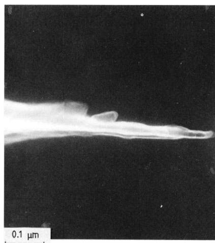
Figure 6.5 SEM image of the edge of a self-sustained oxide layer obtained by thinning a laser-oxidised copper sample. The sample was irradiated for \approx 1980 s at T = 220^\circ\text{C} .
