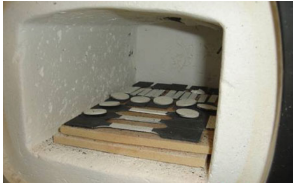
Fig. 7.1 Arrangement of samples in a muffle furnace
