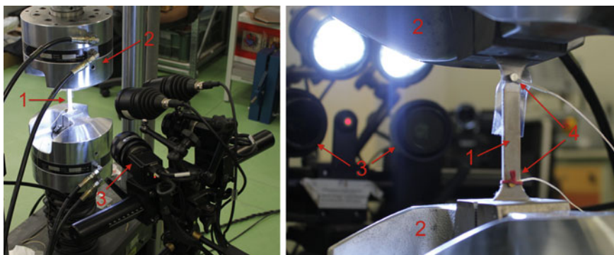
Fig. 6.14 Experimental stand with the ARAMIS system and acoustic emissions for measurement of the TBCs systems deformations
