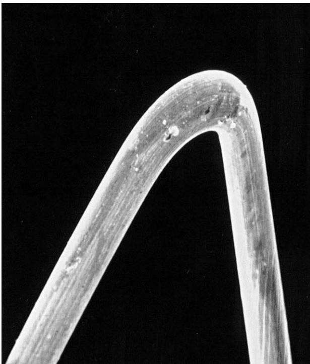
Figure 5.3. The tip of a tungsten hairpin filament. (Reproduced by permission of Williams and Carter 1996.)
