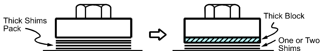
Figure 10. Replacing Thick Shims Pack By Thick Machined Block
