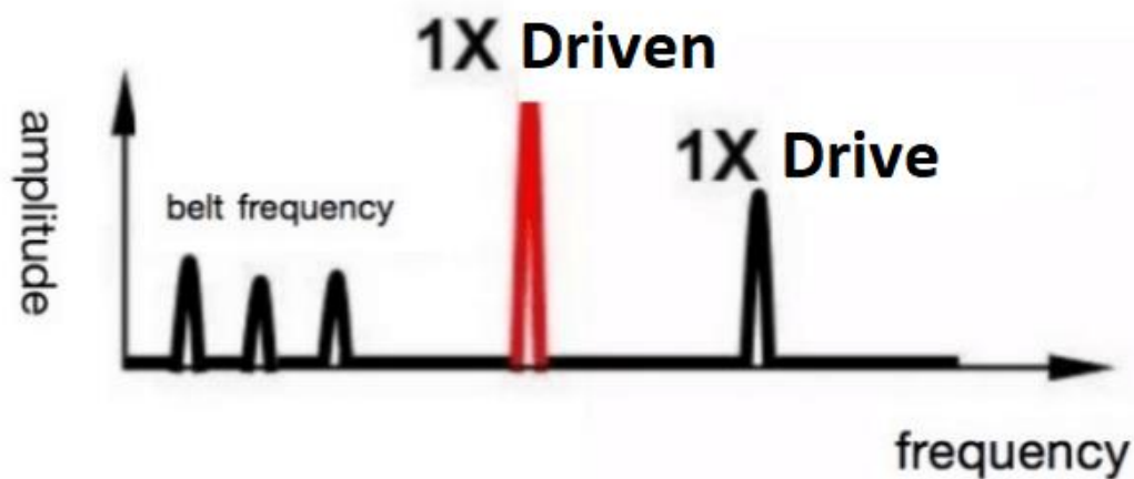
Figure 9.14. Belt frequency with sub-harmonic belt frequencies.
