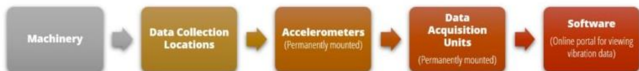
Figure 6.1 .Schematic diagram of automated collection sequence.
