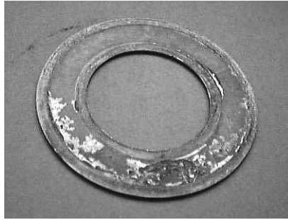
FIGURE 16.3 Steel valve ring subject to corrosion due to water condensation.
