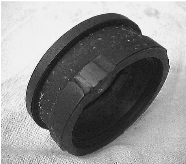
FIGURE 13.24 Carbon ring displaying heavy wear of the torque transmission device.
