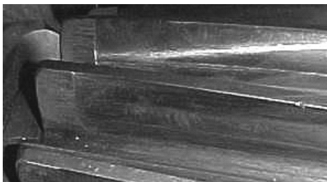
FIGURE 15.5 Gear displaying mild wear.
