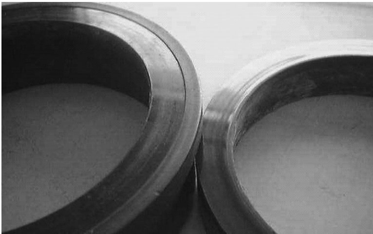
FIGURE 13.12 Faces of a mechanical seal that operated in a propane pump. Note the smooth surfaces, despite an approximately 3 mm material loss on the soft surface.
