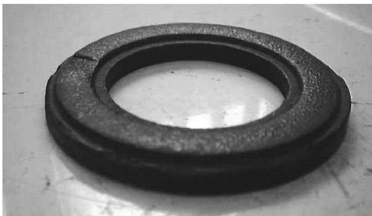
FIGURE 16.1 Reciprocating compressor valve ring subject to heavy wear due to the deposition of abrasive coke particles at the valve seats.
