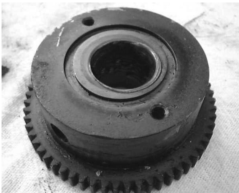
FIGURE 20.4 Overspeed system disc displaying wear on the inside diameter.
