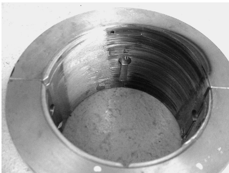
FIGURE 20.18 Pinion bearing displaying heavy rubbing.
