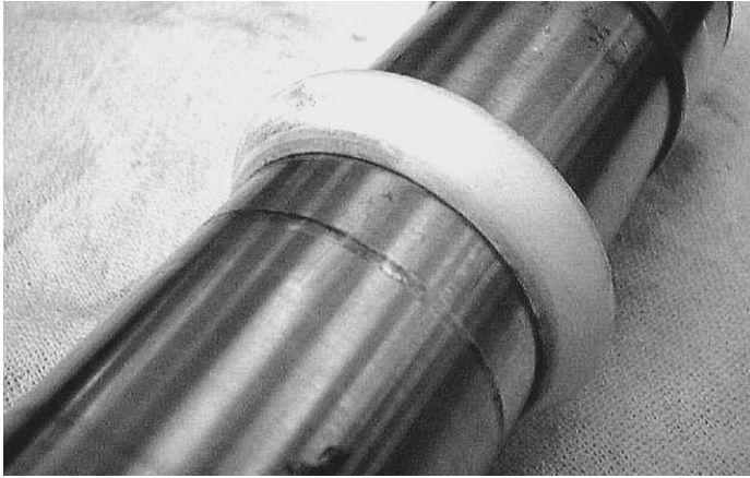
FIGURE 13.27 Seal sleeve with signs of fretting caused by the Teflon wedge.
