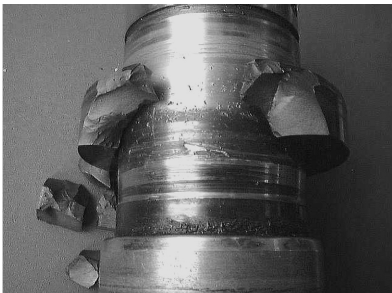
FIGURE 13.18 Tungsten carbide ring damaged by contact with the shaft.
