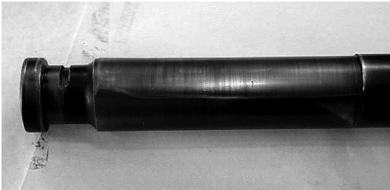
FIGURE 6.5 Metallic surface subject to mild wear.
