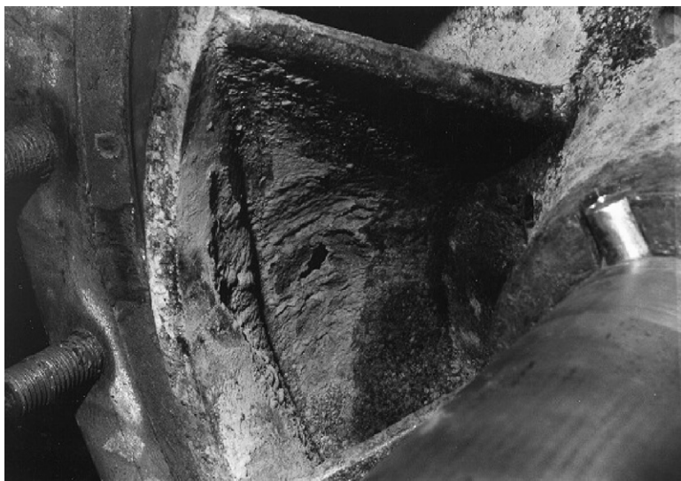
FIGURE 6.24 Cavitation damage in a centrifugal pump impeller.
