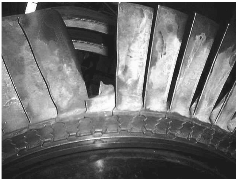
FIGURE 19.14 Hot gas expander rotor that suffered a blade failure due to the formation of nickel sulfide.
