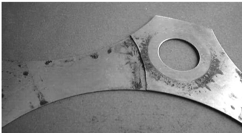
FIGURE 18.3 Centrifugal coupling blade that failed due to misalignment.
