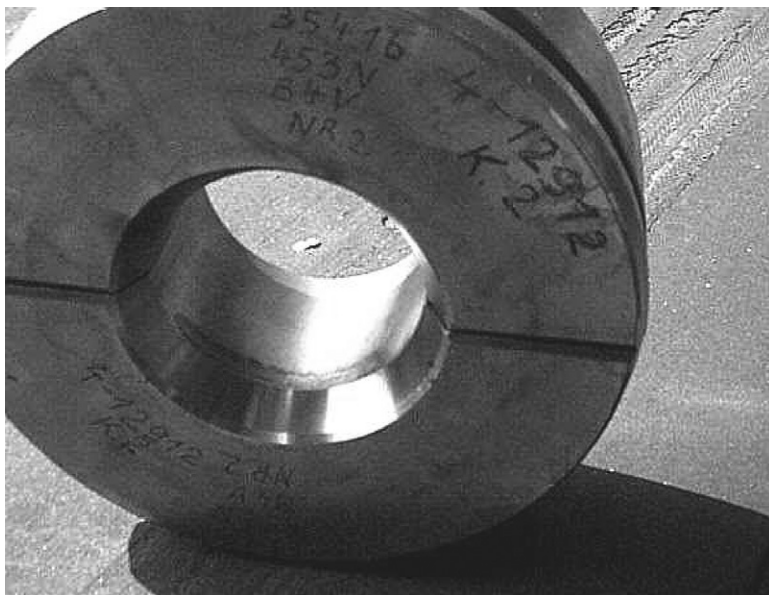
FIGURE 6.13 Compressor split ring with indications of fretting wear.
