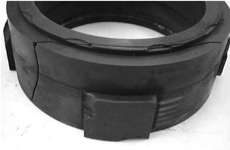
FIGURE 13.19 Carbon ring damaged by drive mechanism impact from oscillating lubrication conditions.
