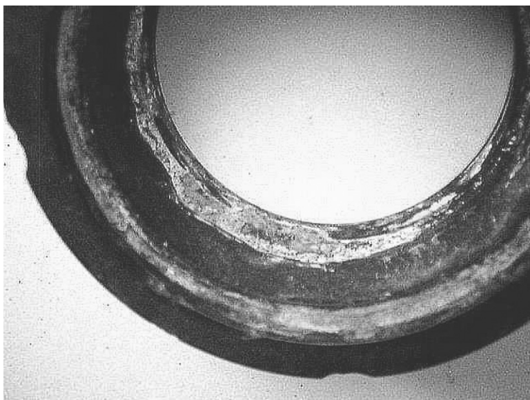
FIGURE 8.7 Iron fluoride incrustation on a mechanical seal carbon ring.
