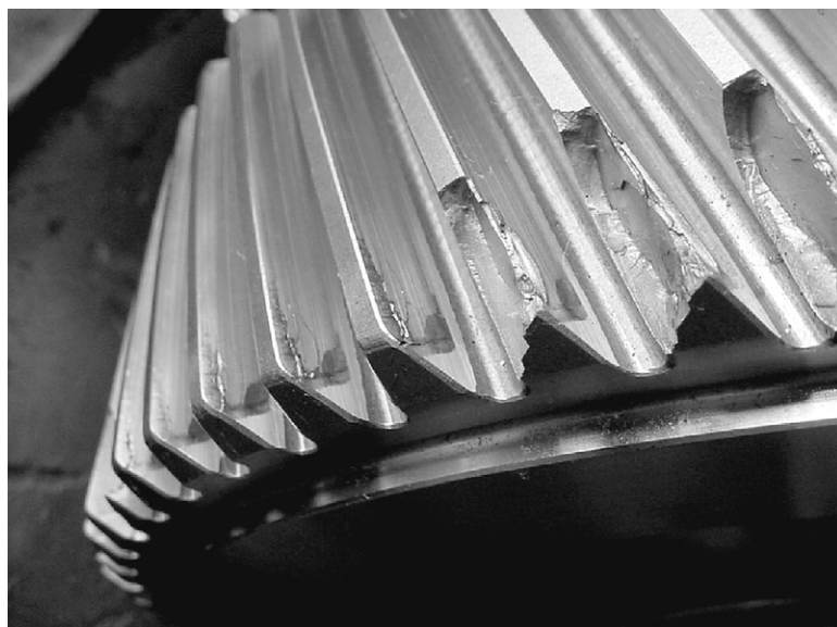
FIGURE 20.16 Broken gear teeth on the step-up gear.
