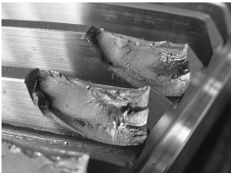
FIGURE 20.17 Closer view of the fracture on the edges of the gear teeth.
