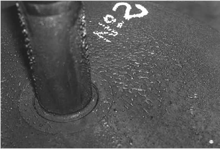
FIGURE 1.2 Reciprocating compressor piston with hard deposits created by the polymerization of the gas.
