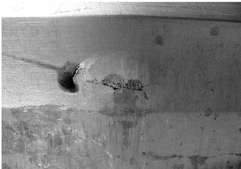
FIGURE 11.13 A blister on the surface of a bearing.
