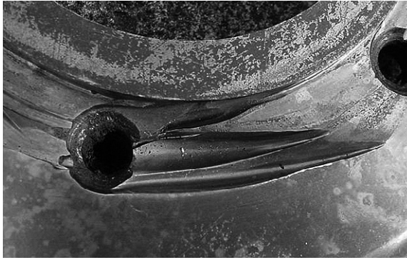
FIGURE 6.19 Severe erosive wear on a pump throttle bushing caused by iron fluoride particles suspended in the pumped fluid.
