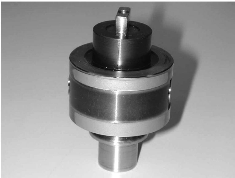
FIGURE 9.1 Primary element of a steam turbine governor with signs of electric discharge damage.
