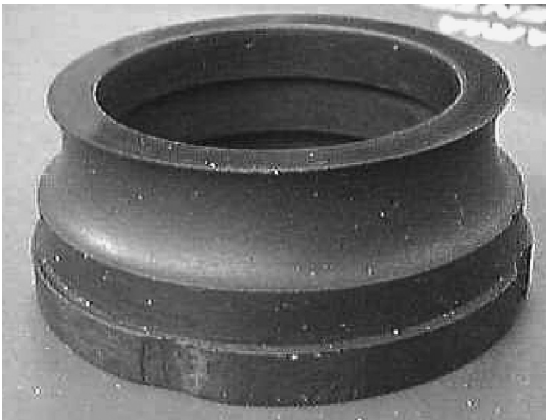
FIGURE 13.14 Carbon ring with erosion due to high-velocity fluid impact.
