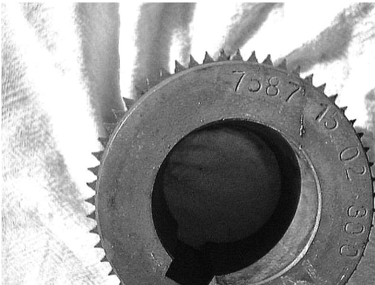
FIGURE 1.5 Gear coupling with signs of severe wear due to the lack of lubrication.
