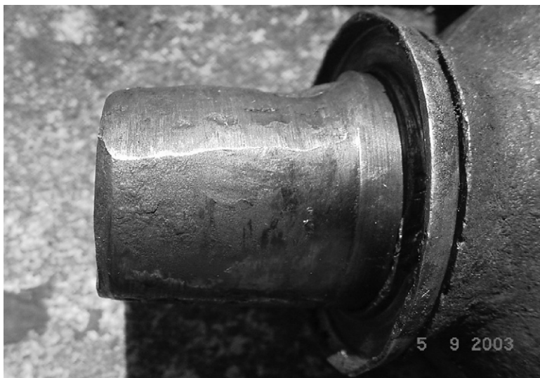
FIGURE 6.9 Crosshead pin with signs of heavy wear, caused by a loss of lubrication.
