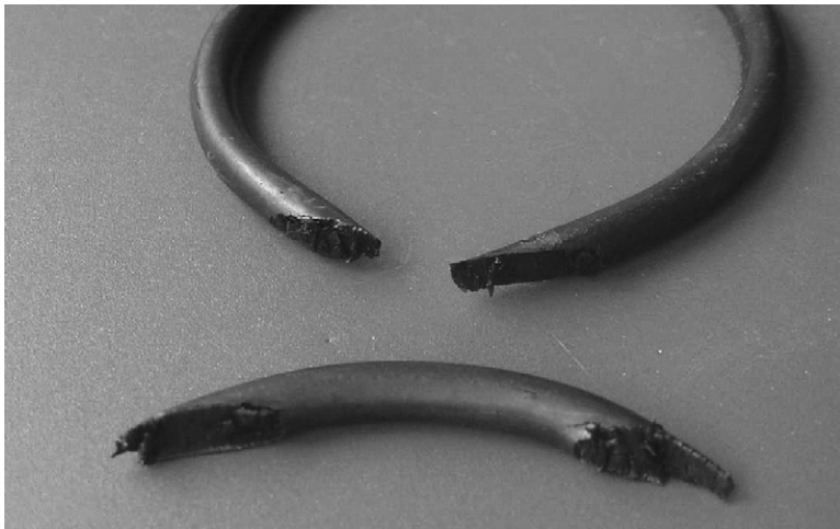
FIGURE 13.23 O-ring cut by the sharp edge on a shaft.
