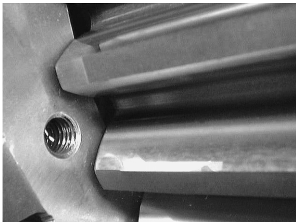
FIGURE 15.3 Gear displaying a polished surface, the result of a correct run-in.
