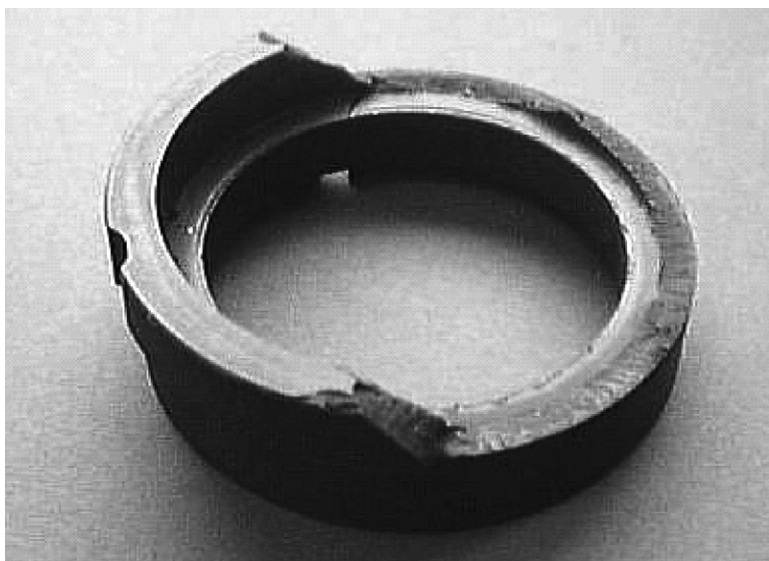
FIGURE 13.17 Carbon ring broken by impact with the inside of the sealing box, caused by pump cavitation.
