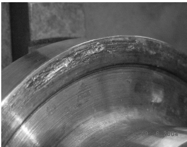
FIGURE 6.4 Metallic surface subject to severe wear and material removal.
