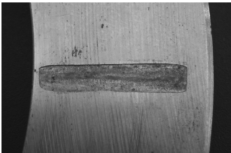
FIGURE 6.12 A centrifugal compressor thrust-bearing support plate with indications of fretting wear.
