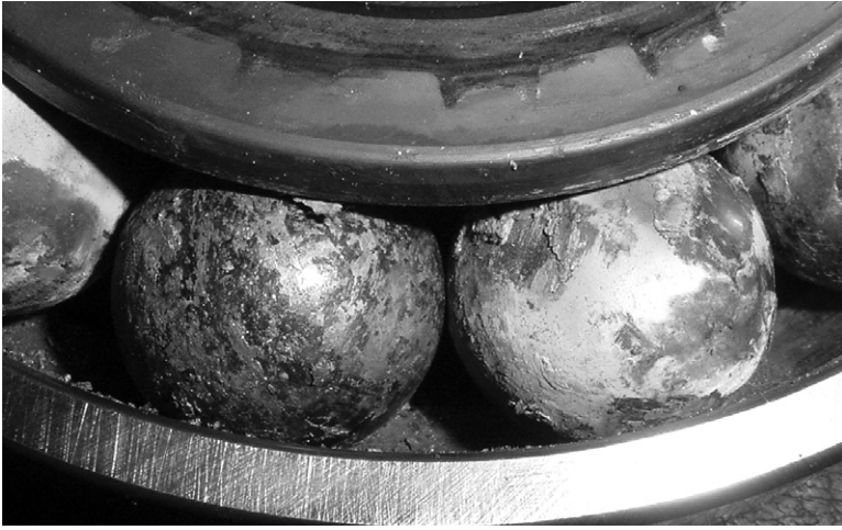
FIGURE 12.23 Thrust bearing of a centrifugal pump that suffered a catastrophic failure due to lack of lubrication.
