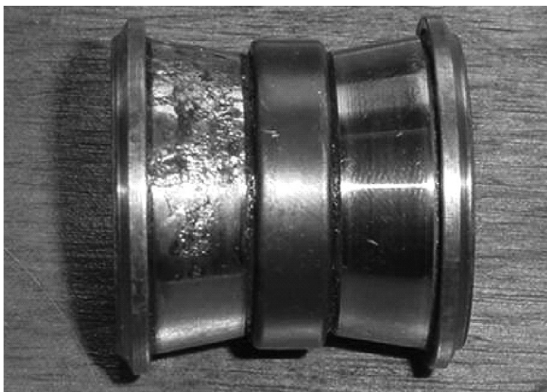
FIGURE 12.14 Double row bearing with heavy damage due to misalignment.
