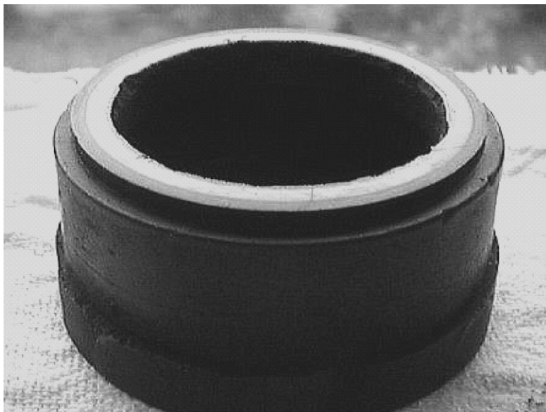
FIGURE 13.20 A carbon ring subject to thermal distortion due to poor heat removal from the interface. Note that there has been contact on the inside diameter only, meaning that the faces have been made convergent by the deformation.
