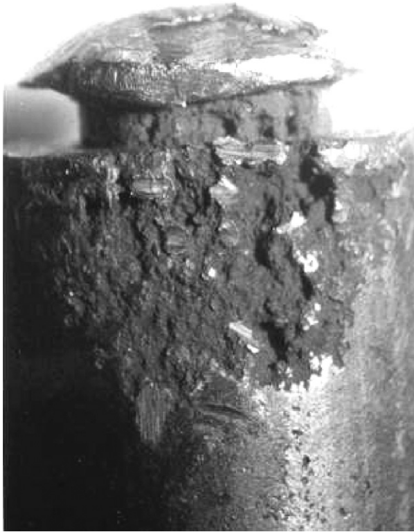
FIGURE 19.5 Signs of erosion found at the shroud rivet on the failed blade.
