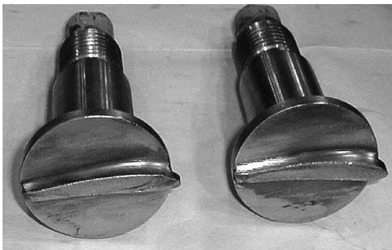
FIGURE 19.7 Fracture surface of the IGV blades, displaying discrete evidence of the fatigue failure.
