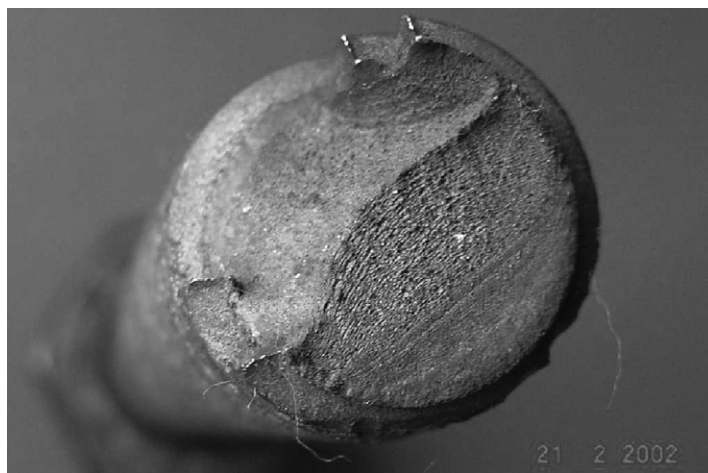
FIGURE 14.3 A fatigue failure of a valve bolt. Note that a certain portion of the fracture surface is oxidized.
