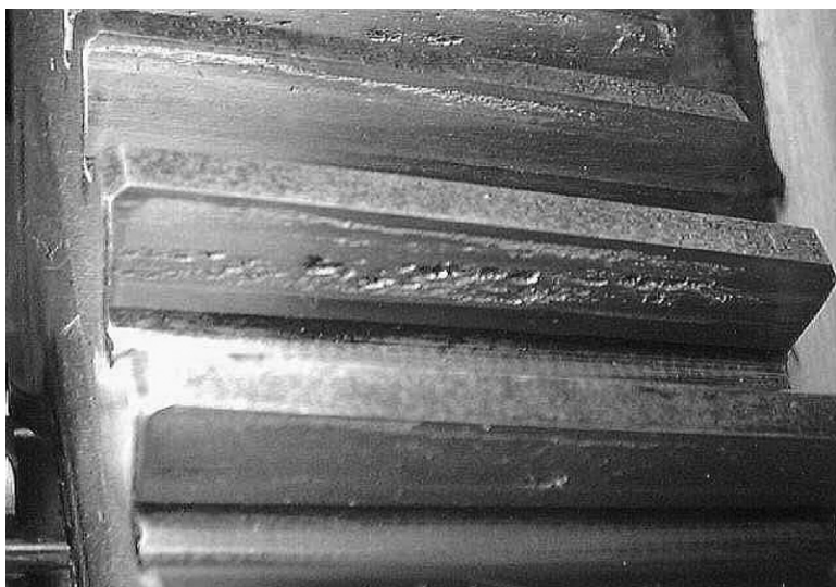
FIGURE 15.8 Overloaded gear, with surface fatigue indications at the dedendum.
