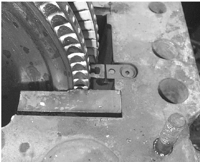
FIGURE 19.11 Steam turbine damaged by water ingestion.
