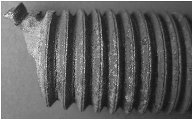
FIGURE 14.5 Bolt of the valve shown in Figure 14.4 that failed due to the overload from the fracture of the first bolt.
