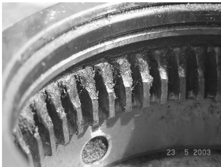
FIGURE 18.9 Gear coupling with sheared teeth due to improper assembly.
