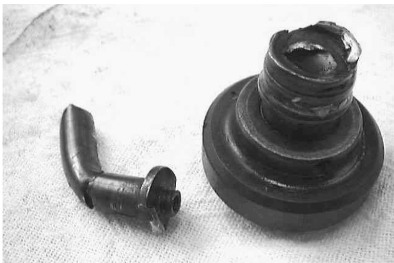
FIGURE 20.3 Overspeed mass and governor coupling damaged after the accident.
