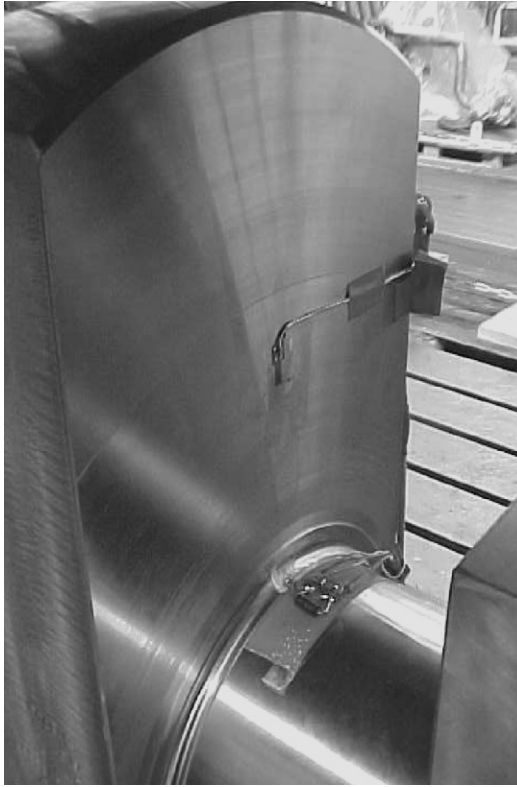
FIGURE 20.14 Measurements of the stress concentration with strain gauges.
