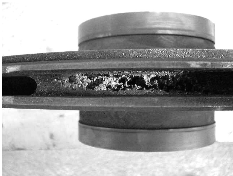
FIGURE 1.6 Centrifugal pump impeller showing signs of wear due to operation with a low flow.
