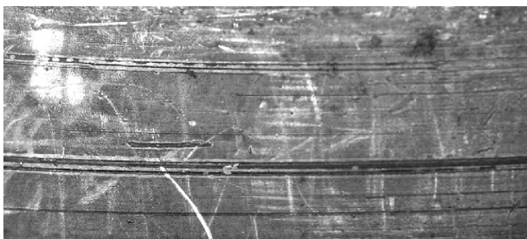
FIGURE 11.5 Radial bearing of a reciprocating compressor grooved by hard particles.
