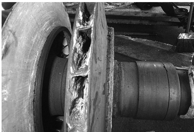
FIGURE 8.6 Ammonium chloride incrustation in a compressor rotor.
