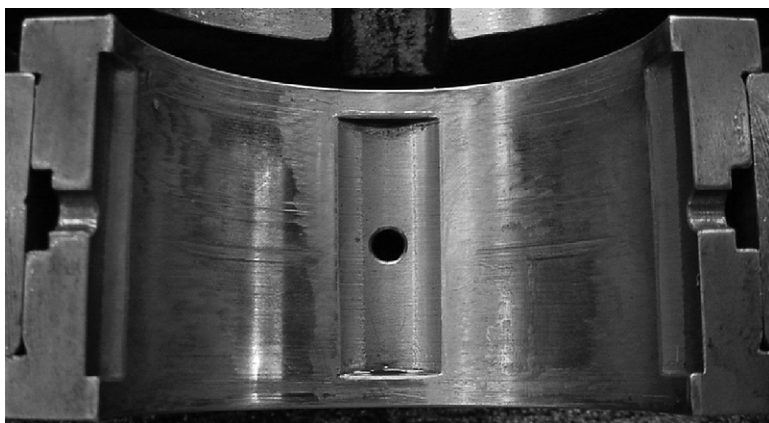
FIGURE 6.8 Hydrodynamic bearing showing some signs of mild wear.
