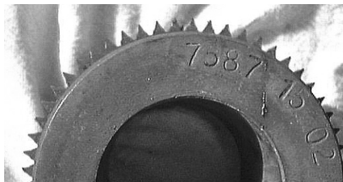
FIGURE 18.8 Gear coupling displaying heavy wear due to lack of lubrication.
