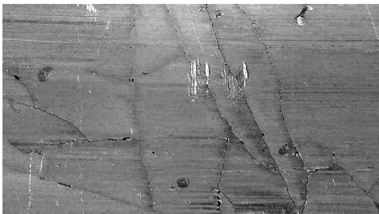
FIGURE 11.8 Bearing surface with thermal fatigue cracks.
