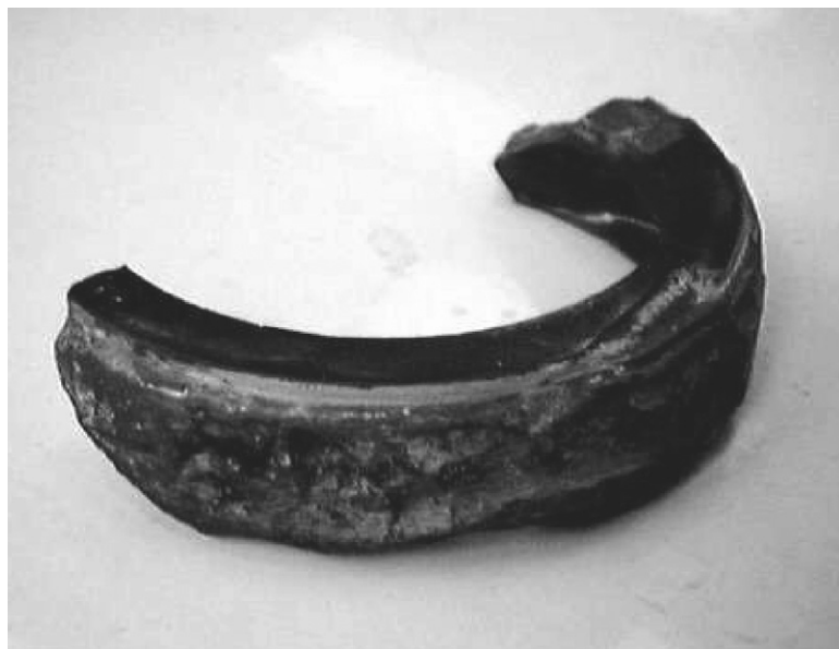
FIGURE 13.8 Carbon ring showing severe corrosion due to misapplication.
