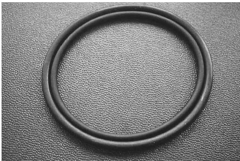
FIGURE 13.9 A swollen O-ring, shown on the outside. The ring on the inside is a new one, introduced into the picture to make comparison possible.
