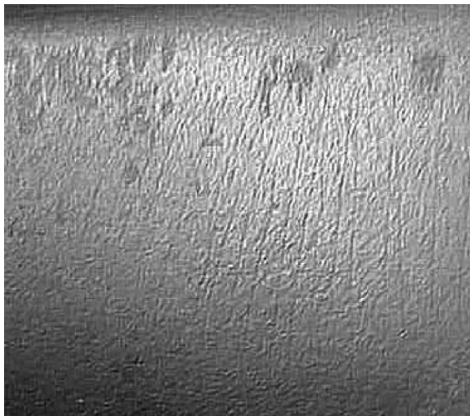
FIGURE 19.15 Thermal fatigue on a hot gas expander blade surface caused by improper control of the cooling steam.
