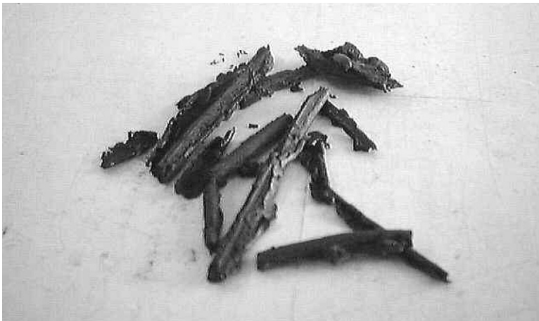
FIGURE 13.11 Elastomer O-ring that suffered chemical attack due to exposure to hydrocarbons.
