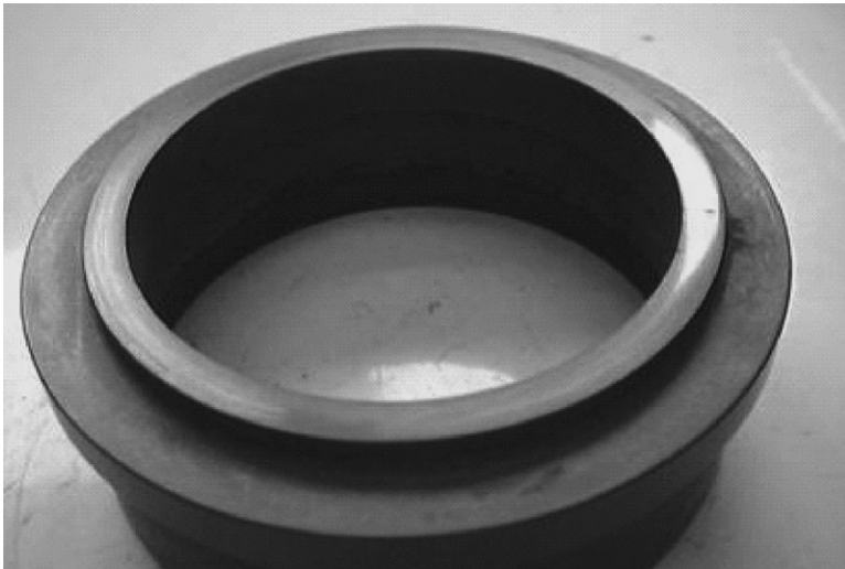
FIGURE 13.21 Carbon ring mechanically distorted by a drive mechanism problem. A crack developed at the distorted point.
