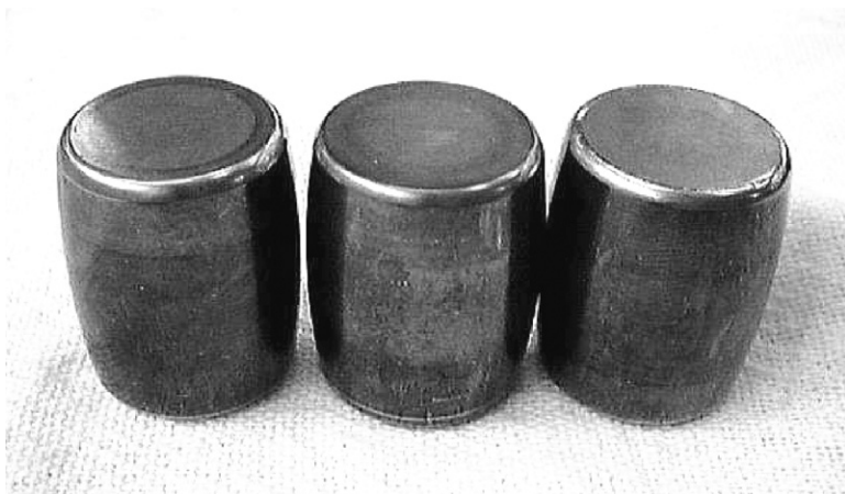
FIGURE 12.22 Rollers subject to poor lubrication, with the consequent polishing of the surface and oxidation.
