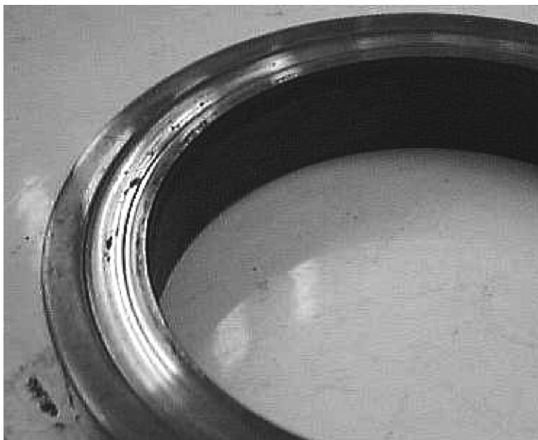
FIGURE 13.13 Seal ring with grooves produced by hard particles.
