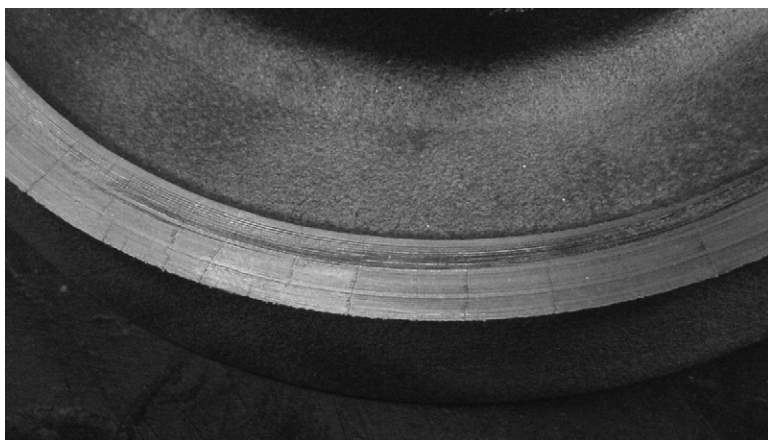
FIGURE 6.3 Surface subject to sliding wear. Concentrically placed scratches caused by the sliding can be seen together with radial cracks caused by the heat chock.
