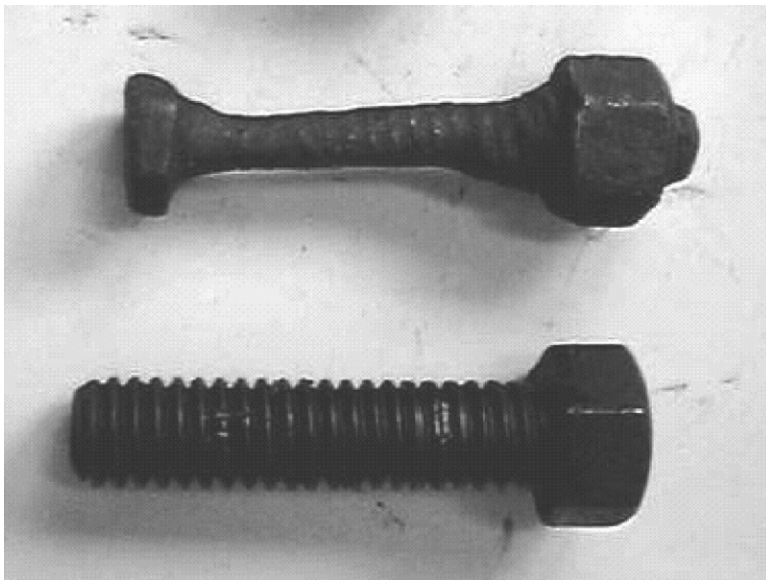
FIGURE 14.6 A bolt corroded by contact with hot hydrocarbons.
