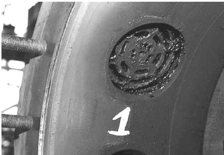
FIGURE 16.2 Compressor valve covered with coke.
