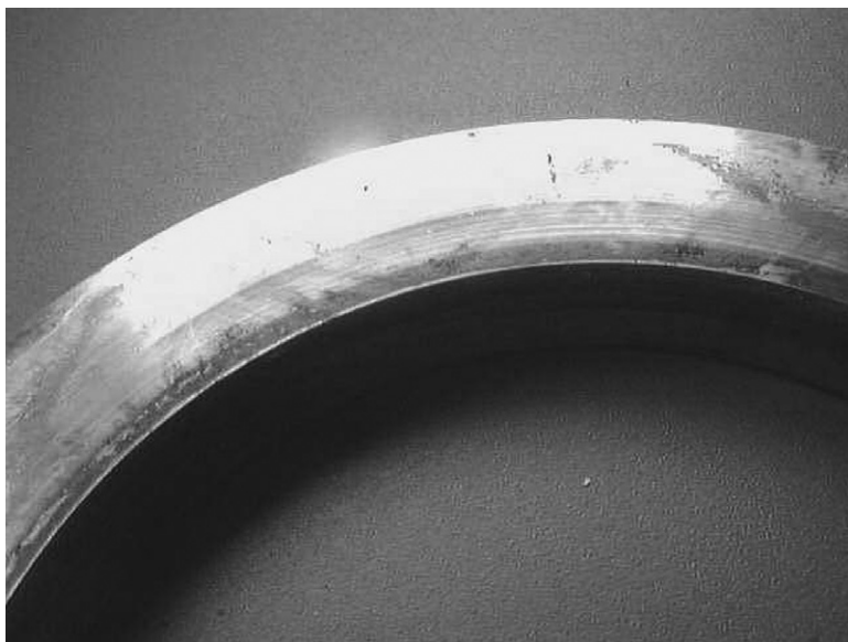
FIGURE 12.21 Axial bearing race with signs of oil additive plating due to high temperature.
