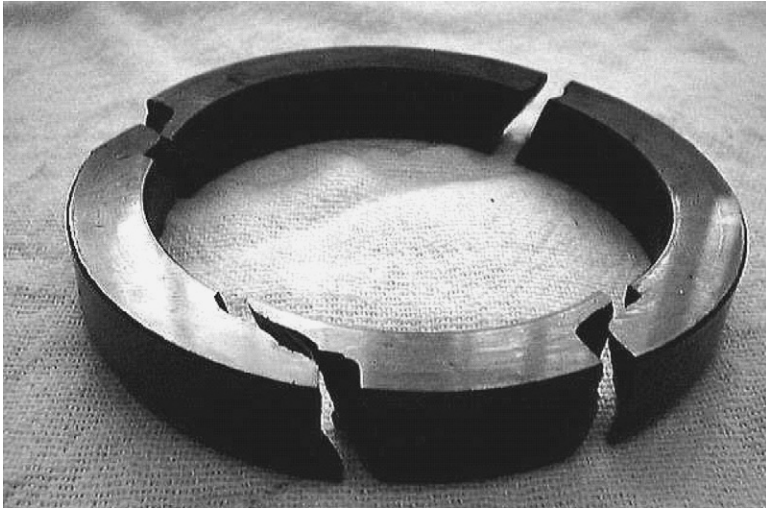
FIGURE 13.16 Silicon carbide seal ring broken due to thermal chock.
