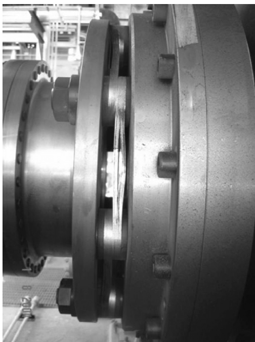
FIGURE 18.5 Blades plastically deformed by the oscillating torque.
