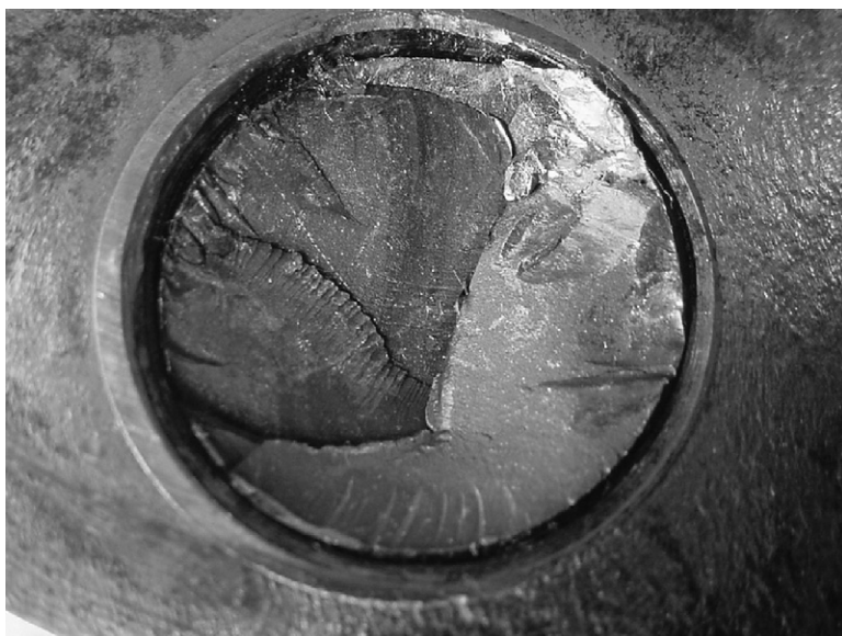
FIGURE 14.9 Fracture surface, displaying ratchet marks.
