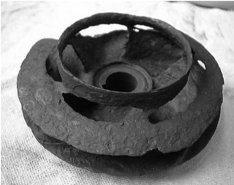
FIGURE 7.2 Pump impeller that suffered uniform corrosion.
