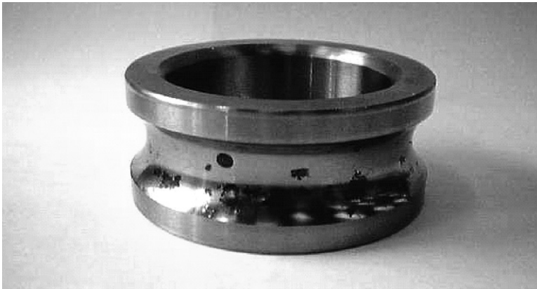
FIGURE 12.27 Corrosion due to contamination of the oil with water, caused by ineffective sealing of the machine.
