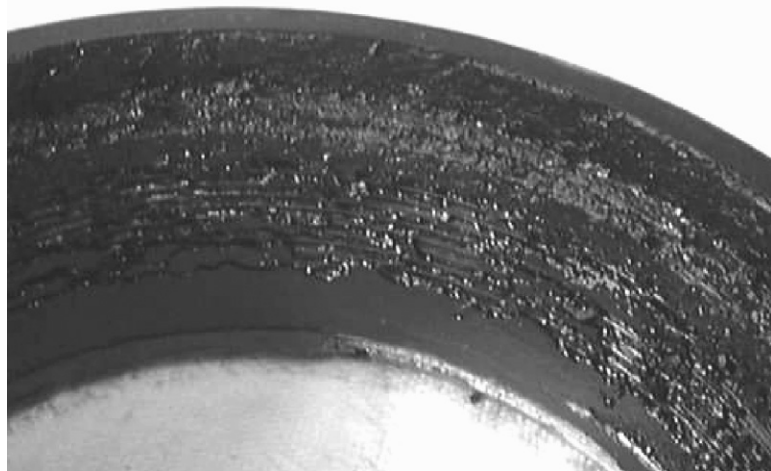
FIGURE 13.22 Metal bellows with coke accumulation on the inside.
