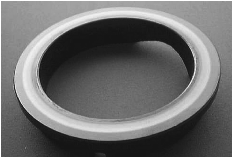
FIGURE 13.7 Silicon carbide seal ring showing a normal contact pattern after a long time in service.
