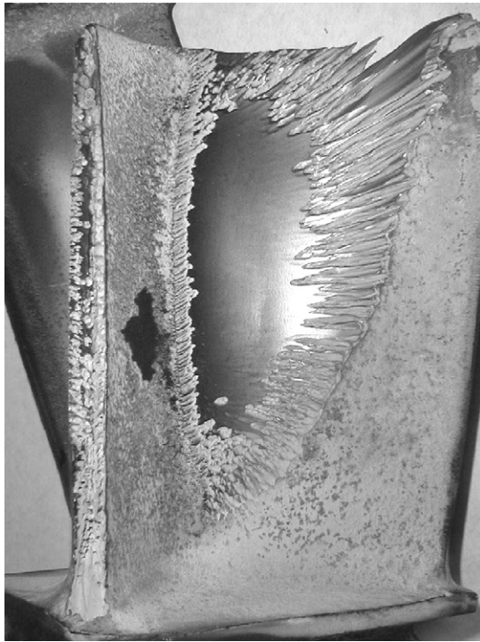
FIGURE 19.9 Hot gas turboexpander blade with signs of wear due to the impact of hard catalyst particles.
