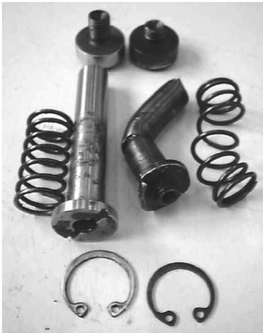
FIGURE 20.6 Comparison between the damaged (right) and a new (left) overspeed mass. Note the difference in bolt size of the new component.
