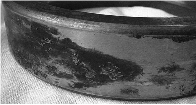
FIGURE 12.19 Bearing outer race with signs of fretting due to a loose fit.
