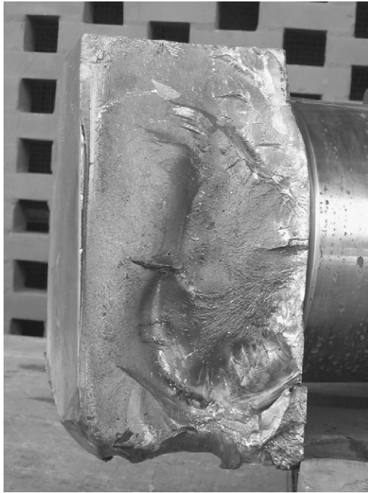
FIGURE 20.12 Crankshaft fracture face. Note the ratchet marks on the right side, indicating a high stress concentration and several fracture initiation spots.
