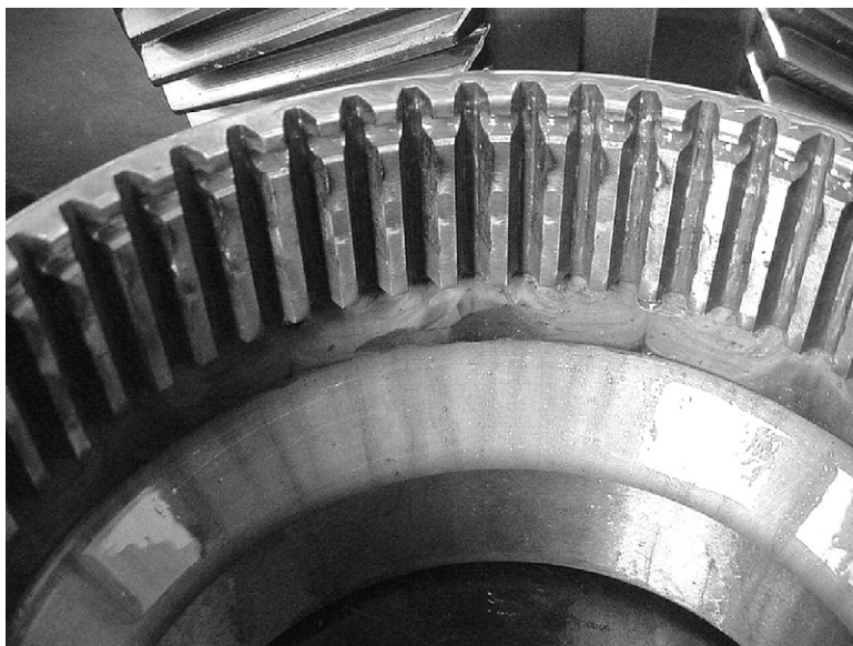
FIGURE 20.19 Gear coupling displaying signs of electrical discharge damage.
