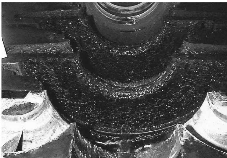
FIGURE 8.3 Coke incrustation in a centrifugal compressor.
