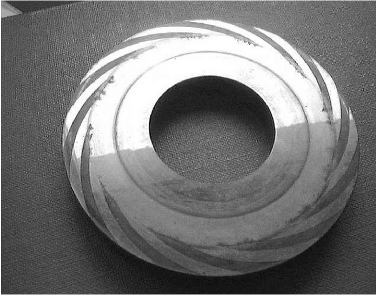
FIGURE 13.2 Mechanical seal face with grooves to improve the hydrodynamic effect.
