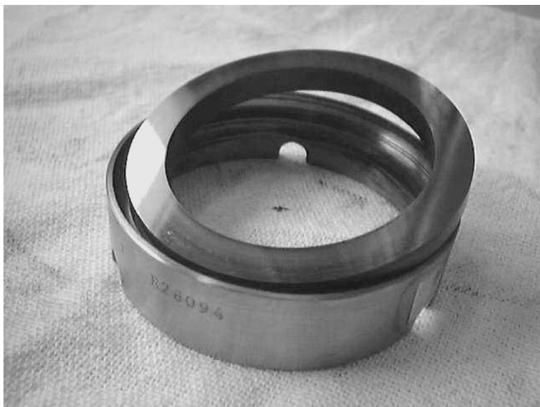
FIGURE 13.26 Seal ring with inserted tungsten carbide face.
