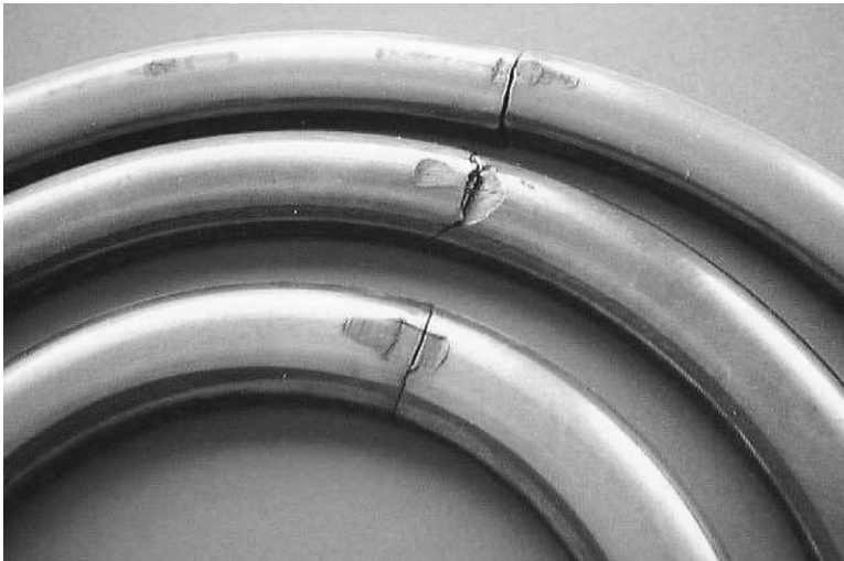
FIGURE 16.4 Valve rings broken due to irregular action of the valve unloaders. Note the indentation caused by the unloader fingers.
