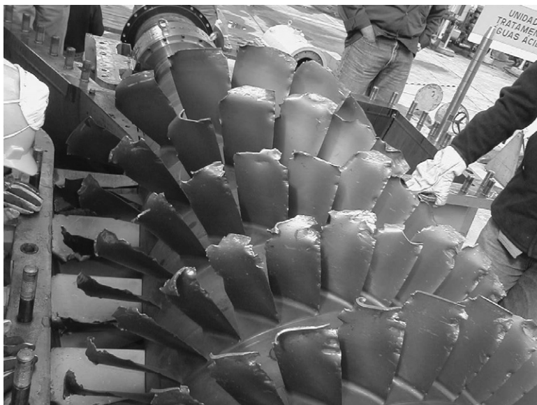
FIGURE 19.6 Axial blower rotor damaged from the fracture of the IGV blades.
