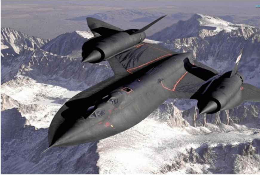
Fig. 3.4 SR-71 Blackbird with airframe comprises 93% titanium [26]
