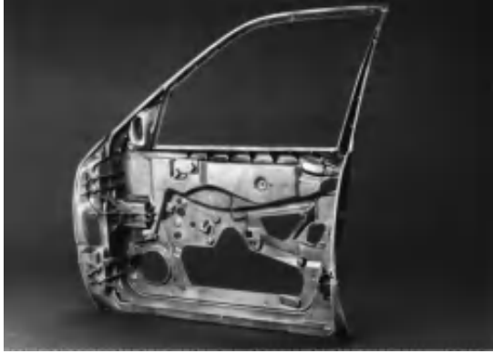
Figure 8: Concept for inner-door parts: version 3, Mg die-casting
