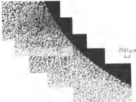
Figure 16: The crack-free surface of a thixo-cast component (AZ91D) [22]
