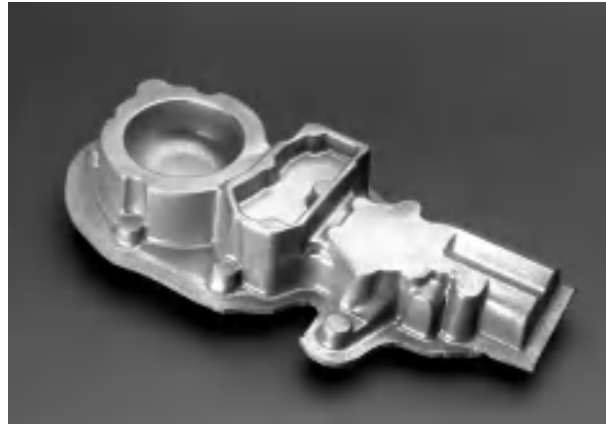
Figure 13: VANOS housing of WE43-T5 (200 × 80 mm)
