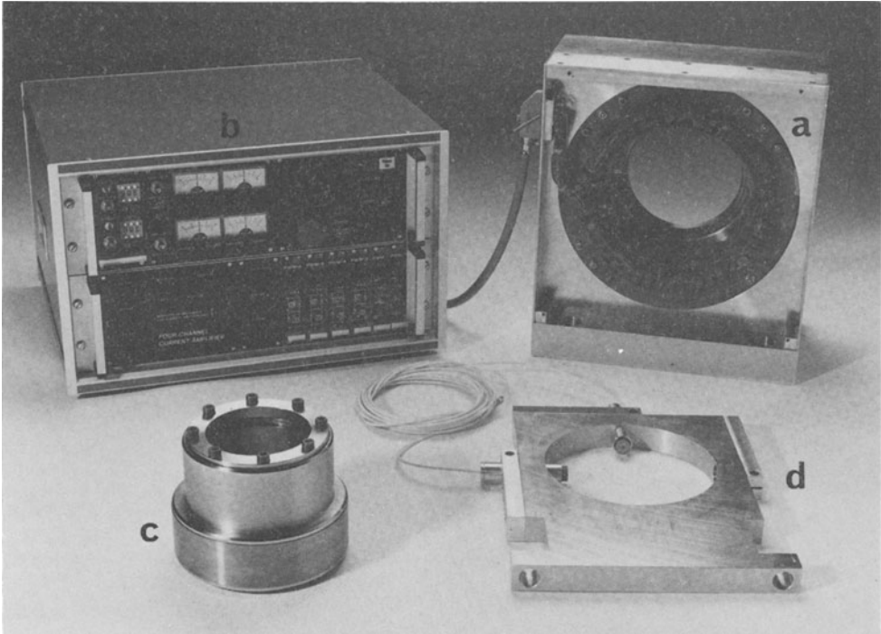
Fig. 1: Magnetic Actuator ETH-190/50/1 a) Magnet unit b) Power amplifier and signal conditioning c) Rotor sleeve d) Sensor unit.
