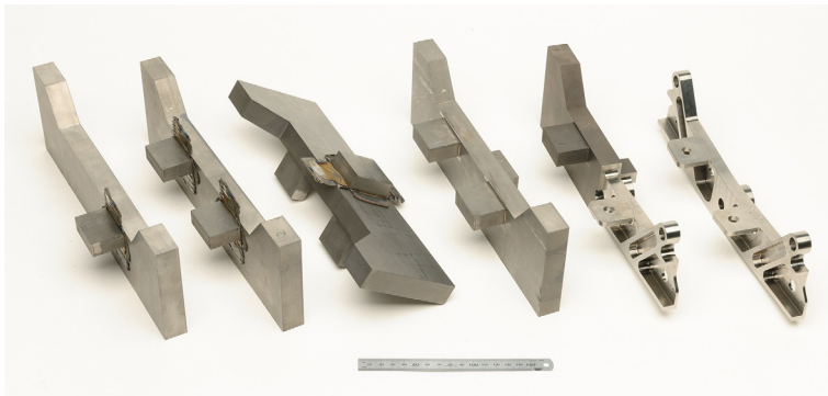
Fig. 1.10 Near net shaped parts produced by linear friction welding.
