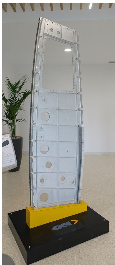
Fig. 1.9 Wing rib with feet attached to rib by linear friction welding.
