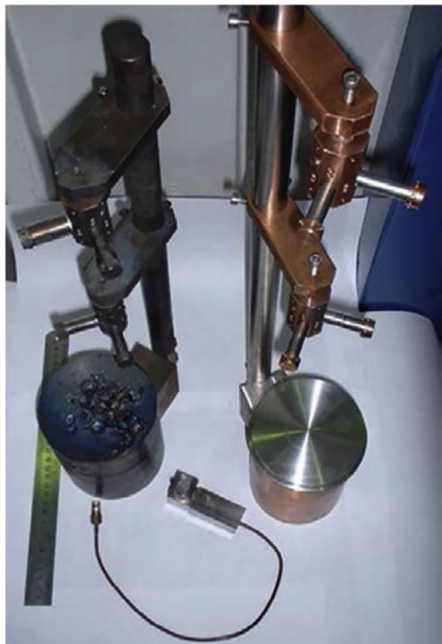
Fig. 6.14 Electron beam quality control device Beam Probe by CVE and TWI.
