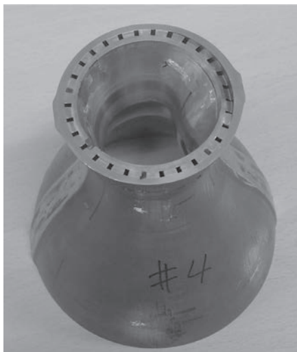
Fig. 10.26 Photographs of combustion chamber pressure welded with copper cooling channels.
