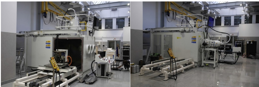
Fig. 6.24 Quick tooling change, possibility to set up electron gun in vertical and horizontal position, EB machine at Instytut Spawalnictwa (Institute of Welding) in Poland.
