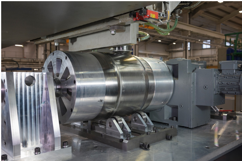
Fig. 1.6 Friction stir welding of Ti-6-4 propellant tank for European Space Agency.
