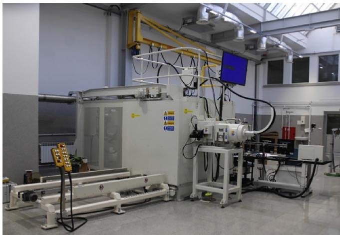
Fig. 6.12 A universal electron beam welding machine model XW150:30/756 for welding and surface modification installed at the Institute of Welding in the year of 2014, (30 kW, 150 kV), produced by Cambridge Vacuum Engineering (CVE).
