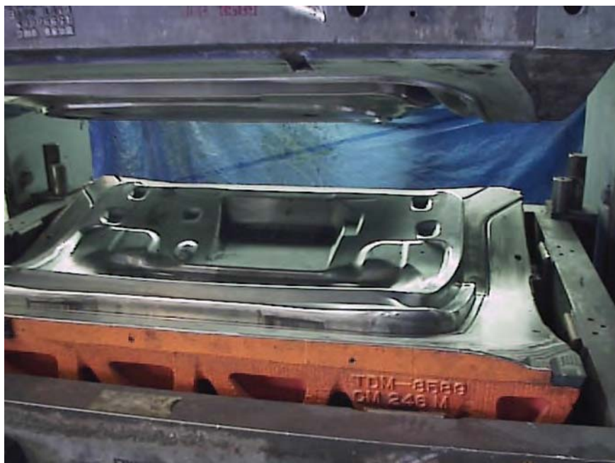
Fig. 15.18 Segmented flexible binder tool for the liftgate inner in mechanical press. Source: Ref 15.8
