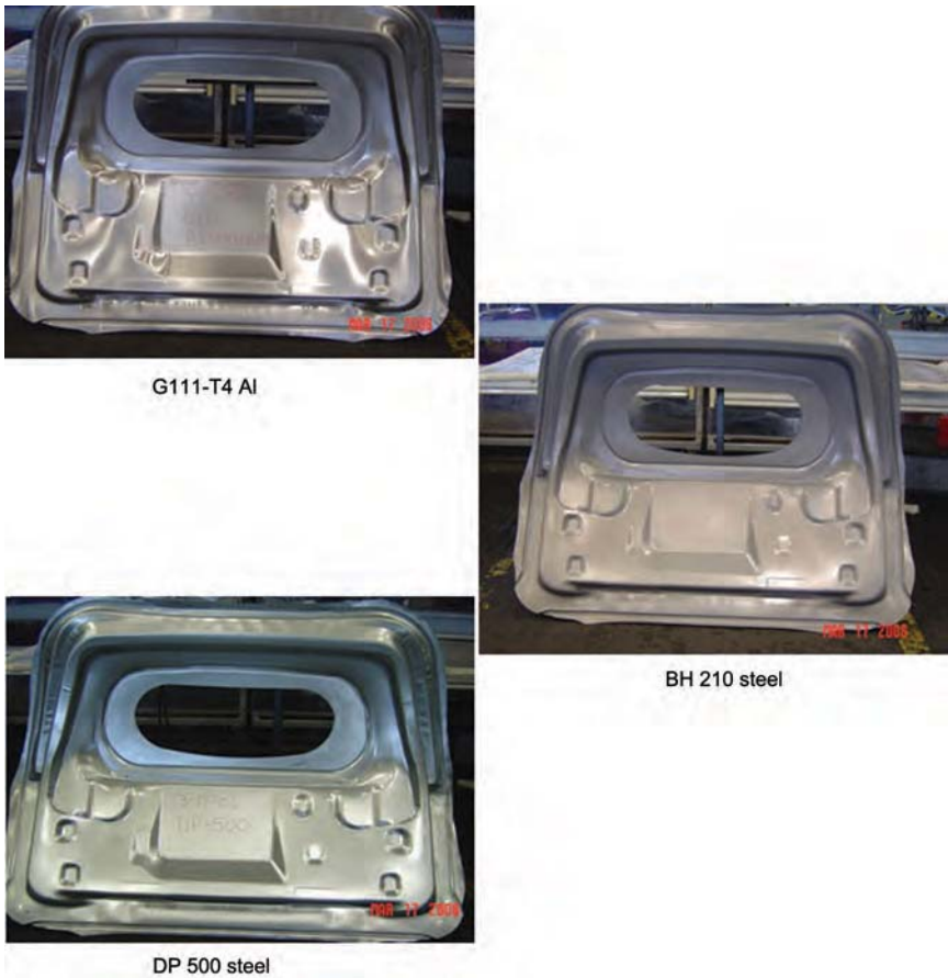
Fig. 15.19 Liftgate inners made from three different metals using the same flexible tooling. Source: Ref 15.8
