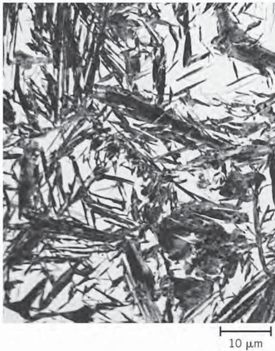
Fig. 2.11 Martensite microstructure (needle-shaped grains) and retained austenite (white matrix). Source: Ref 2.1
