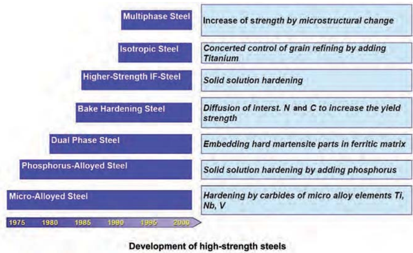
Fig. 1.12 Development of high-strength steels over time. Source: Thyssen, Ref 1.14
