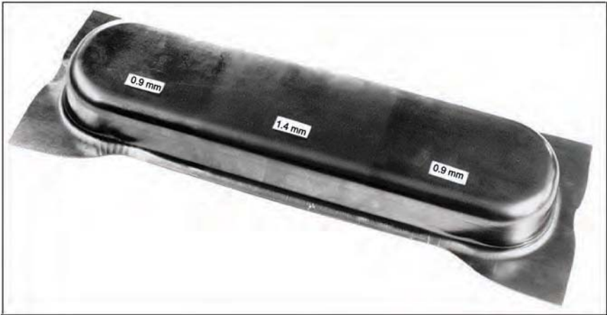
Fig. 15.26 Experimental pan made from flexible rolling blank. Source: Ref 15.10
