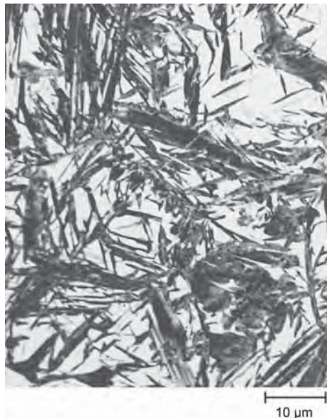
Fig. 8.1 Microstructure of martensite. Source: Ref 8.1
