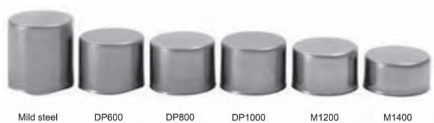
Fig. 4.18 Variation of cup height with strength for different types and grades of steel. Source: Ref 4.10
