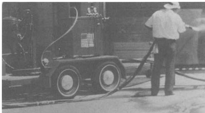
FIG. 29—ADMAC high-pressure water blasting equipment (courtesy of KTA-Tator, Inc.).
