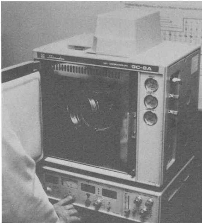
FIG. 3—Gas chromatograph used to generate chromatogram (courtesy of KTA-Tator, Inc.).
