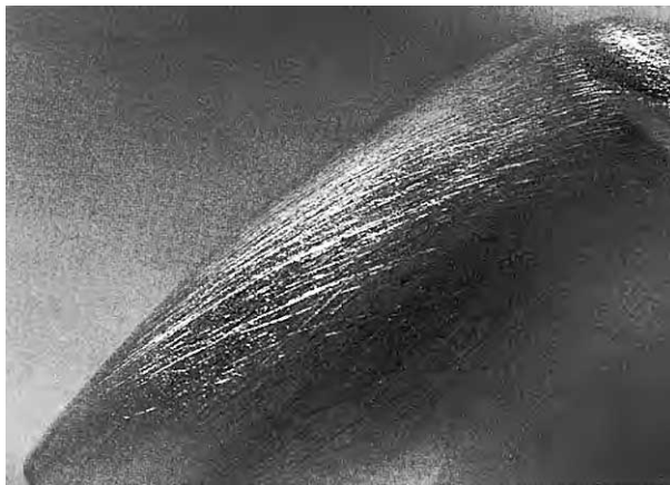
Figure 3.28 Photo showing craze formation on an acrylic part
