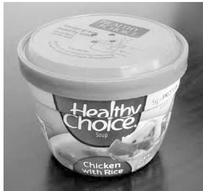
Figure 7.18 The injection molded HDPE microwavable food container has a shrink fit “foamed” thermoplastic label that also acts as a thermal insulator
