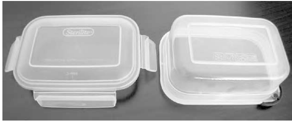
Figure 7.16 Unlike attached or direct print labels, labels (text, symbols, etc.) that have been molded into a thermoplastic item have no negative impact on the recyclability of the item. Molded labeling is the preferred method of labeling from a recycling perspective but the lack of contrast limits its practical value
