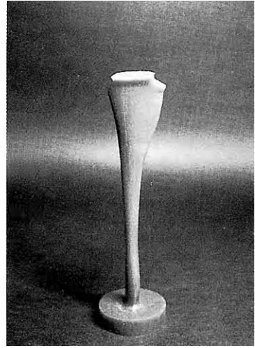
Figure 5.4 (left) Machined plastic parts for a prototype drive assembly, and (right) prosthetic part machined from plastic stock
