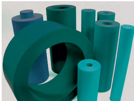
Figure 5.2 Semi-finished thermoplastic rod and sheet stock serve as the raw material for machined plastic prototypes
