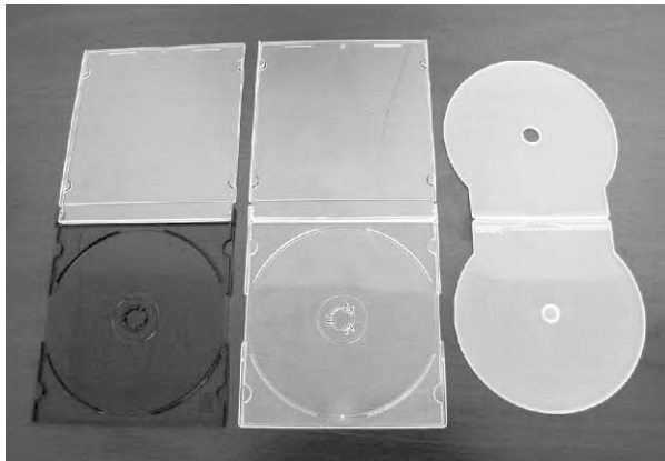
Figure 7.8 The CD “jewel” cases are hinged using molded features. The “one-piece” PP case on the right is molded with an integral hinge, eliminating any need for disassembly. The two-piece polystyrene hinges (left and center) have snap hinge features that are easily disassembled. Disassembly of the PS cases themselves is not a pre-requisite for recycling/regrinding. Although disassembly is not necessary in either case because all of the parts are polystyrene, disassembly would lead to two higher value streams in the case of the natural and black case. In this sense, the all-transparent case could be considered to be more recyclable than the natural and black case
