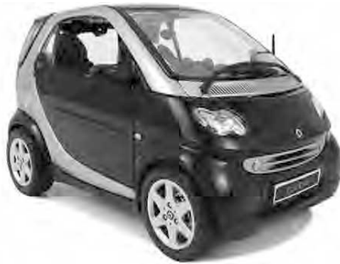
Figure 7.20 Almost all plastic automotive body panel are painted with highly UV resistant class A surface coatings to meet the demands of the application. Some exterior parts, particularly black and gray parts, are pigmented internally. More vibrant-in color body panels have had limited application commercially. Smart Cars have molded-in color body panels that are said to be fully recyclable [24]
