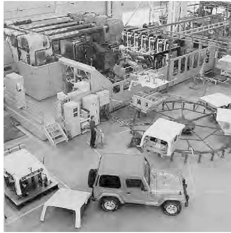
Figure 7.13 The injection molded thermoplastic removable hardtop for the Jeep® Wrangler is a more recyclable alternative to its thermosetting composite predecessor
