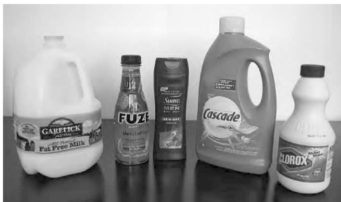
Figure 7.17 Each of the containers shown in the figure are blow molded HDPE containers; however, each container has a different type of attached label. Most labels are printed on thermoplastic films. All of these items are recyclable as post-consumer HDPE, some more easily than others due to their different label types. Labeling methods from left to right are: a stretch film LDPE label, a heat shrink film label, an oriented plastic film label with pressure sensitive, an in-mold label (IML), and a wrapped oriented film label with adhesive at the overlap area only
