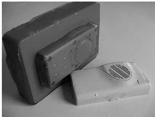
Figure 5.32 Stereolithography epoxy core shell backed with metal powder filled cast
