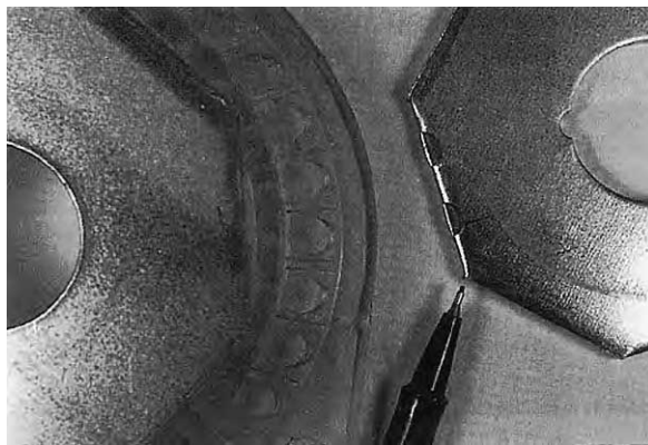
Figure 6.76 Sharp edges on the metal insert result in stress concentrations and crazing due to the mold shrinkage of the polymer. Edges on inserts should be well rounded to provide a more uniform stress distribution
