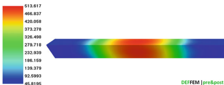
Fig. 9.18 The temperature field after 25 s of heating (type C sample)
