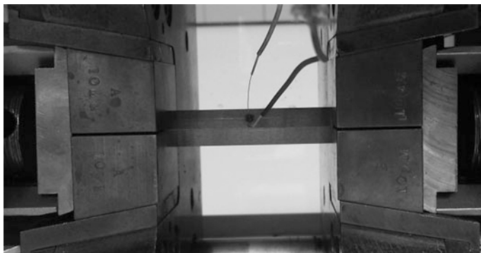
Fig. 9.1 The view of the Gleeble 3800 simulator with a type C hexahedral sample and a control thermocouple installed
