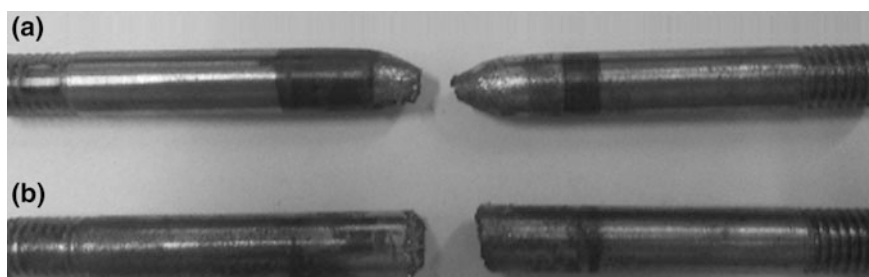
Fig. 7.8 The appearance of the C45 steel samples after reaching the temperature of a 1350 °C and b 1400 °C
