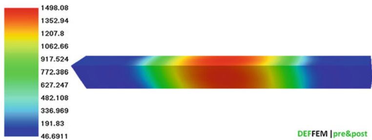
Fig. 9.21 The temperature distribution just before deformation at the nominal temperature of 1450 °C (type C sample)
