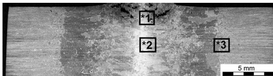
Fig. 9.34 Identification of the microstructural test areas (1-peak, 2-centre, 3-transition zone)
