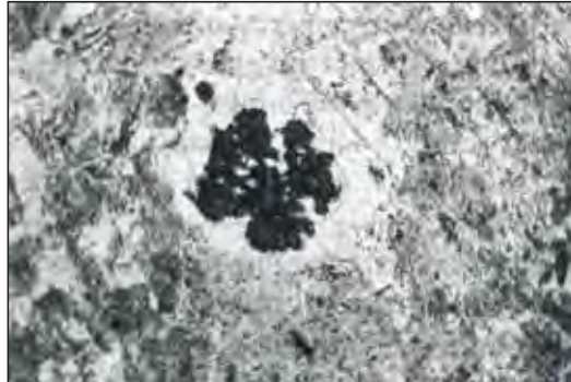
Figure 7.16 Temper carbon is present in the form of approximately spherical aggregates in a malleable cast iron.
