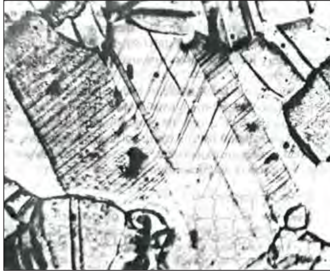
Figure 5.8 Slip lines on a prepolished surface of copper after plastic deformation.
