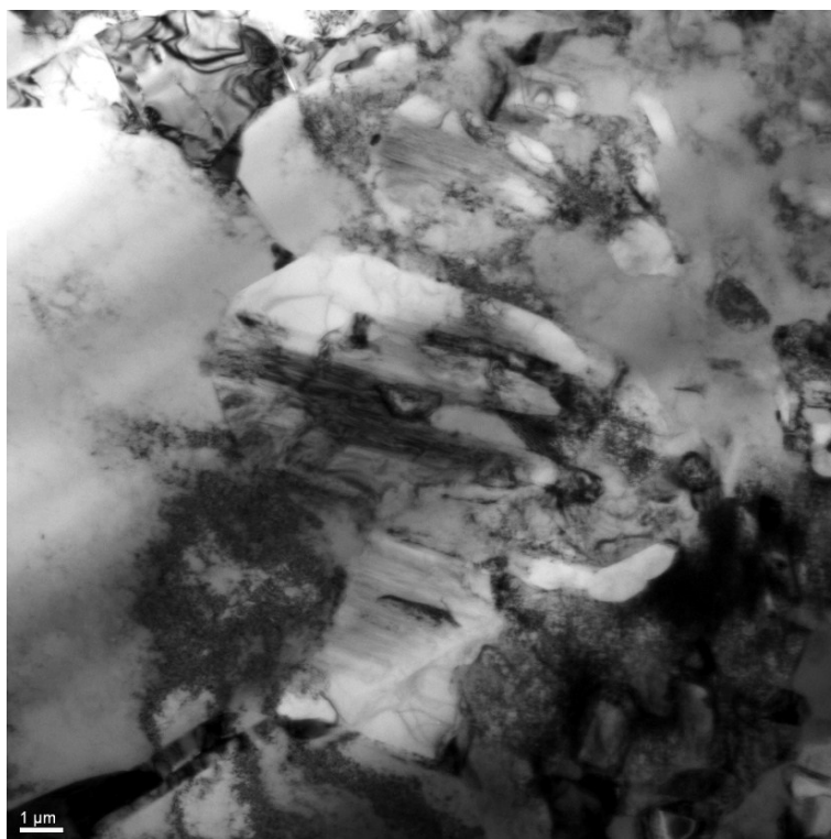
Figure 3. Electron-microscopic image and the structure of silumin of the grade AK12 before electroexplosive doping (initial state).
