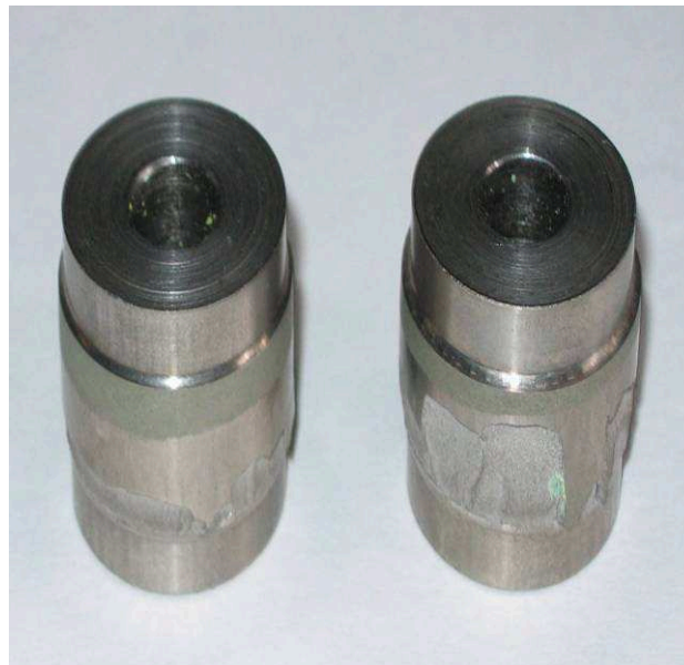
Fig. 9. Appearance of samples pressed through a matrix after shear test
