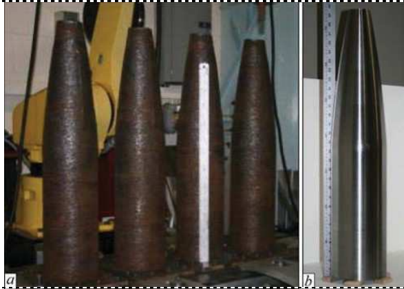
Figure 3. Shell casing of 160 mm diameter and 800 mm length with 8 to 18 mm wall thickness of 32 kg weight from high-strength steel made by WAAM technology (pulsed MIG welding) with productivity of 4 kg/h before (a) and after (b) machining [9].
