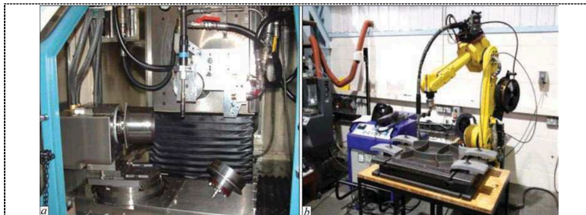
Figure 1. Complexes for realization of additive welding technologies [9]: a – five-axes system with CNC milling and WAAM technology; b – WAAM process without machining realized using an anthropomorphic laser.
