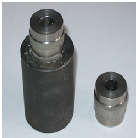
Fig. 4. The sample and a matrix for shearing testing technique
