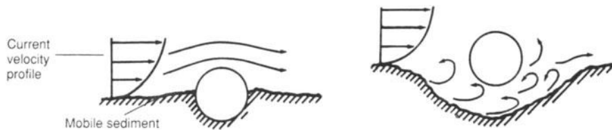
Fig. 1.7. Schematic representation of the development of a subsea pipeline freespan.
