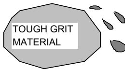
Figure 2.10 Role of grit shape and toughness of grit material in abrasive wear.
