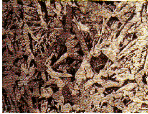
Figure 8.17 Micrograph of Wittmanstraten microstructure.
