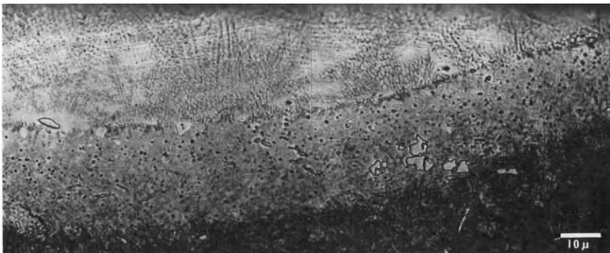
Fig. 5.26. Laserglaze TM processed M-50 steel showing undissolved carbides in HAZ. These carbides are dissolved in the melt zone.
