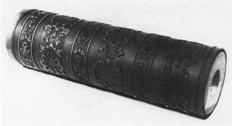
Fig. 2.13. Flexographic print roll machined by laser (Courtesy of Laser Techniques Ltd).
