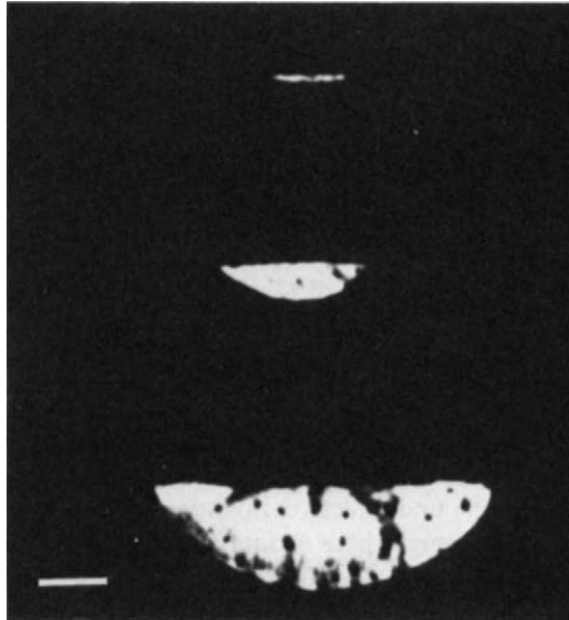
Fig. 6.2. Transverse sections of laser melted trails in Udimet 700 for an incident beam intensity of 535 W: (top) v = 111 \text{ cm s}^{-1} ; (middle) v = 23 \text{ cm s}^{-1} ; and (bottom) v = 3 \text{ cm s}^{-1} . Marker represents 0.1 mm.
