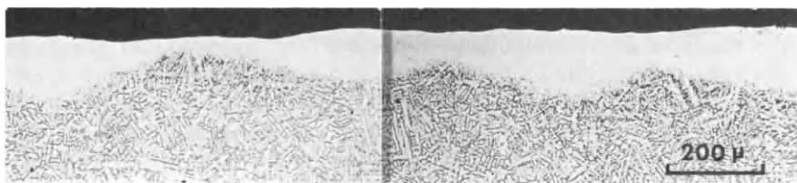
Fig. 5.16. Overlapping Laserglaze™ passes at 3.0 kW, 25 cm/s, in the 1.5 w/o B alloy from fig. 5.15(a) (VHN of melted region = 600 kg/mm 2 ).
