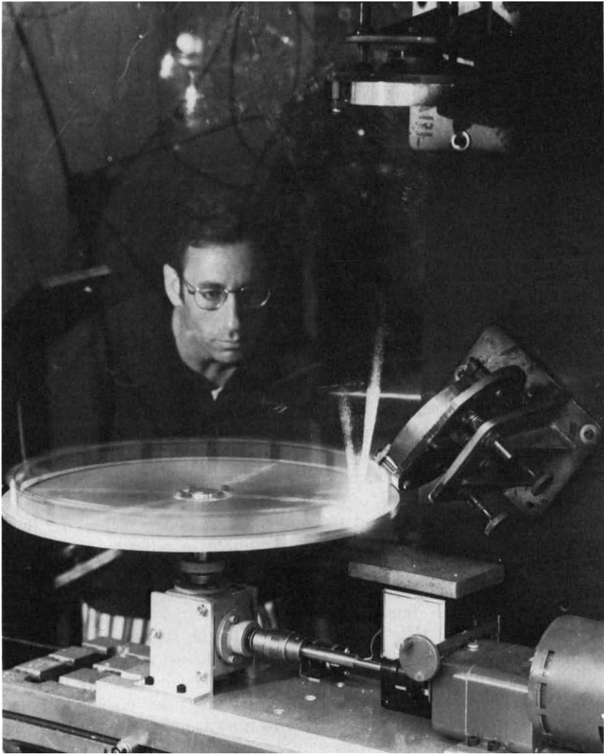
Fig. 5.30. Photograph of laserglazing being performed (gas shield removed for visibility).
