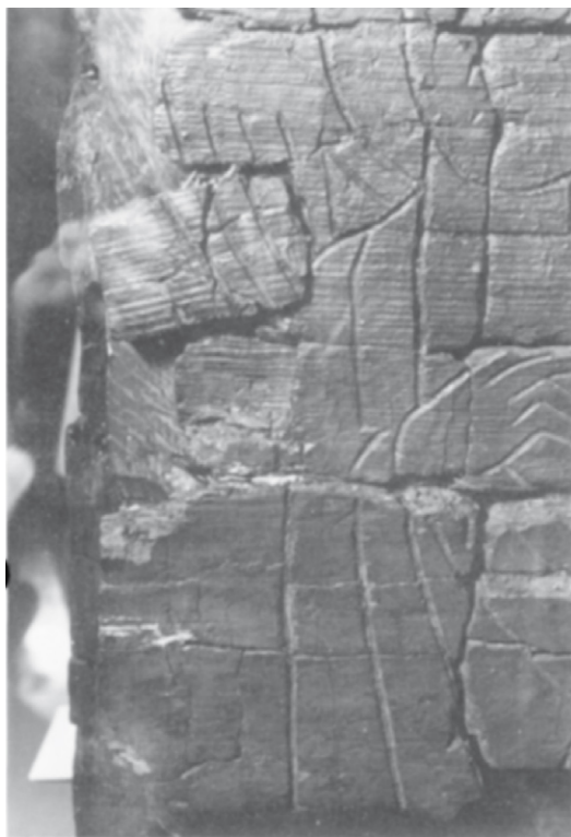
FIGURE 2.7 The slumping, after 30 years, of a piece of wood stuck in place with poly(vinyl acetate). Source: Cronyn and Horie (1985).
