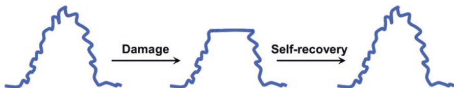
Fig. 2 Principle of self-recovery superhydrophobic surfaces based on restoration of surface topography
