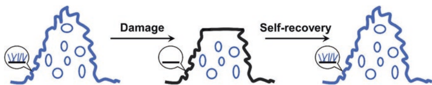
Fig. 6 Principle of self-recovery superhydrophobic surfaces based on the combination of low surface energy material migration and rough topography restoration. Blue represents the low surface energy materials; black represents the basic structural materials
