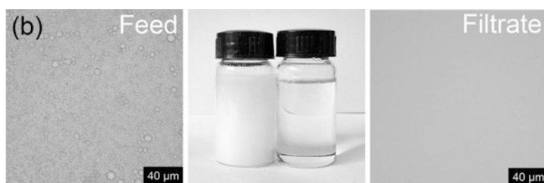
Fig. 7 Destabilization of an oil-in-water emulsion before (left) and after the oil is completely separated from water phase (right). Optical microscopy images allow comparing both vials during the separation process. (Reprinted with permission from Ref. [48], copyright Elsevier)
