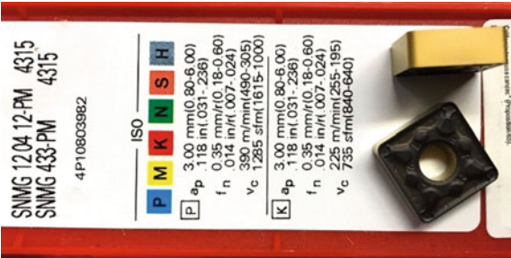
Fig. 1.7 Example of a box with cutting inserts where the recommended cutting speeds ( P —for steels, K —for cast irons)
