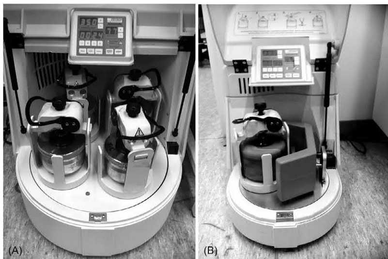
Figure 3.19 Photos of Fritsch planetary-type high-energy ball mill of (A) Pulverisette P5 and (B) Pulverisette P6. The equipment is housed in the Nanotechnology Laboratory, Energy and Building Research Center (EBRC), Kuwait Institute for Scientific Research (KISR).
