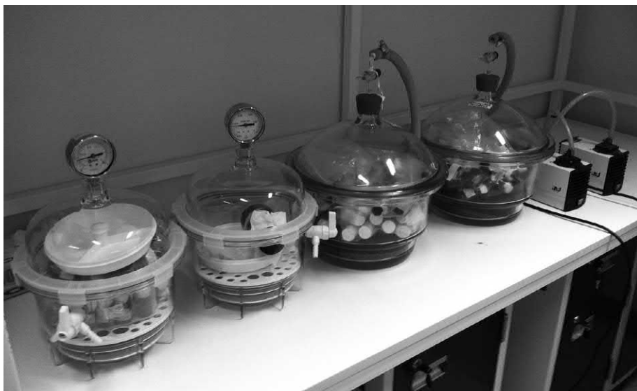
Figure 4.4 The powders of as-ball-milled samples are sealed under argon gas atmosphere in Pyrex glass bottles and stored in vacuum-silica gel dissectors. The photo taken from KISR-Nanotechnology Lab, Kuwait.
