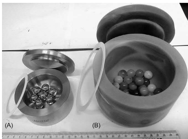
Figure 3.20 Photos of the vials used for Fritsch planetary ball mills with capacity of (A) 80 mL and (B) 500 mL. The vials and the balls shown in (A) and (B) are made of tempered steel agate materials, respectively (Nanotechnology Laboratory, Energy and Building Research Center (EBRC), Kuwait Institute for Scientific Research (KISR)).
