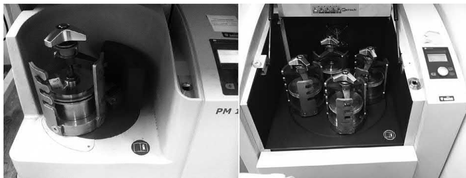
Figure 3.22 Photos of Retsch planetary-type high-energy ball mill of (A) PM 100 and (B) PM 400. The equipment is housed in the Nanotechnology Laboratory, Energy and Building Research Center (EBRC), Kuwait Institute for Scientific Research (KISR).
