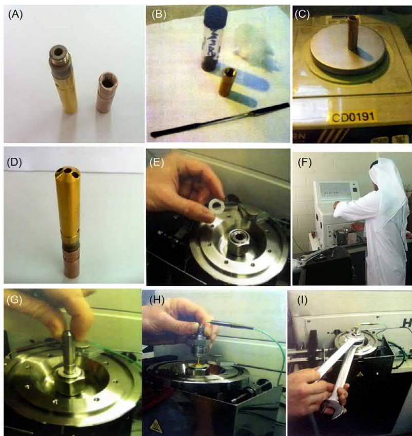
Figure 9.19 Photos present the several steps used to investigate the hydrogenation/dehydrogenation properties of as-prepared \text{MgH}_2 powders, using Sievert-type apparatus (Hidden Isotherma, IMI System, England, KISR-EBRC/NAM Lab, Kuwait).
