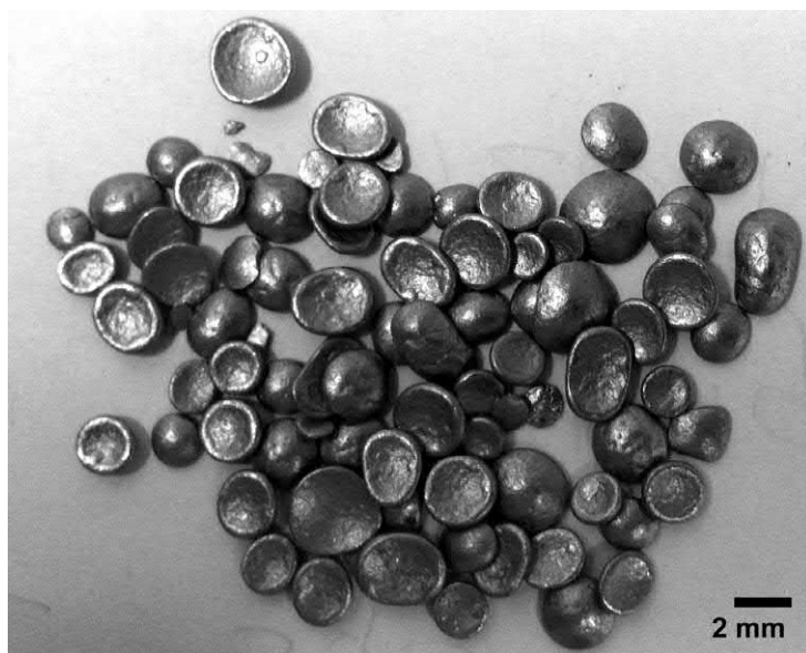
Figure 4.3 Photo of \text{Ni}_{33}\text{Al}_{67} powders after planetary dry ball milling for 25 h at rotation speed of 250 rpm in an argon gas atmosphere, using Cr-tempered steel milling tools and in the absence of PCA. (Unpublished work of the author)
