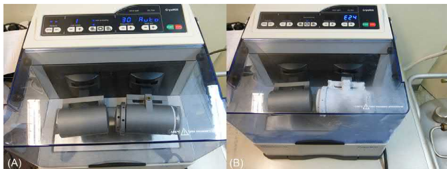
Figure 3.17 A photo of Retsch Mixer CryoMill. This type of high-energy ball mill can be used at (A) ambient temperature mode or (B) under flow of a liquid nitrogen. The equipment is housed in the Nanotechnology Laboratory, Energy and Building Research Center (EBRC), Kuwait Institute for Scientific Research (KISR).
