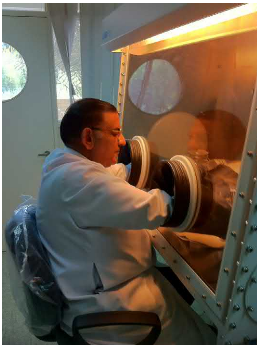
Figure 4.5 Photos taken from KISR-Nanotechnology Lab, Kuwait, for the author while handling the ball-milled powders inside a glove box (mBRAUN Glove Box, Dieselstr. 31, D-85748 Garching-Germany; http://www.mbraun.com ) under a helium gas atmosphere.
