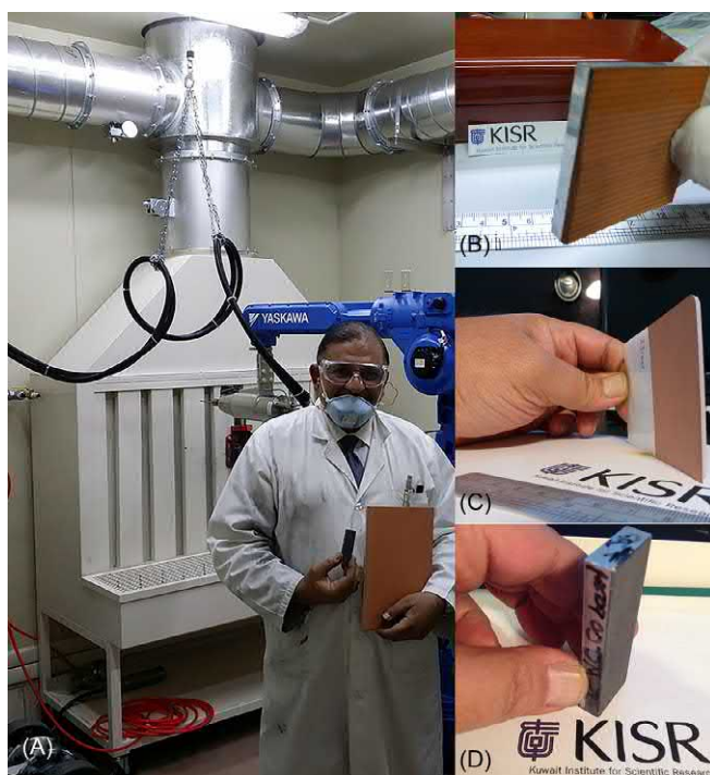
Figure 12.11 Combinations between particles' temperature, velocity, and size lead to a successful cold spraying processing for depositing wide range of (A) and (B) pure metals such as Cu onto a variety of substrate materials including steel (A and B) or polymers (C). Cold spraying can be used also for deposition of hard composite materials such as WC-Co-based nanocomposite powders. (The photo presents the author in the cold spray laboratory with the cold-sprayed substrate samples achieved by a cold spray equipment provided by Startack Co. Ltd., housed in the Nanotechnology Laboratory, Energy and Building Research Center (EBRC), Kuwait Institute for Scientific Research (KISR).)
