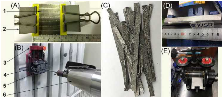
Figure 12.23 (A) The as-CR Mg strips (1) were mounted and fixed by clips (2) on stainless steel (SUS304) sheet, (B) two-movable jaws (3) were used to fix the sample that was aligned to be perpendicular to the nozzle (5) of cold spray (CS) gun (6). A photo presenting Mg-strips after coating with Ni powders for 3 times is shown in (C). The as-coated Mg-strips were wrapped with balance papers and placed between two-jaw type vise for 16 h (D), and then CR for 10 times to ensure straightening (E). [26]
