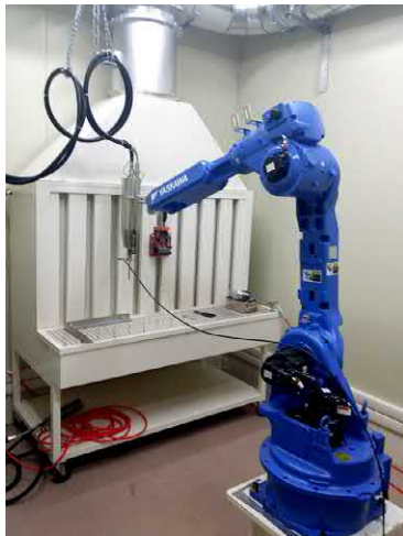
Figure 12.1 Robotic system of a cold spray equipment provided by Startack Co. Ltd., Japan, housed in the Nanotechnology Laboratory, Energy and Building Research Center (EBRC), Kuwait Institute for Scientific Research (KISR).
