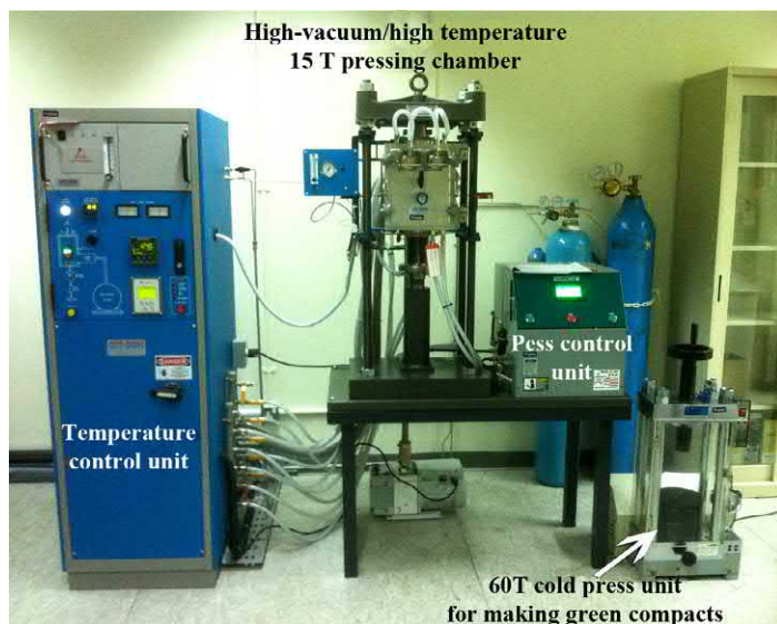
Figure 5.11 High vacuum/temperature hot press (OXY-GON, USA) employed for powder consolidation in the Nanotechnology Laboratory, Energy and Building Research Center (EBRC), Kuwait Institute for Scientific Research (KISR).
