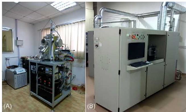
Figure 12.2 Typical electron beam physical vapor deposition (EBPVD, manufactured by Blue Wave Semiconductors, USA) and chemical vapor deposition (CVD, manufactured by First Nano, USA) equipment used in coating processes. (The equipment is housed in the Nanotechnology Labs, EBRC-KISR.)
