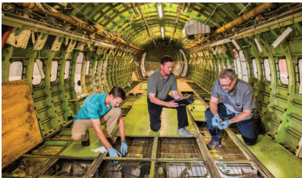
Sandia National Laboratories senior scientist Dennis Roach, center, works inside the cabin of a B737 test bed, installing and acquiring data from structural health monitoring sensors. Sandia mechanical engineers Stephen Neidigk, left, and Tom Rice, right, are also part of the monitoring team.
