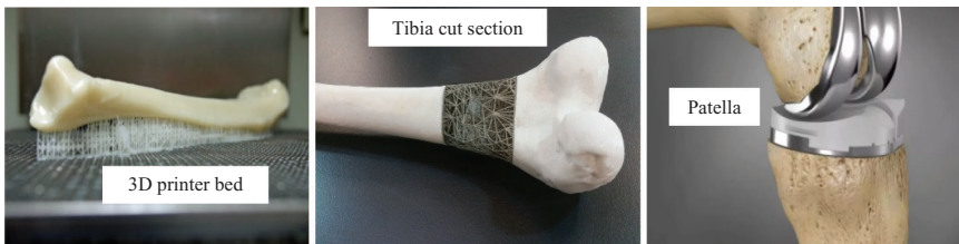
Figure 2.12 (a) 3D-printed tibias complete with supports at the bottom during additive manufacturing. (b) 3D-printed tibias with inner supports in hollow portion shown through cut section. (c) 3D-printed patella fitted on the defective bone of the lower leg and tibia.
