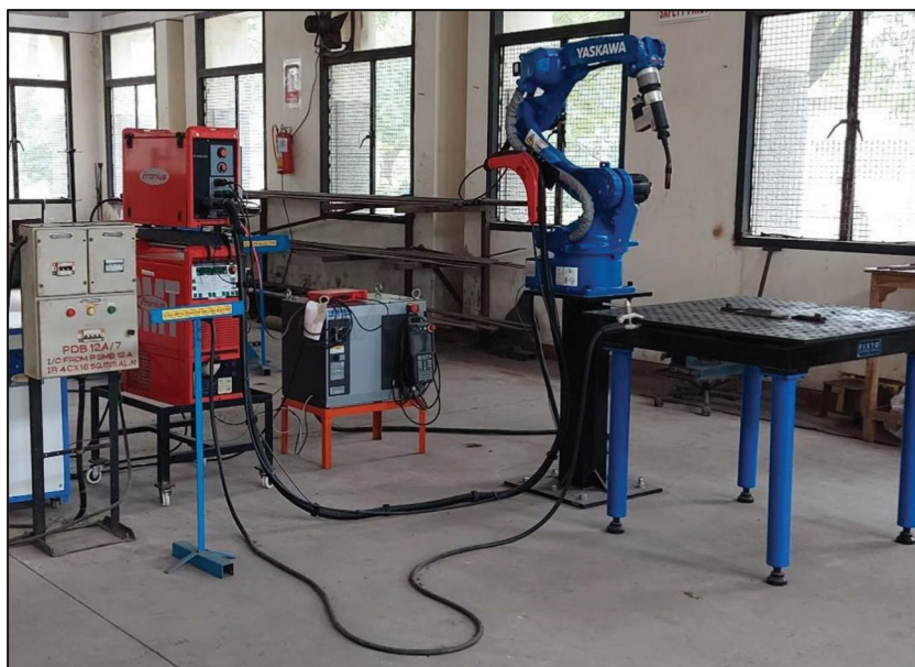
Figure 16.9 Robotic CMT-WAAM arrangement at Welding Research Cell, SVCE.
