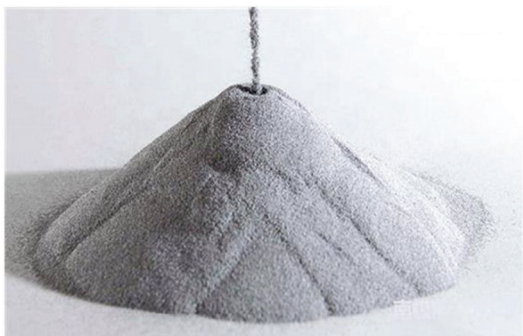
Figure 17.1 AlSi10Mg alloy powder.
