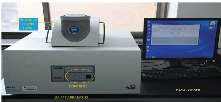
Figure 11.7 Photographic view of Netzsch LFA 447 apparatus used for the measurements.
