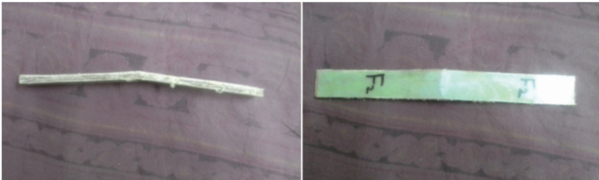
Figure 6.5 Flexural tested specimen.
