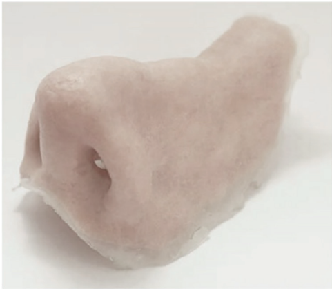
Figure 2.22 A customer-specific nose prosthetics made from silicone using 3D printer.
