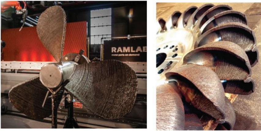
Figure 16.6 WAAM products – propeller [10] (left side) and turbine [11] (right side).
