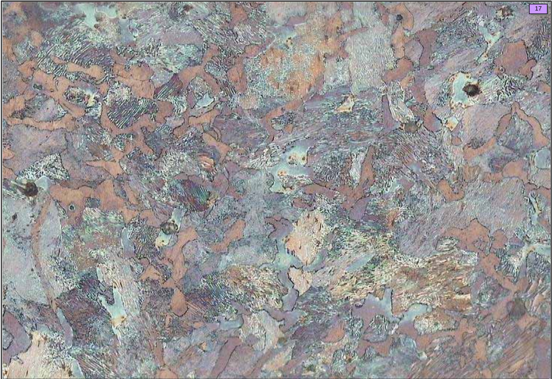
Photo.24: 500x, Same as in Photo.23, but in the larger area. The microstructures consist of Pearlite and Ferrite.
