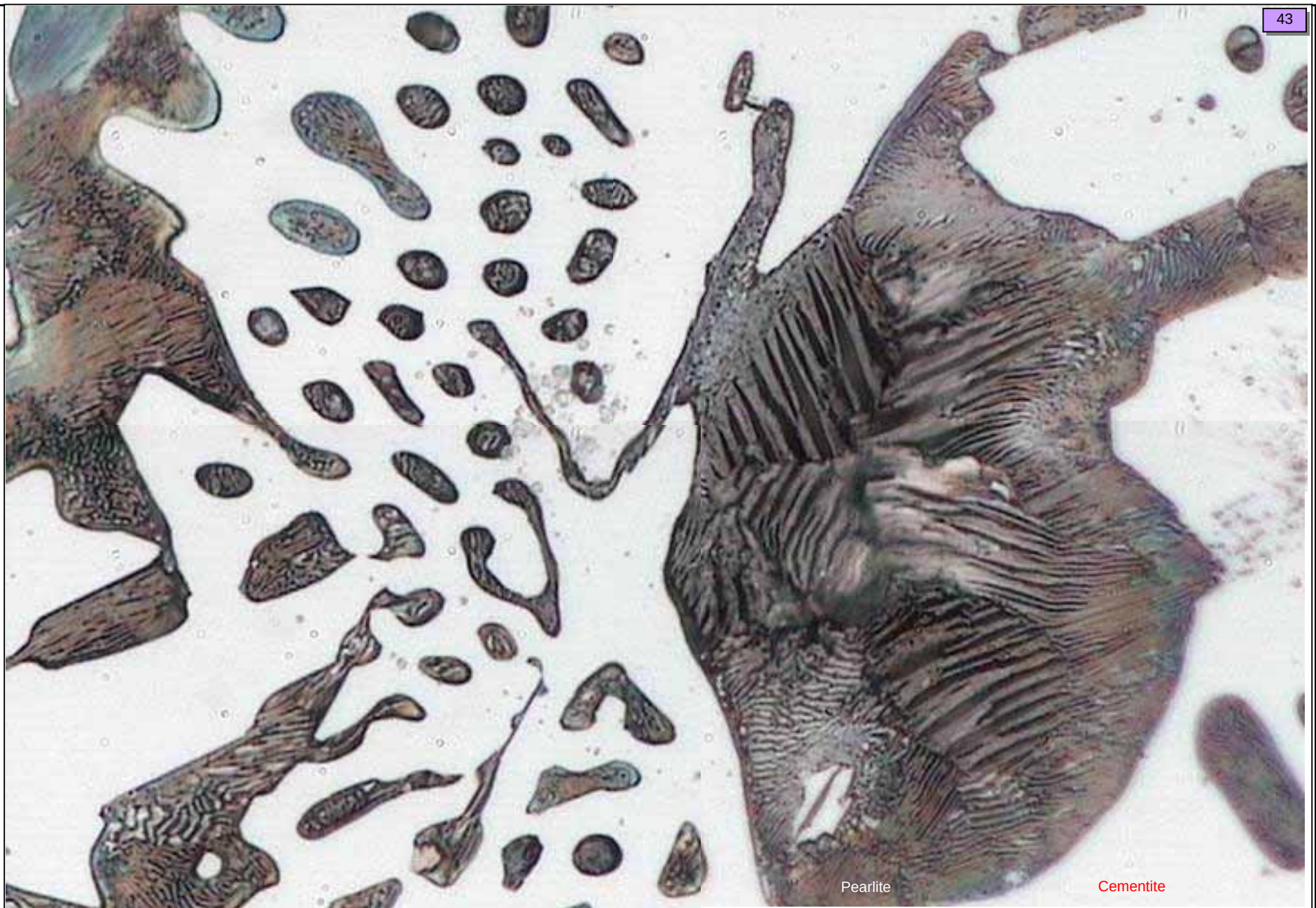
Photo.63:1000x, Same as in Photo.62, but in larger area, showing Pearlite, and Ledeburite.
