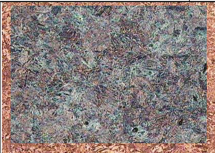
Photo.49:100x, Microstructures are Pearlite and ferrite.
