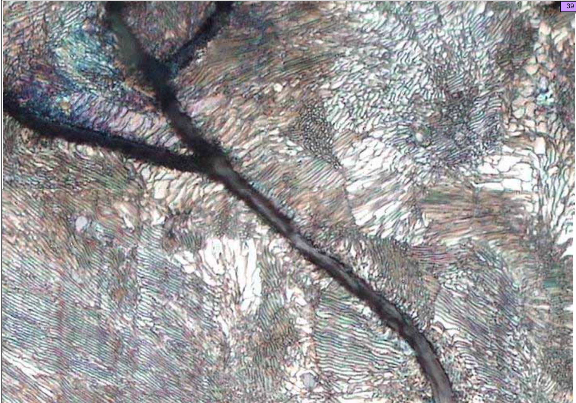
Photo.57: Same as in photo.56, but in larger area. Dark gray branches are graphite flakes. The matrix consists of Pearlite (small lines of cementite and Ferrite), and Ferrite.
