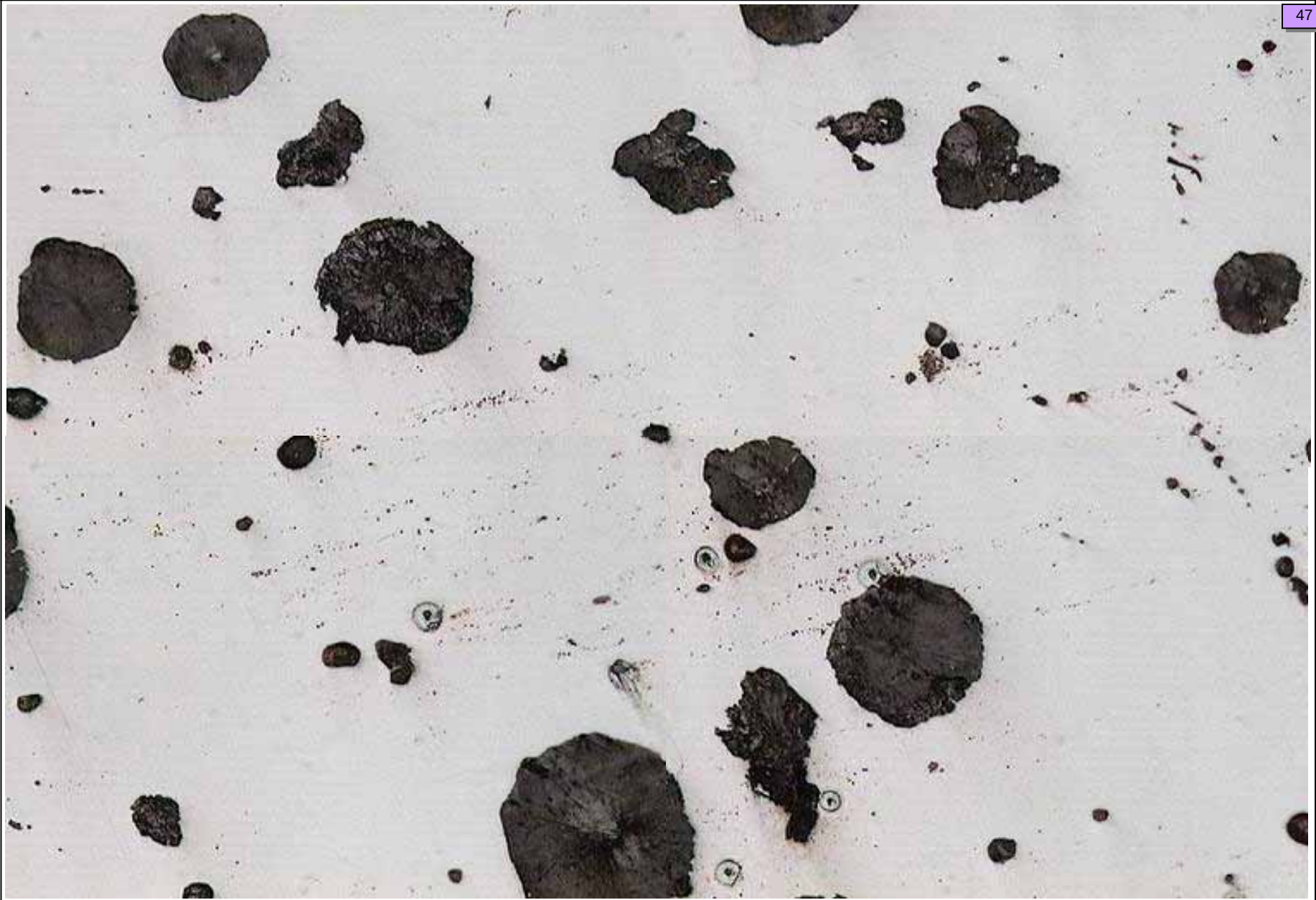
Photo.69:200x, Round particles are spheroidal graphites. The matrix can not be revealed in unetched condition.
