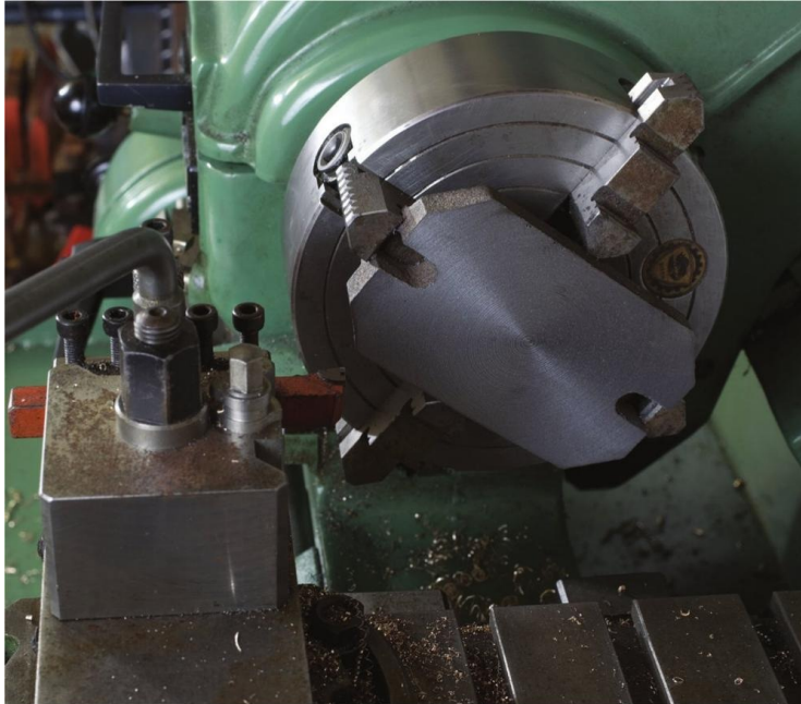
A base plate casting in a four-jaw independent chuck.
