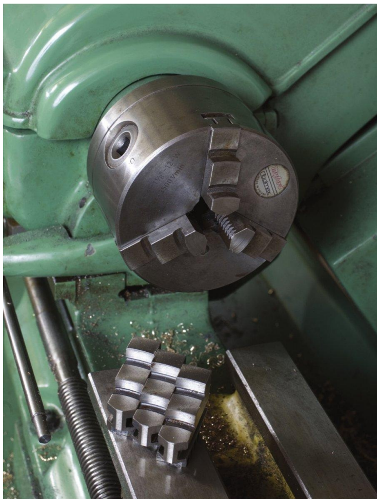
A self-centring three-jaw chuck fitted with 'drill jaws'. Note the external jaws, which are interchangeable with the drill jaws.
