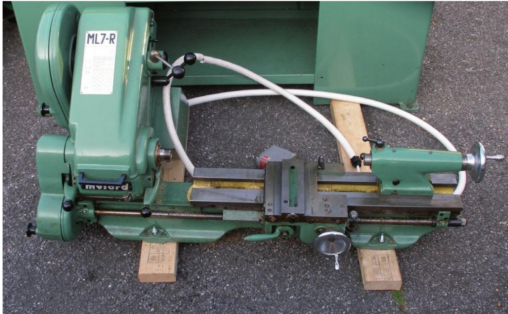
Two planks of wood bolted to the lathe feet will often turn an unmanageable mass of metal into an easily handled machine.
