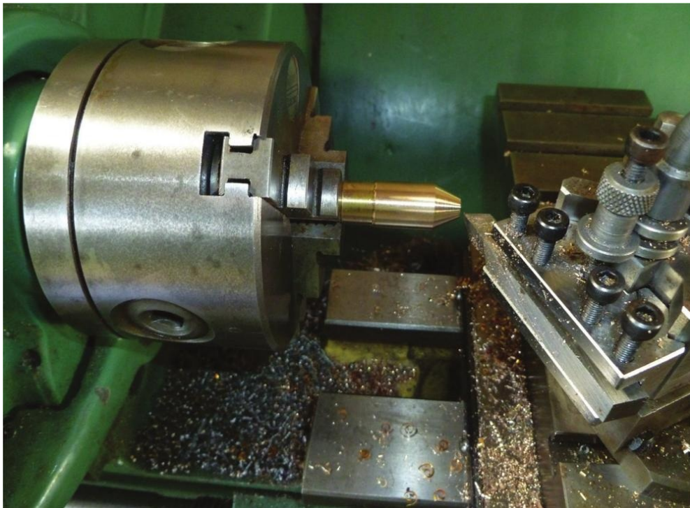
Turning a taper with the topslide.
