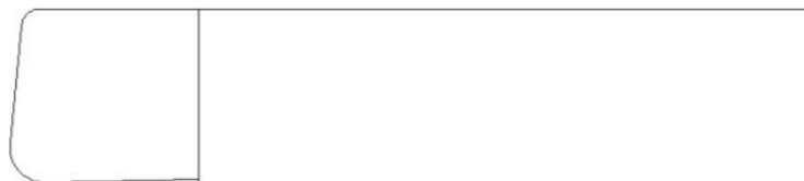
Shallow boring tool capable of facing across the bottom of a hole.
