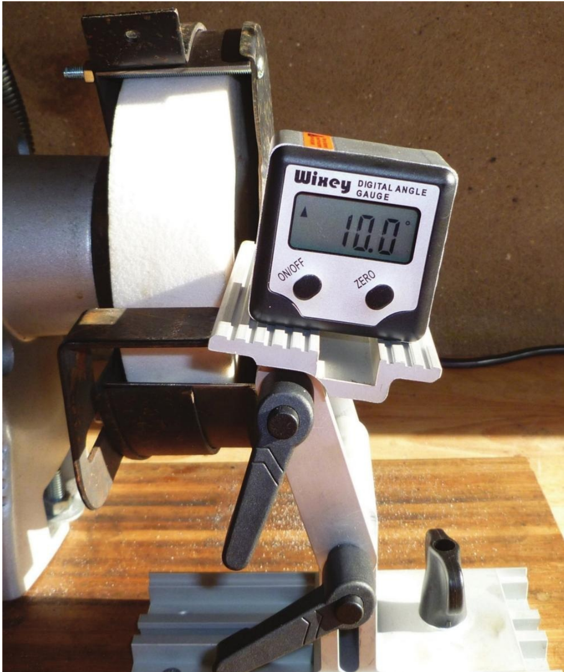
The grinding rest is set to the correct angle of 10 degrees to grind the end of the tool.
