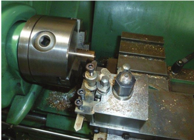
Double-ended chamfer tool chamfering a diameter.
