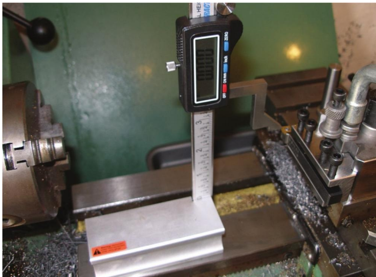
Setting the height of the tool.
