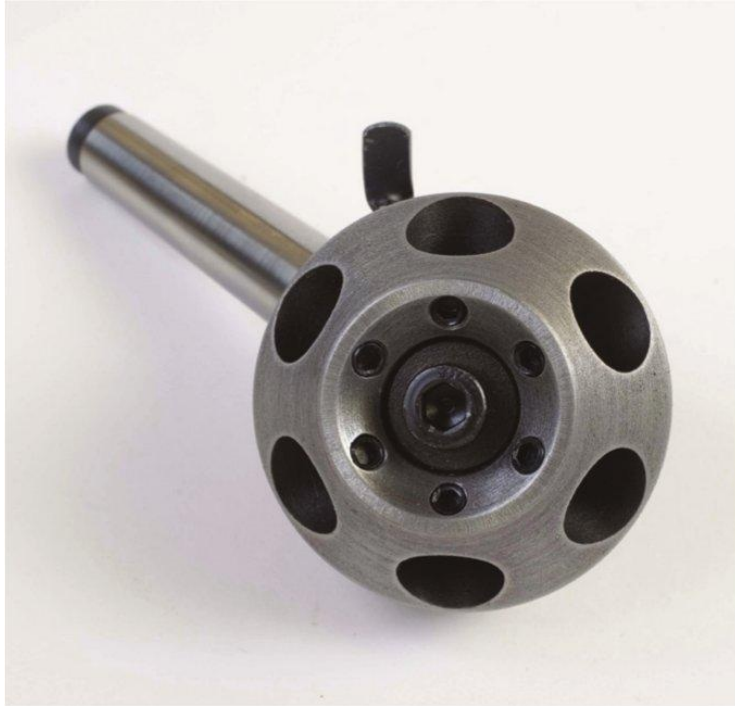
An indexing turret that fits directly into the tailstock of the lathe.
