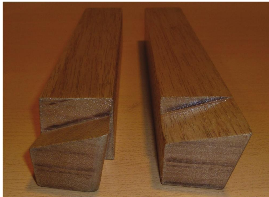
The left-hand tool is suitable for both facing and turning; the right-hand tool is suitable for turning only.
