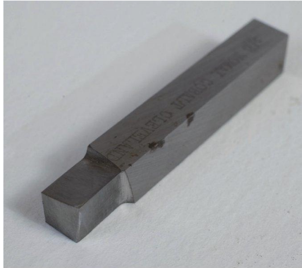
A general-purpose HSS turning tool suitable for mild steel.
