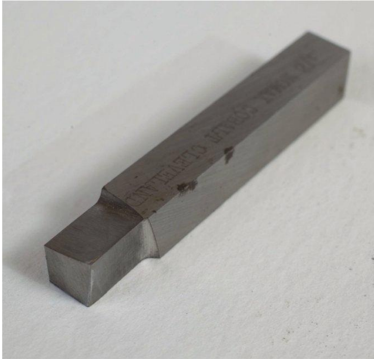
The third angle has been ground.
