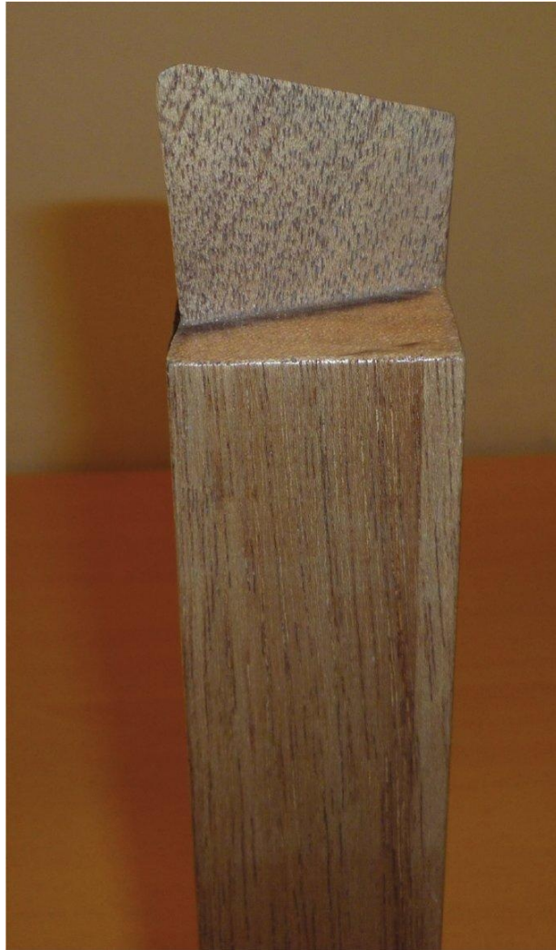
Top of the facing and turning tool, showing the front and side relief.
