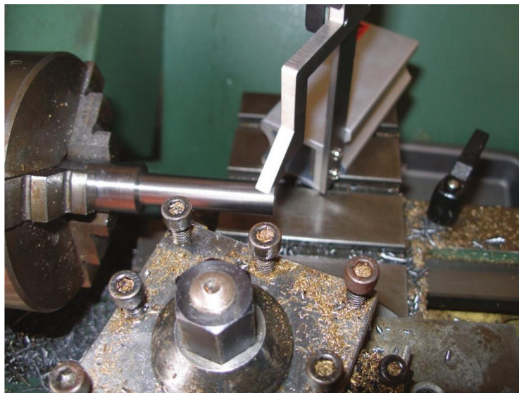
Measuring the height of the bar above the cross slide.
