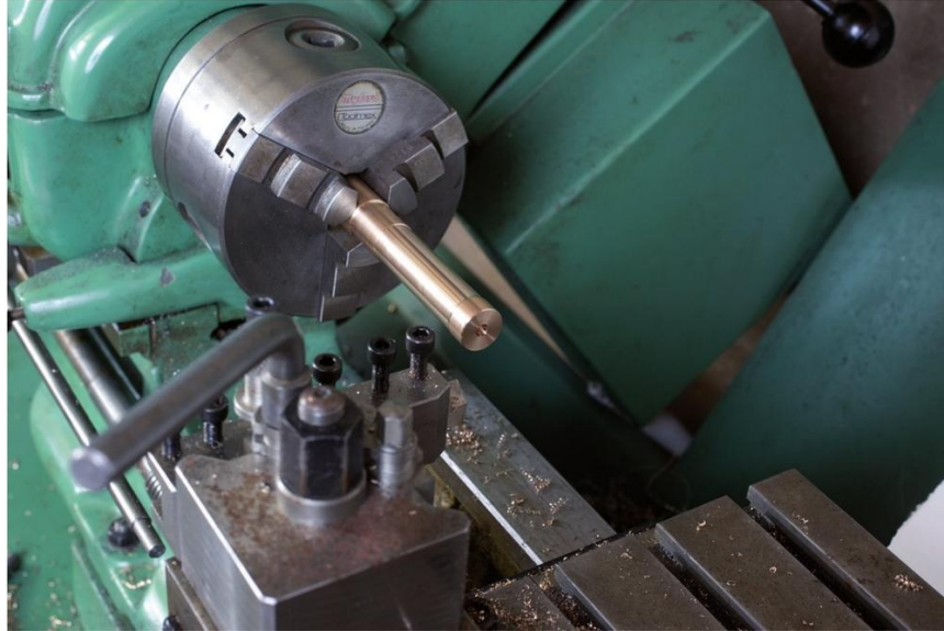
Using a test bar to check for parallel turning.
