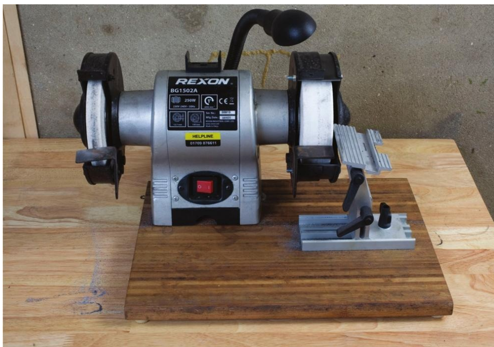
The guard of this off-hand grinder has been widened to accept a recessed wheel.
