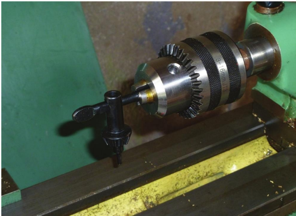
This drill chuck requires a chuck key.
