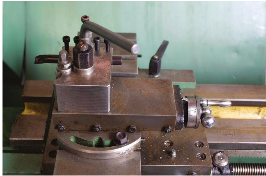
The top slide is mounted on the cross slide.
