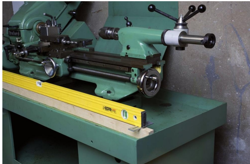
Put the spirit level on the cabinet's longitudinal axis and use the adjustable feet to level the lathe.
