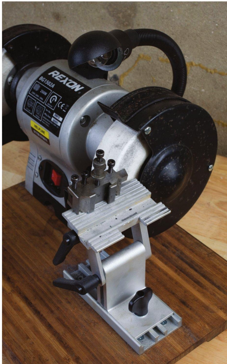
Grinding the second angle.
