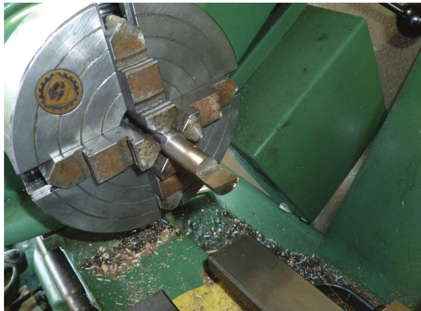
Boring the hole using the four-jaw chuck method.
