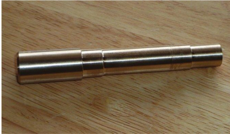
The finished shaft.
