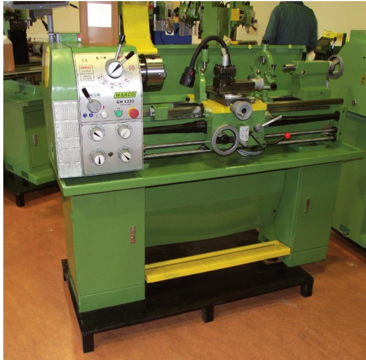
A larger industrial lathe with a foot-operated emergency cut-off switch and brake.
