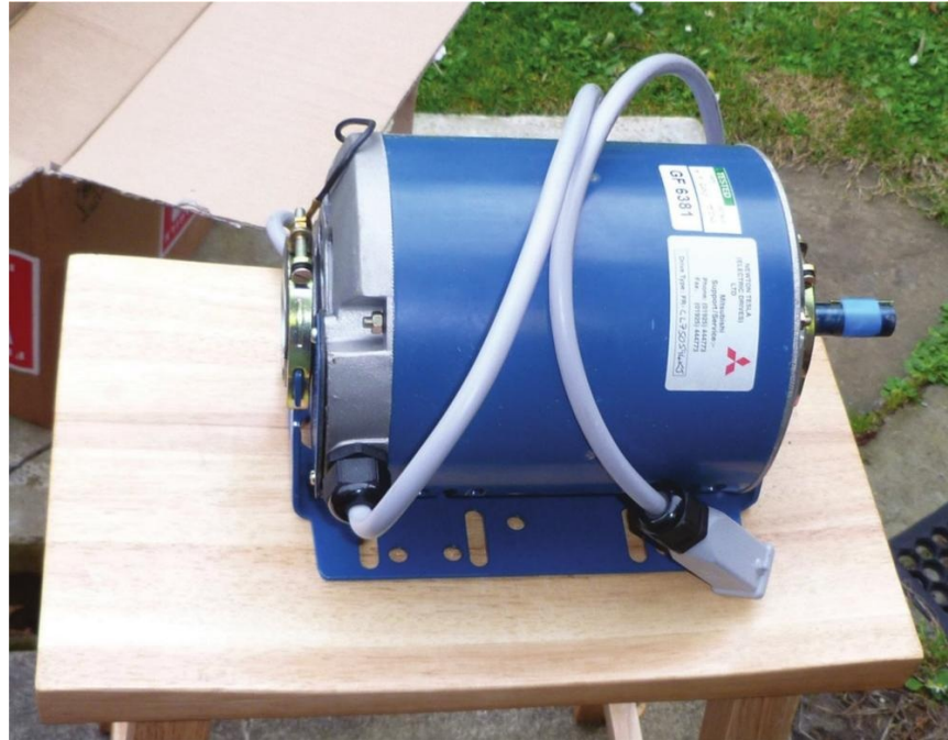
This motor is part of the inverter package shown in the previous illustration. No wiring is involved as the motor lead plugs straight into the inverter box.
