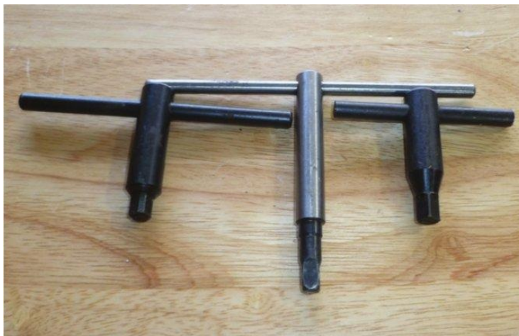
Although most lathe chuck keys have square ends, they are often of different sizes. Keep each key with its own chuck.
