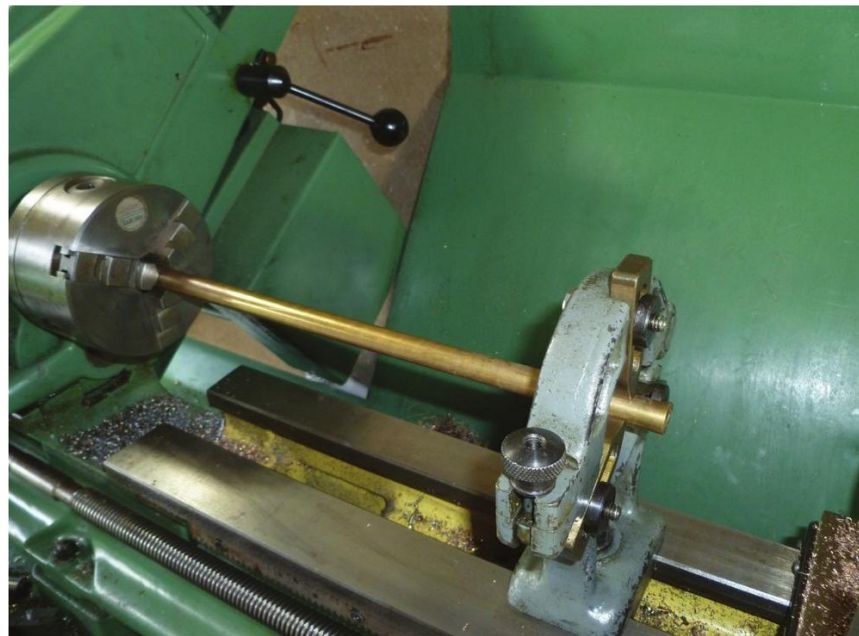
Using the fixed steady.
