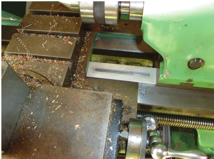
A useful tailstock end back stop method.
