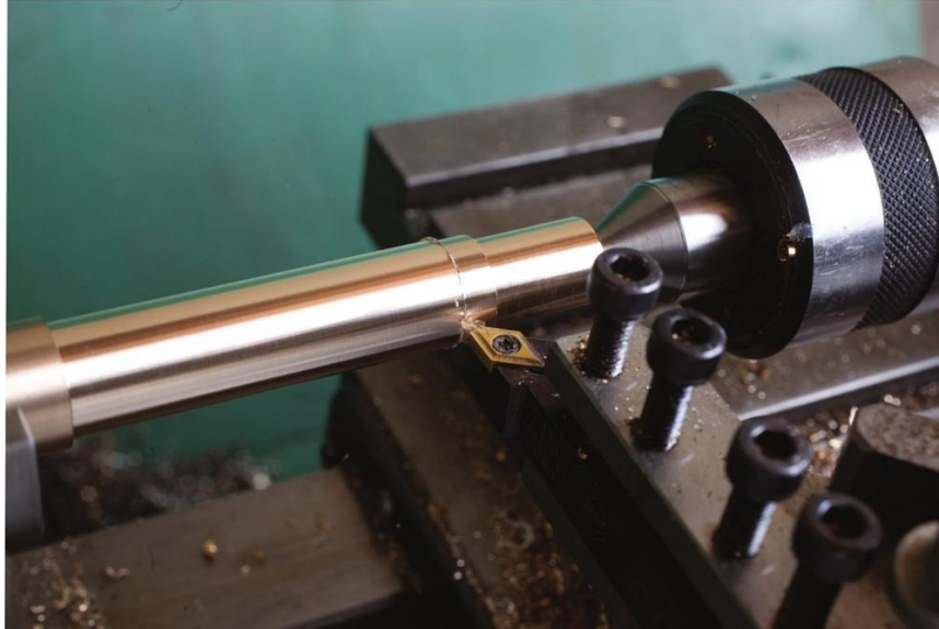
Turning a step on a bar using the stop. The bar is held in the three-jaw chuck and supported with the tailstock centre.
