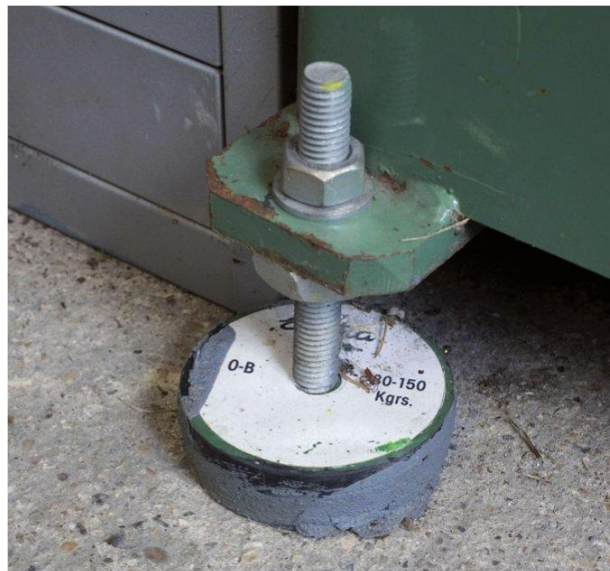
Adjustable feet are very useful for levelling up the lathe.
