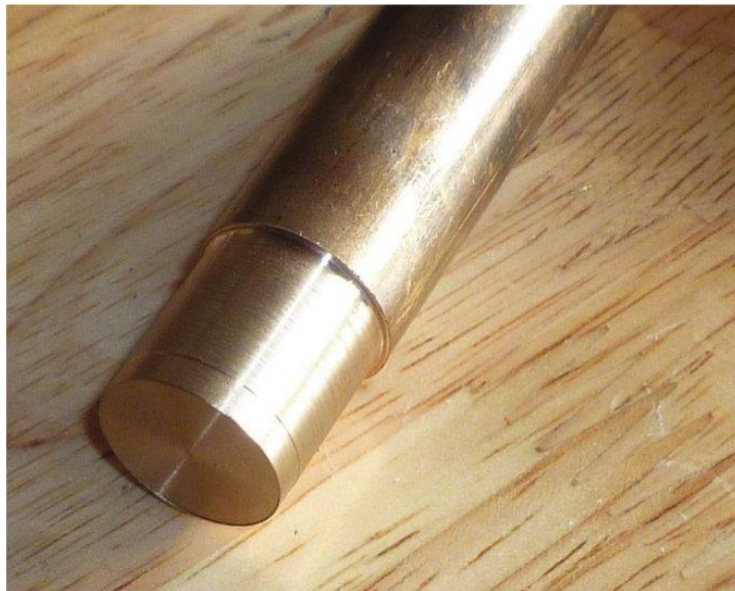
Checking a bore with a home-made gauge. The lead in is one thou smaller than the bore required.
