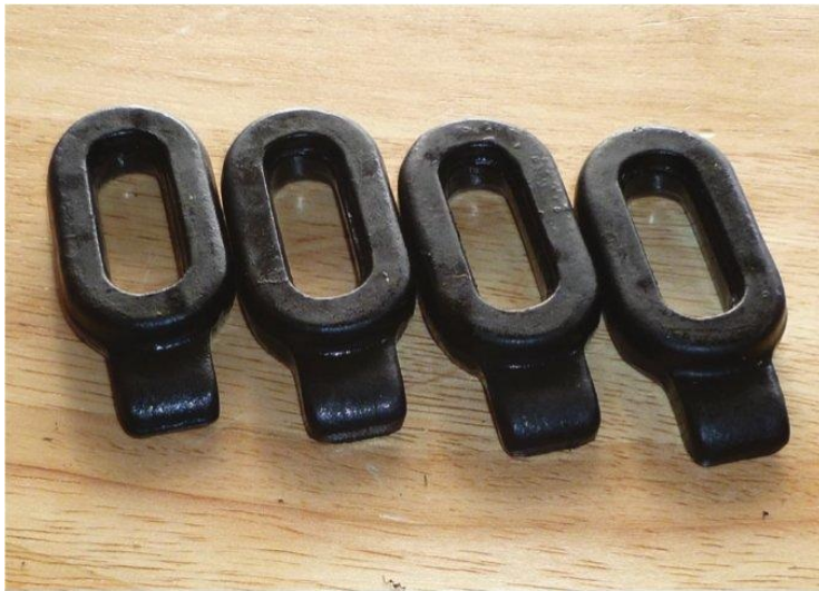
A simple clamp set is very useful when machining a casting on the faceplate.
