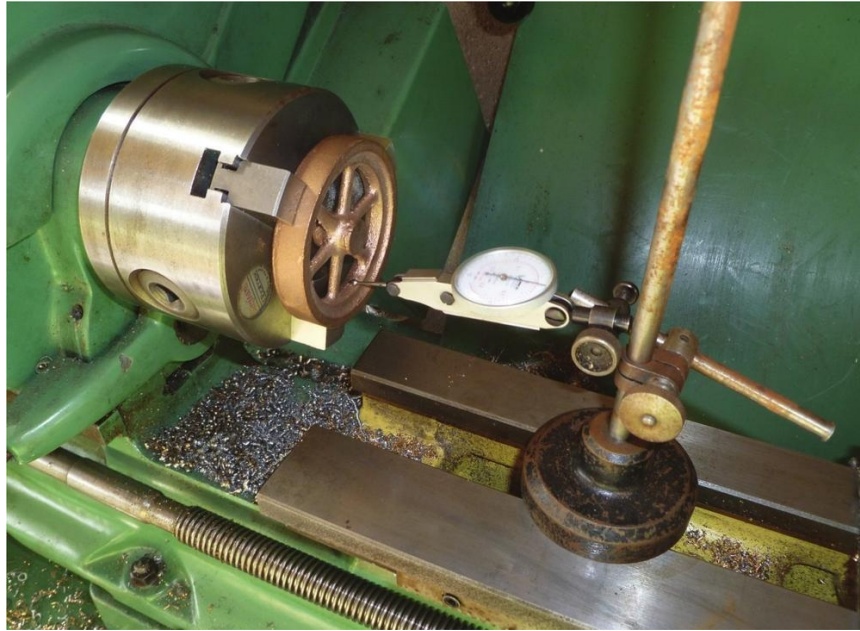
Using a scribing block with a dial test indicator.
