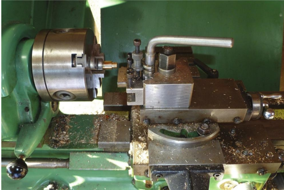
Cutting a screw thread with the top slide set parallel to the lathe.
