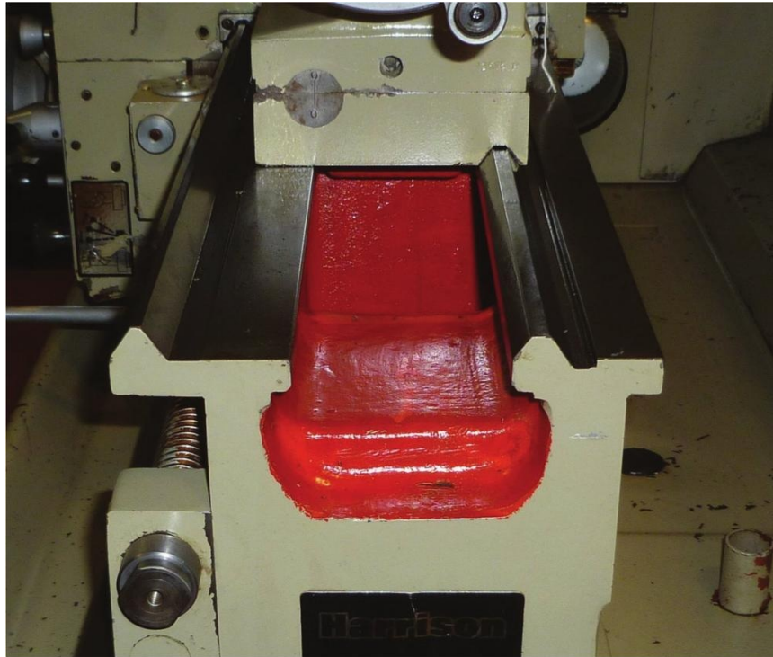
A lathe bed with raised and inverted Vees. The carriage usually slides on one set of Vees and the tailstock slides on the other.
