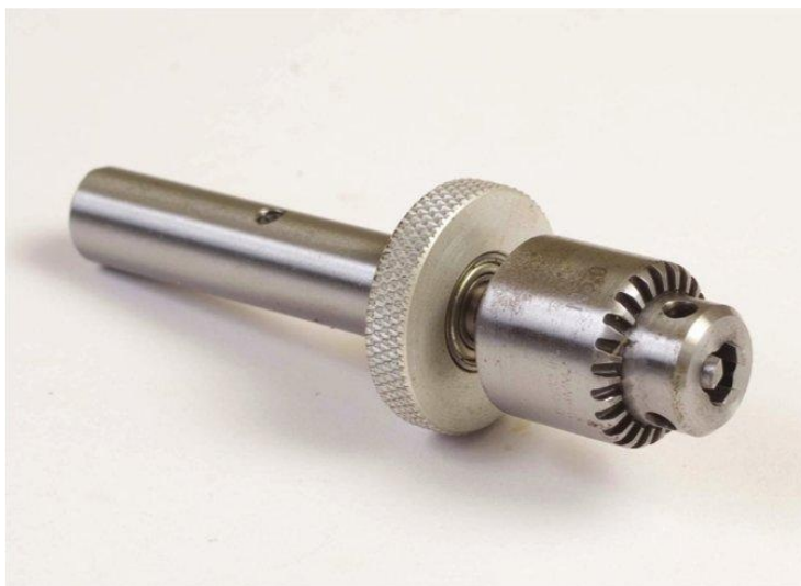
A sensitive drilling attachment that fits into the
