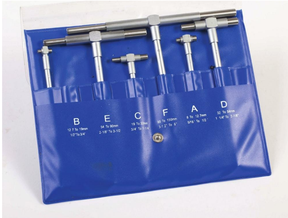
A set of telescopic gauges for checking a bore, used in conjunction with a micrometer.
