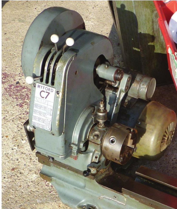
The Myford TriLeva attachment will only fit ML7 and C7 lathes and is not suitable for ML7R or Super 7 lathes.
