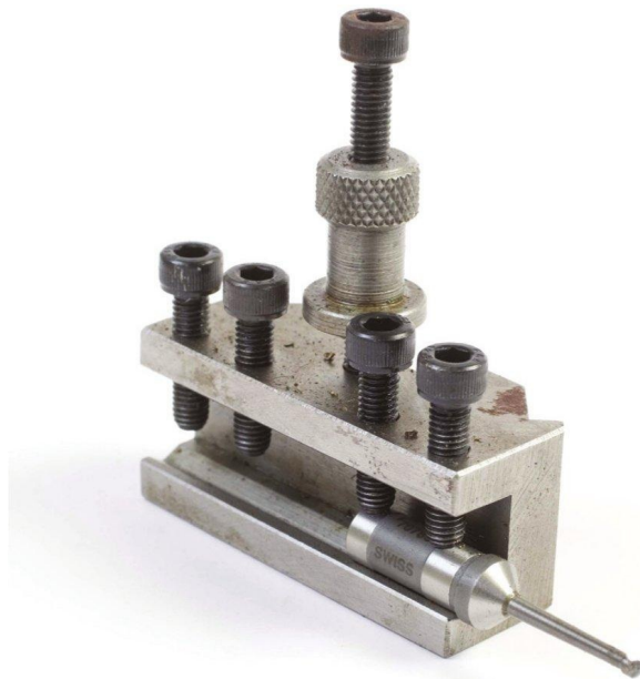
Standard tool holder with a Vee to take round tool holders.
