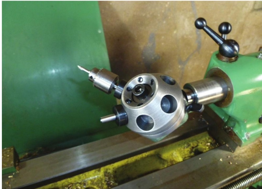
An indexing turret set up with a stop and a centre drill.
