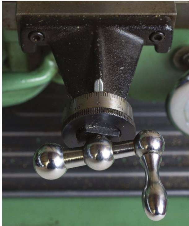
Zero setting dials make turning and screwcutting to depth very easy.
