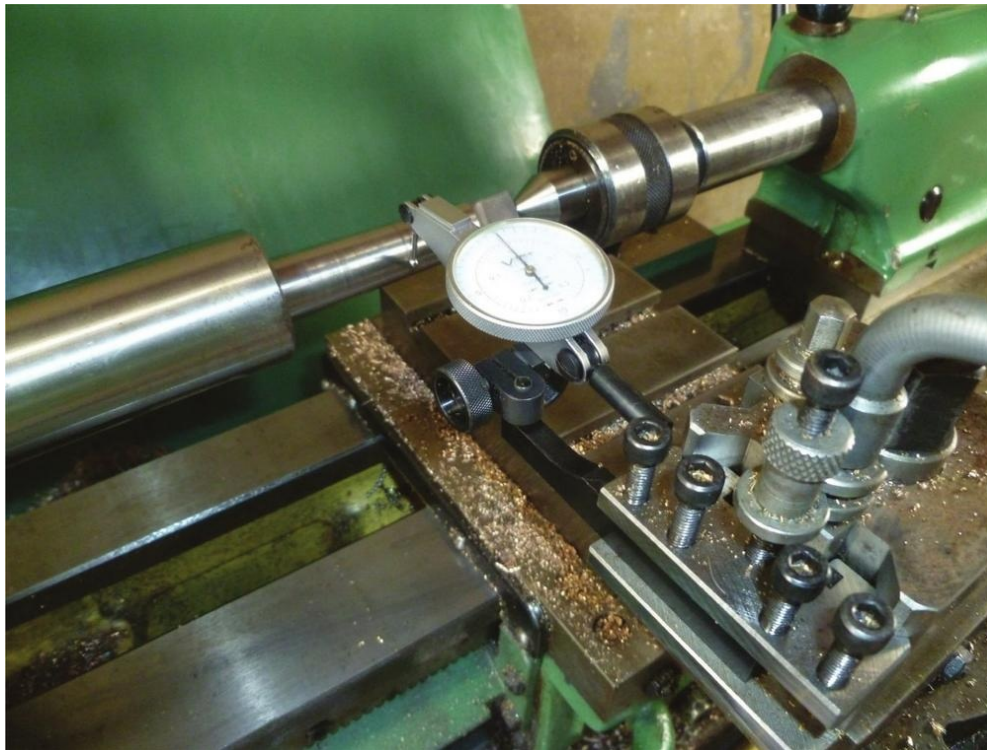
Setting the top slide by clocking an existing taper.
