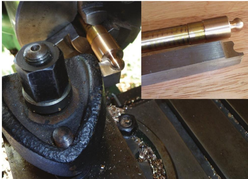
A form tool cutting a ball. The inset view shows the form tool and a finished ball.
