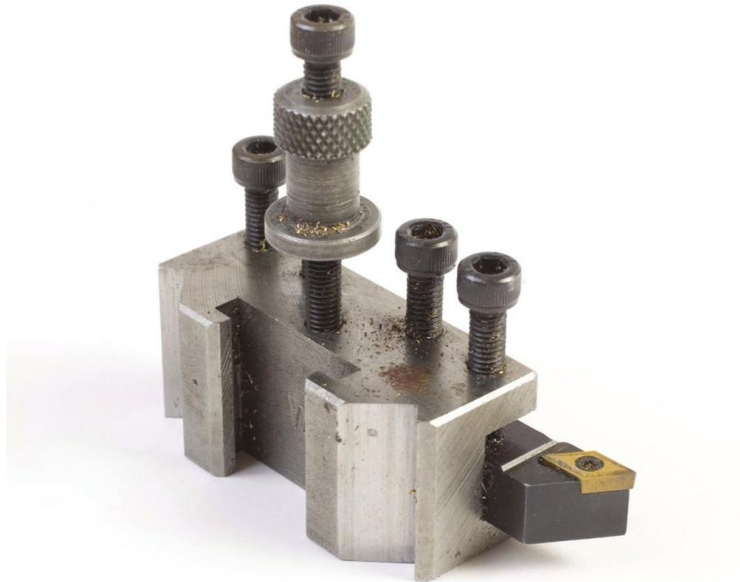
Back of a quick-change tool holder, showing the dovetail type of mounting.
