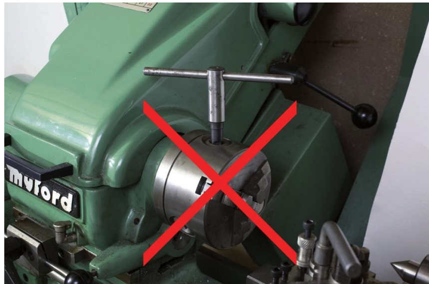
Do not leave the chuck key in the chuck.
