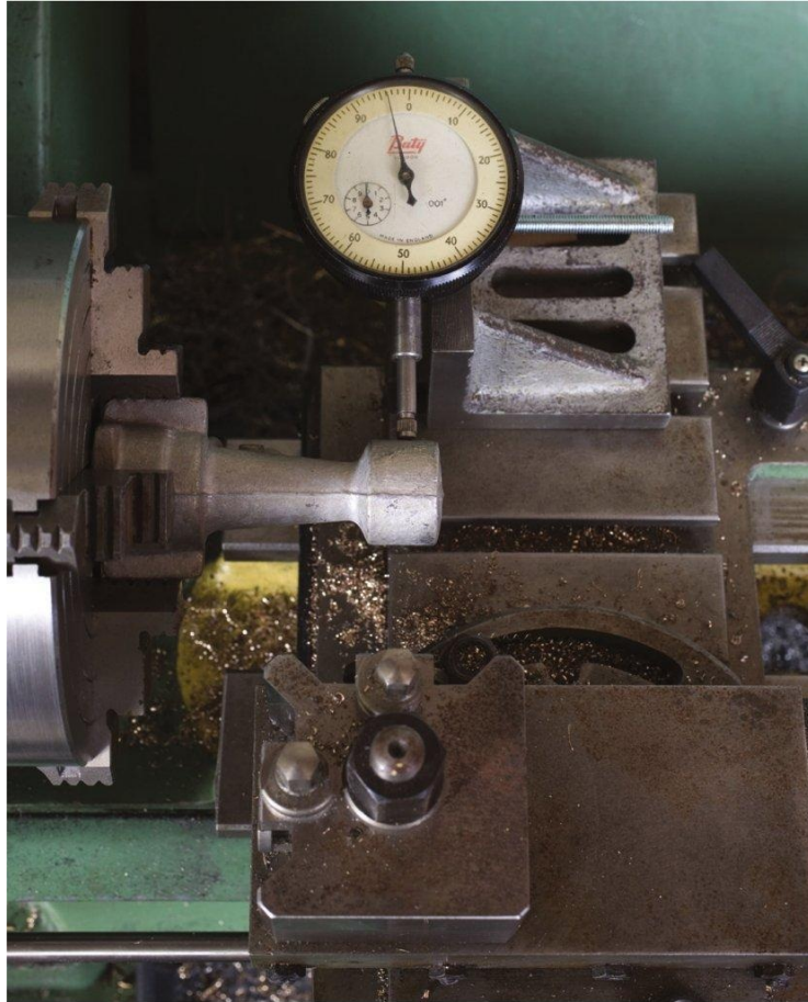
Clocking the end of a casting in a four-jaw chuck.
