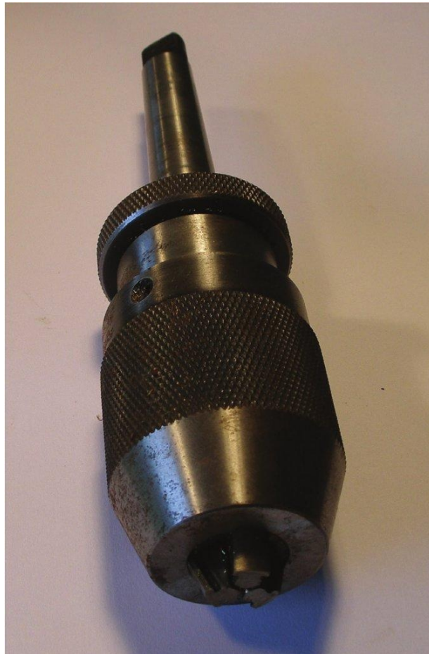
Hand-tightening drill chuck.
