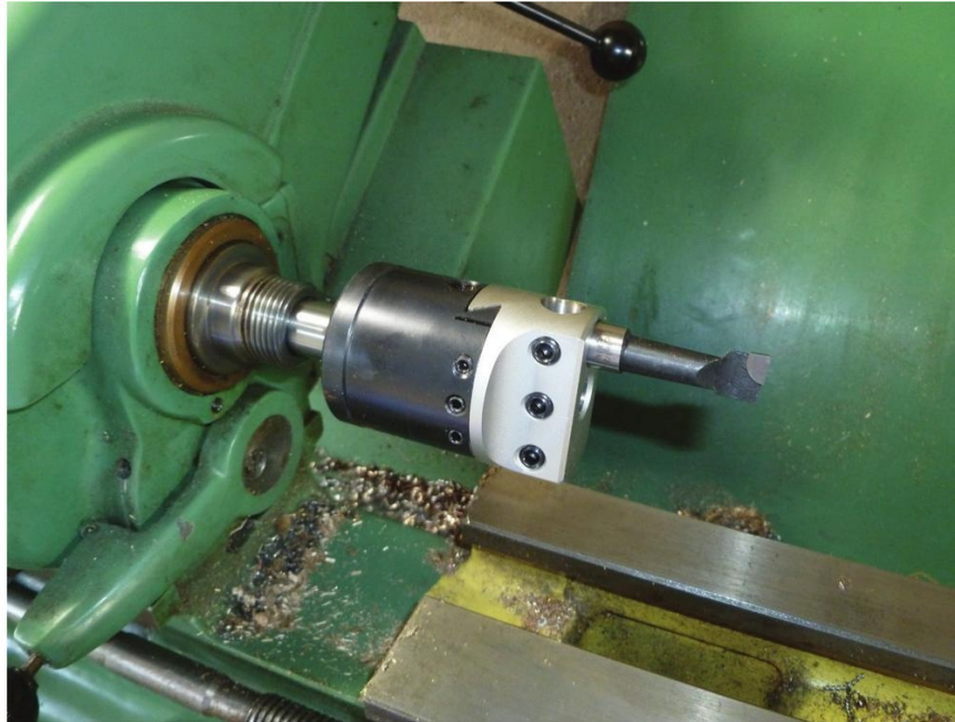
Using the boring head in the lathe mandrel.
