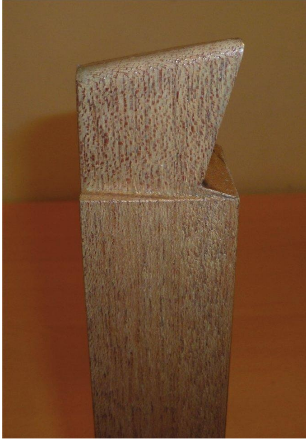
Left-hand side of the facing and turning tool, showing the front and top rake.
