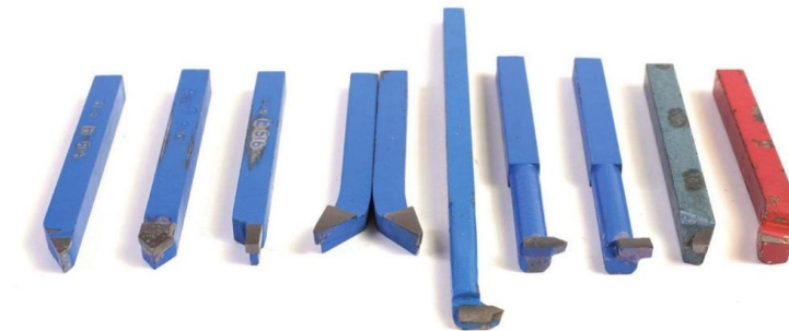
Brazed-on carbide-tipped tools come in various grades, shapes and sizes.
