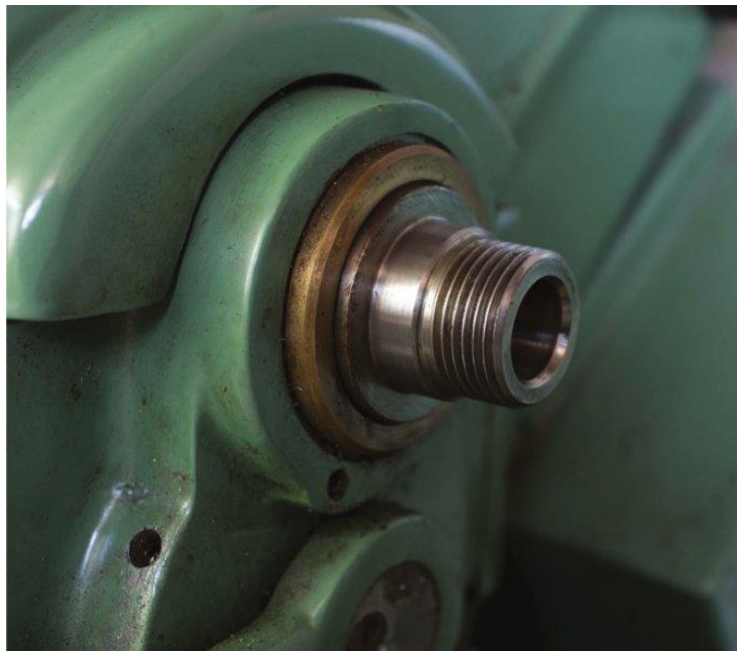
Close-up view of a Myford headstock on an ML7R. Note the large bronze bearing at the front. The earlier ML7 lathes had white metal bearings, although the C7 capstan had bronze bearings and a hardened lathe spindle.
