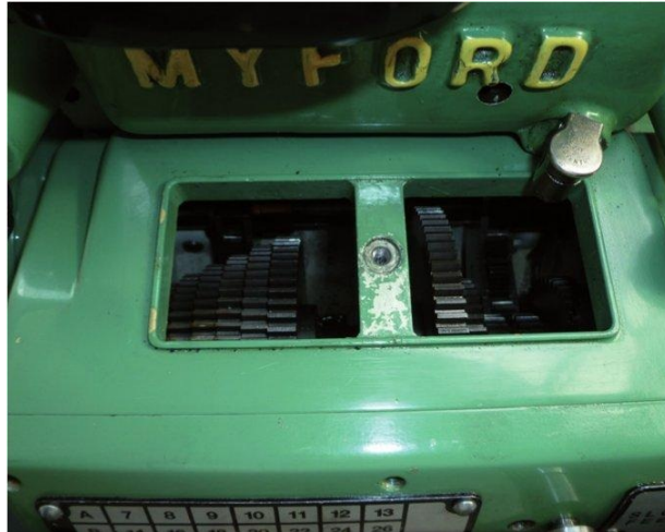
The cone gears inside a typical Norton screwcutting gearbox (not an original Myford one).
