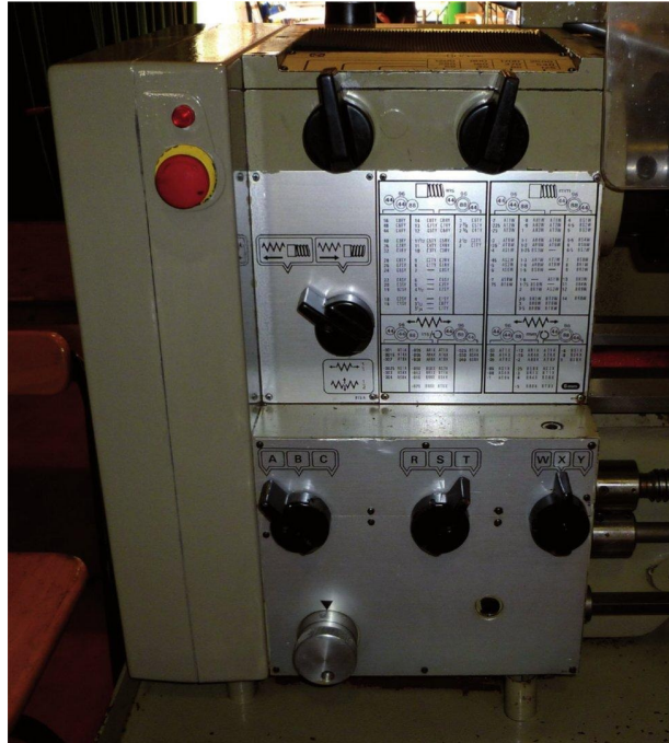
An all-geared head on a modern industrial size lathe.
