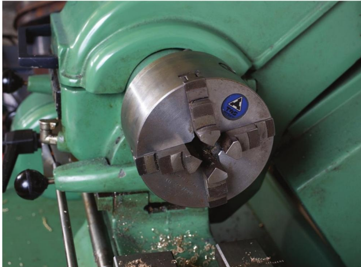
A self-centring four-jaw chuck. These also come with external jaws and soft jaws are usually available.
