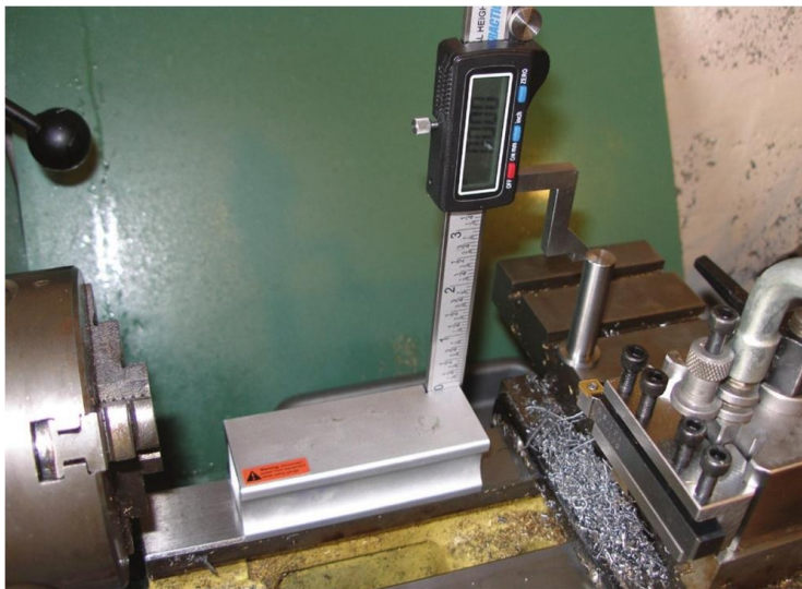
Setting the height gauge to the lathe centre height.
