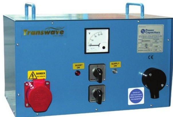
This static converter is suitable for powering one 3 phase motor. If you fit a socket on the output, however, different individual machines can be plugged into it, one at a time.
