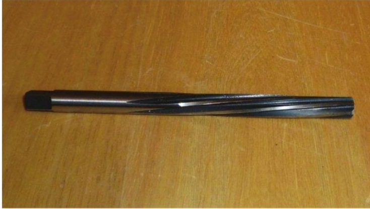
Hand reamer; the front part has a slight taper.
