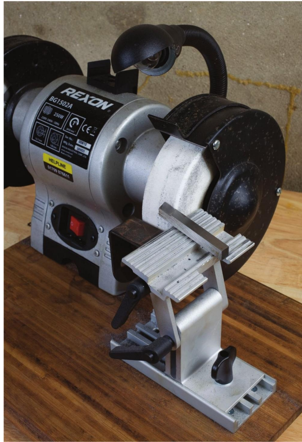
Grinding the third angle.
