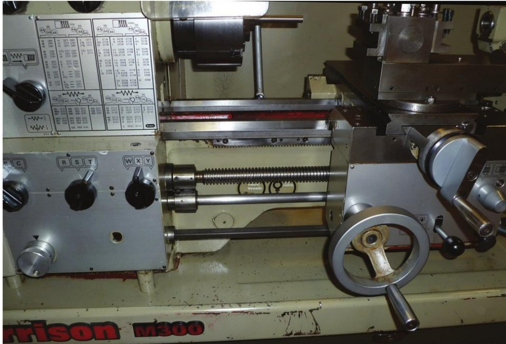
This lathe has both a leadscrew for screwcutting and a drive shaft for the saddle and cross slide feeds.
