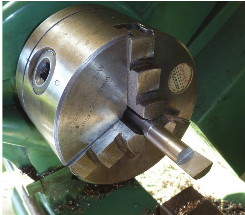
To bore the hole, the first option is to hold a boring bar in the three-jaw chuck. This is a good basic method of boring a workpiece on the cross slide. The only awkward bit is adjusting the boring bar so that a size hole is bored. This is usually done by an adjusting screw pressing onto the back of the tip opposite the cutting edge. The tip itself is usually clamped by a grub screw through the side of the boring bar. However, you can use a boring bar that is a few thou under the required size and finish off with a reamer.
