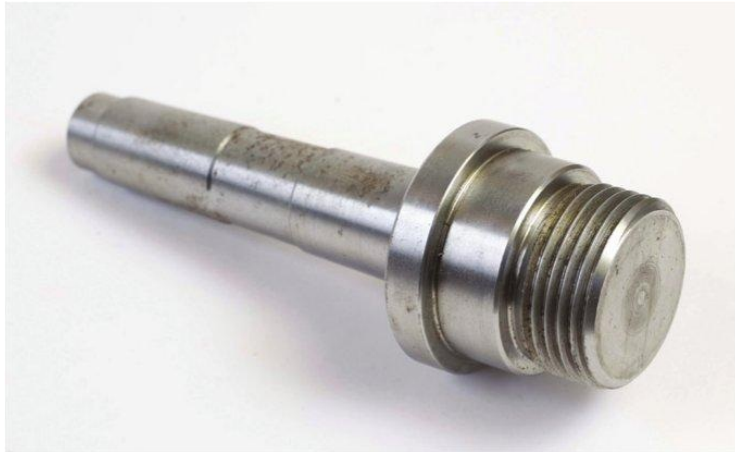
The steady can be set using a chuck mounted on this tailstock adaptor.
