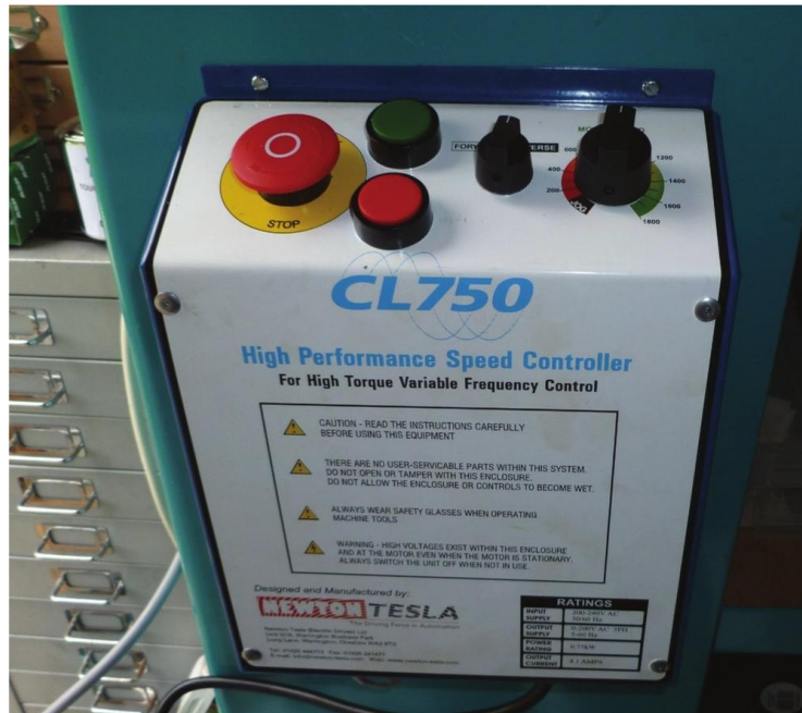
This inverter is designed for mounting on the front of the lathe.
