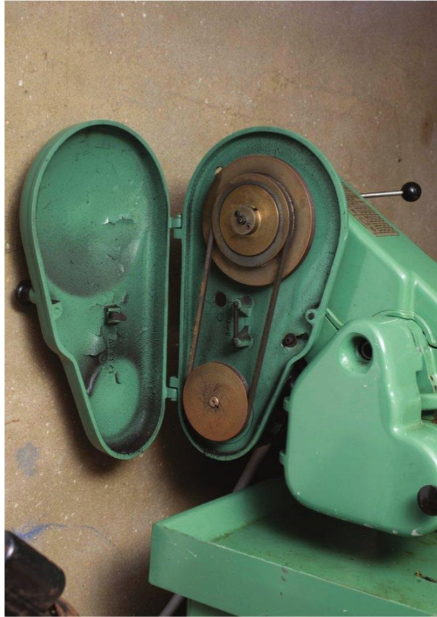
This particular lathe has a two-step motor pulley and countershaft, which doubles the available speeds.
