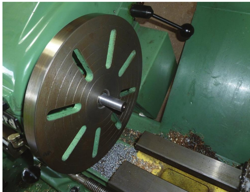
A stub arbor suitable for centralizing a locomotive wheel or flywheel.
