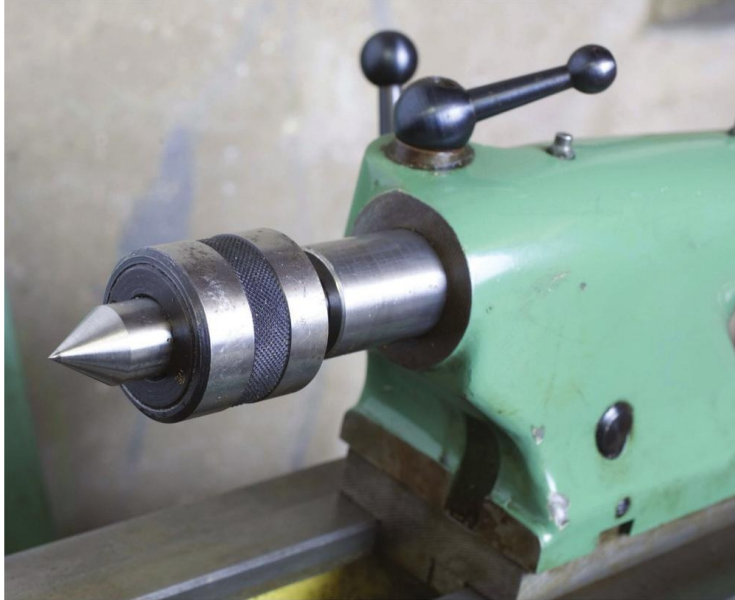
Tailstock running centre, so-called because it runs on ball races.
