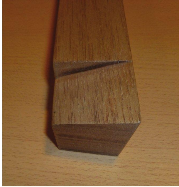
Top of the turning tool, showing the front and side clearance and the top rake.
