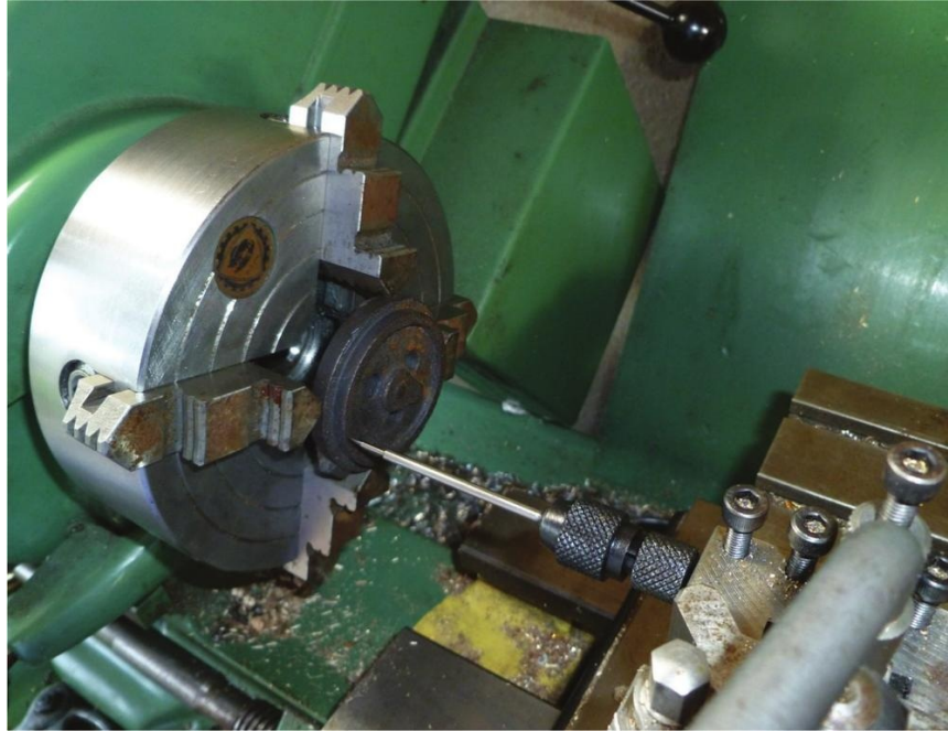
Using a commercial sticky pin to set work true.
