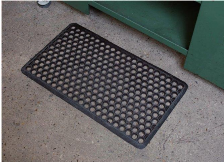
A suitable floor mat will allow swarf to drop through and help keep your feet warm in winter.
