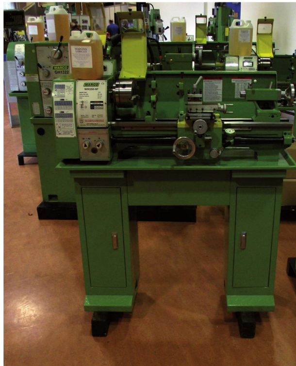
A medium-sized screwcutting lathe suitable for garden shed workshops.
