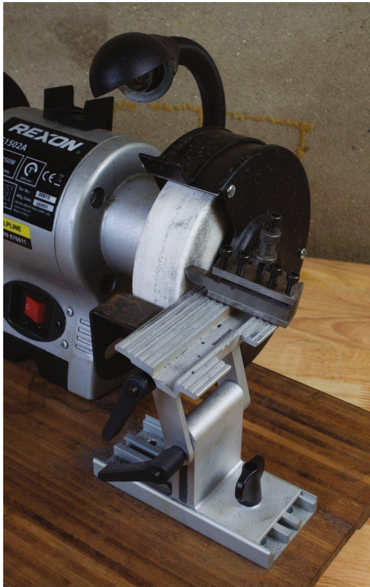
Grinding the first angle.
