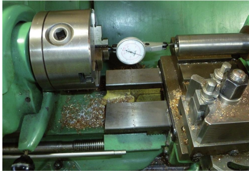
Align the tailstock by using a dial test indicator in the headstock.
