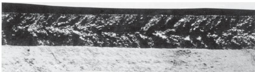
Fig. 7-2. An example of chevron markings on the fracture surface of a 25 mm thick steel plate involved in the collapse of an Allegheny County, Pennsylvania, oil tank in 1988. The origin of the fracture is to the left. (Courtesy of Dr. I. Le May.)
