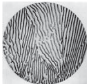
Coarse pearlite formed at about 720°C (Mag ~2,500×)
