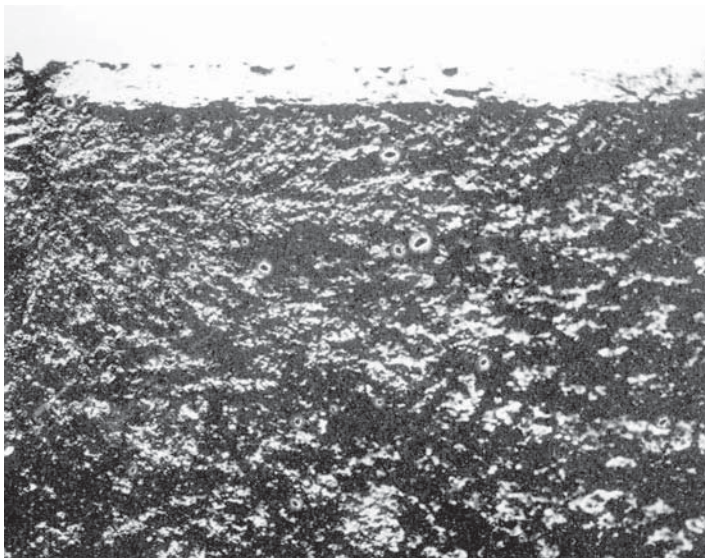
Fig. 7-4. Two flaws, upper left, 3 mm and 1.5 mm in radius, that existed prior to fracture of the critical eyebar of the Point Pleasant Bridge. (From NTSB, 3.)
