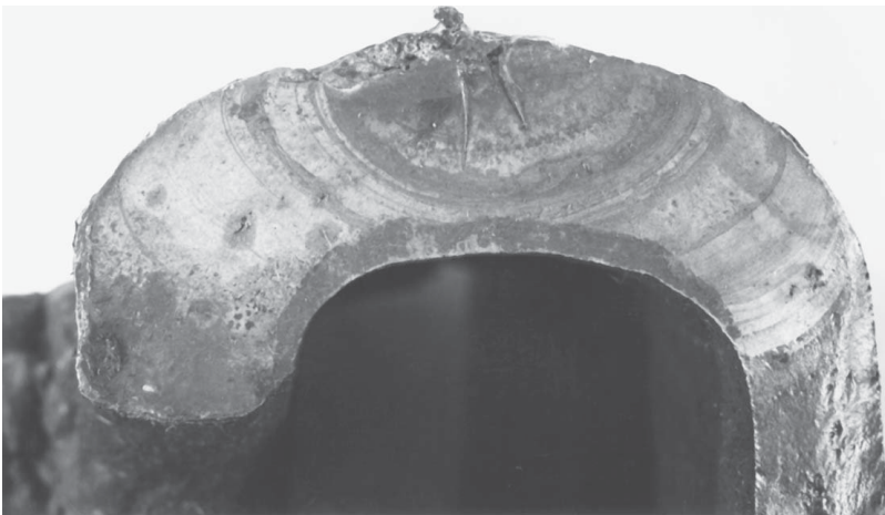
Fig. 10-31. Fatigue beach markings on a steel component. The markings are visible to the eye, and the fatigue crack initiated at a weld defect at the top of the figure.
