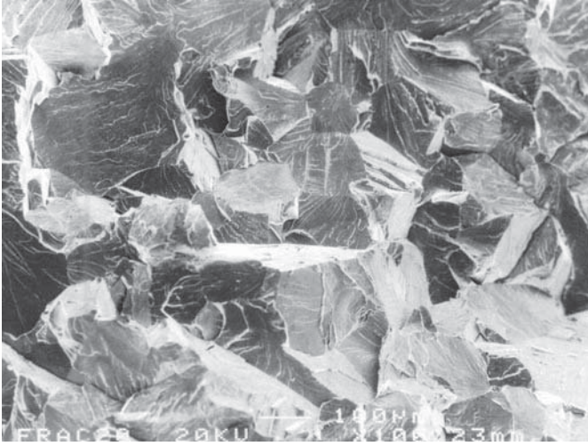
Fig. 7-3. Intergranular fracture in steel. (Courtesy of Dr. J. Gonzalez.)
