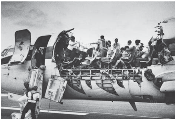
Fig. 1-7. General view showing the damage sustained by the Aloha Airlines Flight 737. (From NTSB, 10.)
