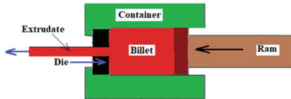
Fig. 7.3 Direct extrusion – working principle
