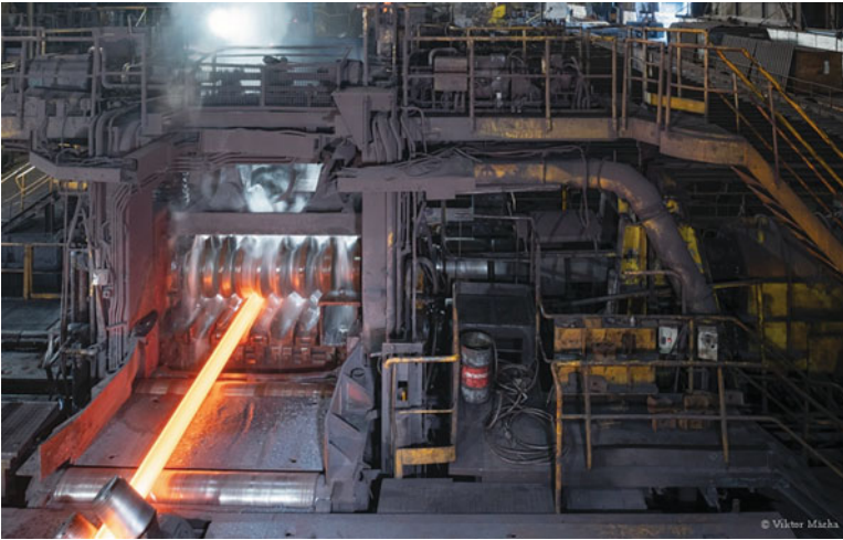
Fig. 5.3 Rolling process to produce hot steel bars. (Courtesy: Viktor Mácha/ viktormacha.com )
