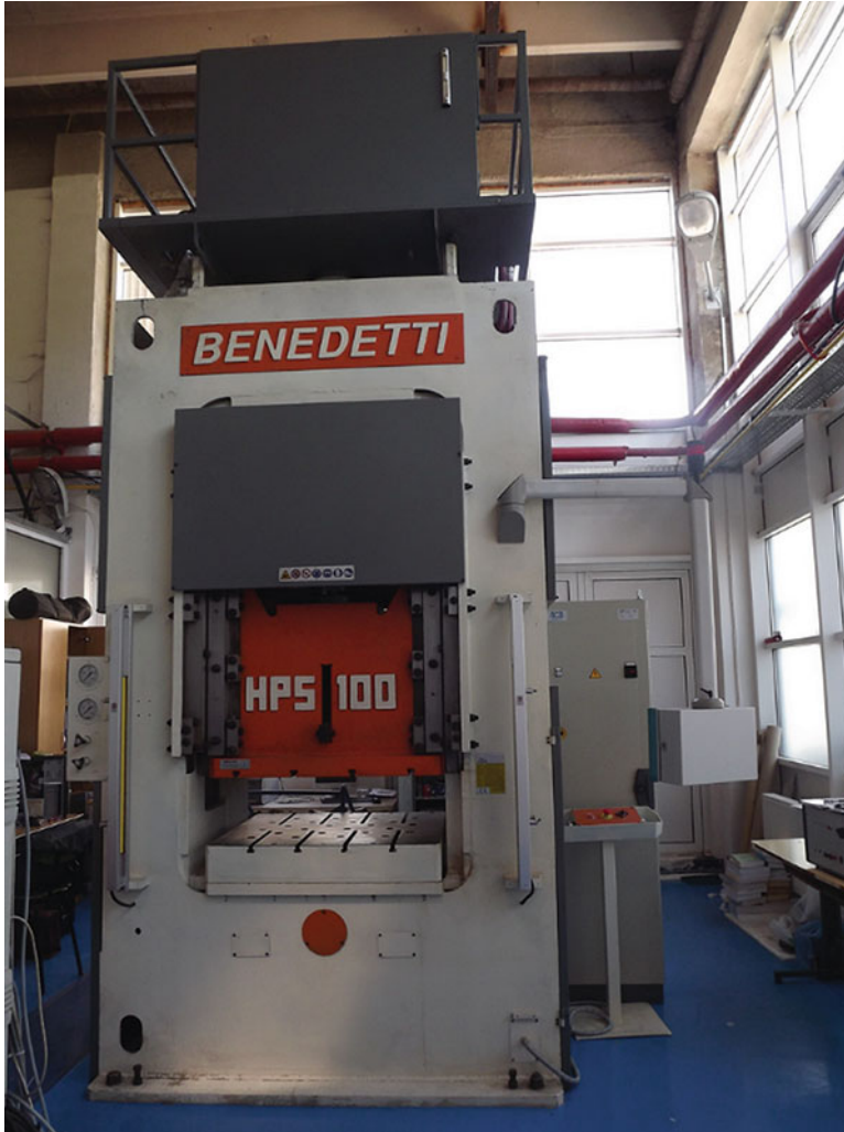
Fig. 12.4 The hydraulic press “Benedetti HPS 100” for deep drawing of metal sheets. (Courtesy: Department of Manufacturing Engineering, Technical University of Cluj-apoca)
