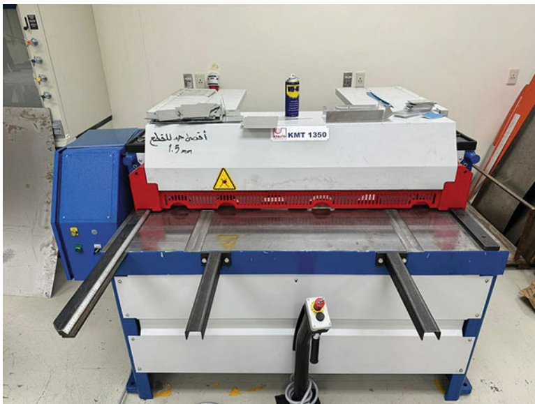
Fig. 10.3 A hydraulic shearing machine. (Courtesy: King Abdulaziz University)
