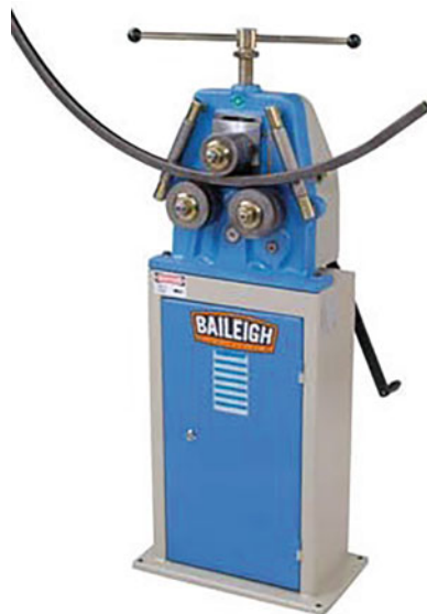
Fig. 11.7 A roll bending machine. (Courtesy: King Abdulaziz University)
