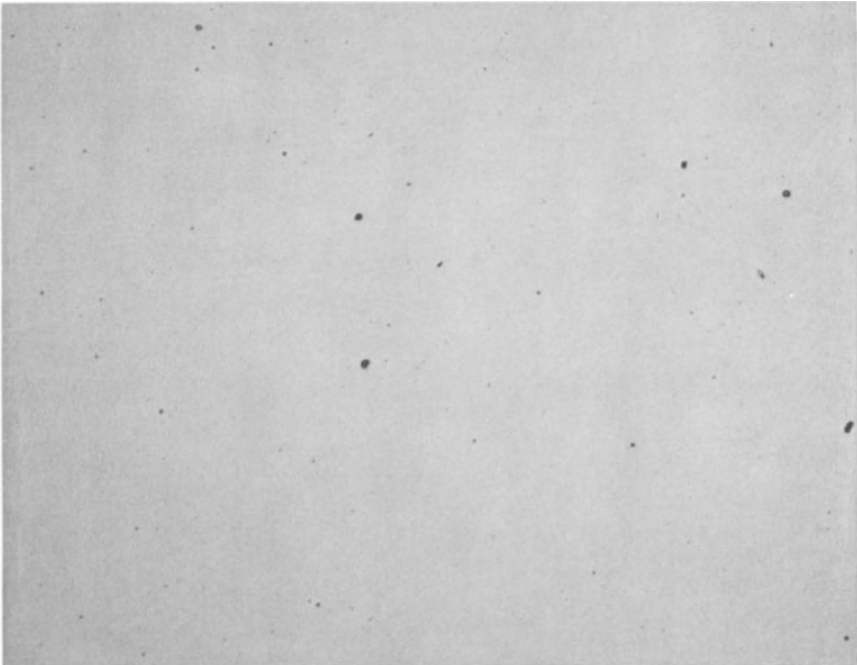
Fig. 27. As-cast Co-Cr-Mo alloy (100X). As-polished.
