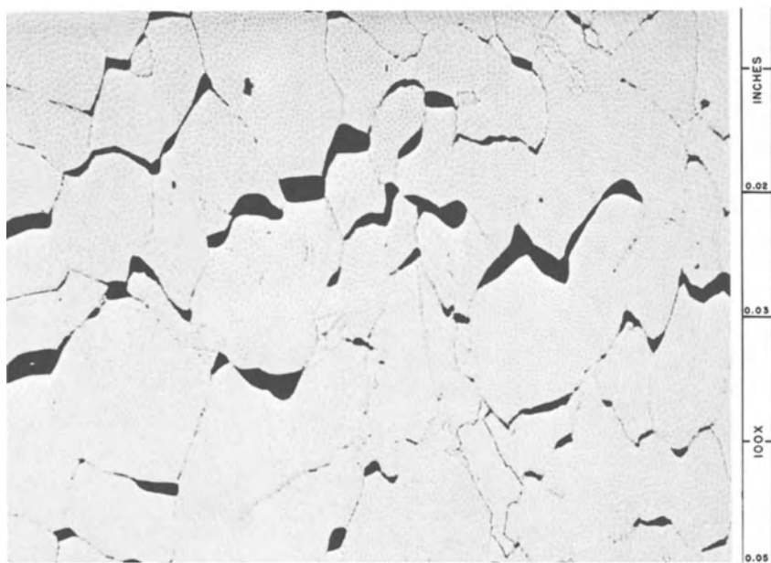
Fig. 5. Microcracks which may develop upon welding highly contaminated Nb—1 wt % Zr Alloy.
