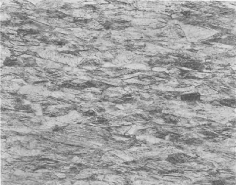
Fig. 3. Cold worked 316L stainless steel (100X), longitudinal section. Etchant: 10% ammonium persulfate, electrolytic.
