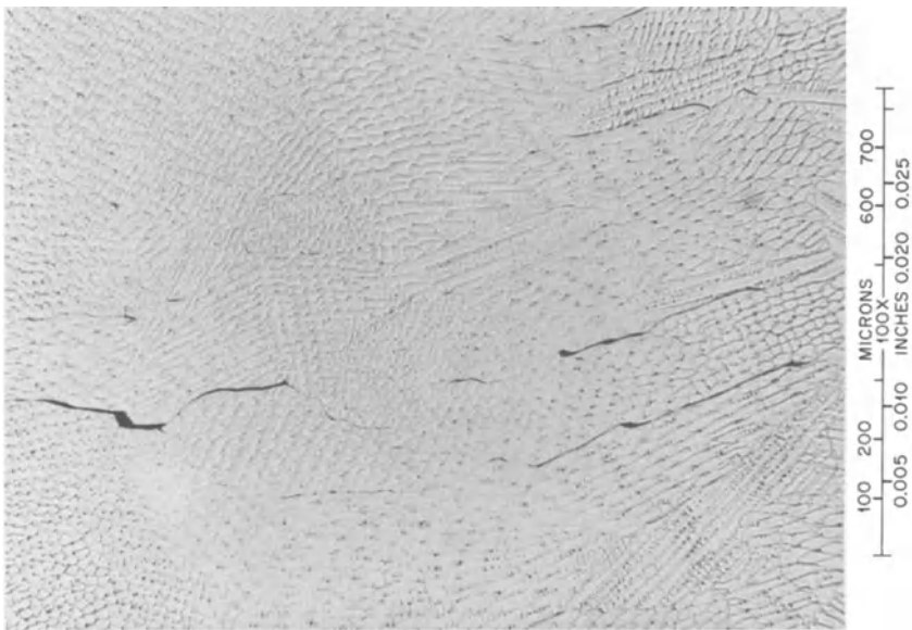
Fig. 1. Cracking in stainless steel weld metal resulting from an inadequate amount of delta-ferrite.
