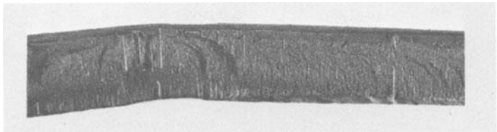
Fig. 5. Photograph of fractured and blued etch disk revealing inclusion stringers.
