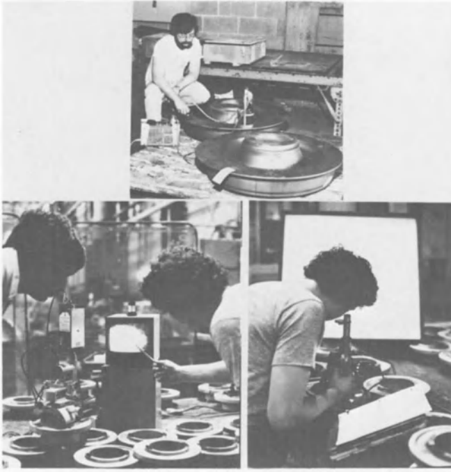
Fig. 10. Top: Large Ti forging being electropolished for direct examination of microstructure. Bottom: Rating ASTM grain size on Waspaloy forgings.
