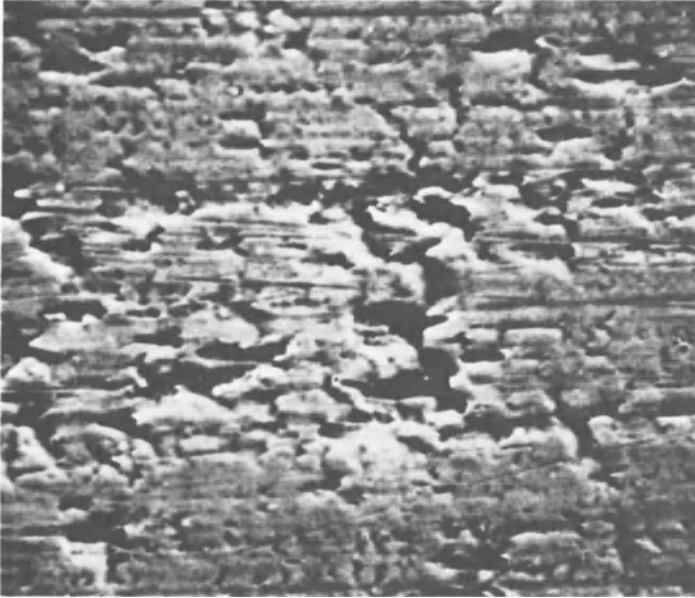
Fig. 5. SEM micrograph of the surface of EC aluminum wire, showing pockmarks probably caused by thick film lubricant pockets. A calcium stearate lubricant was used. Drawing axis is horizontal. 400X. (Reduced 10% for reproduction.)
