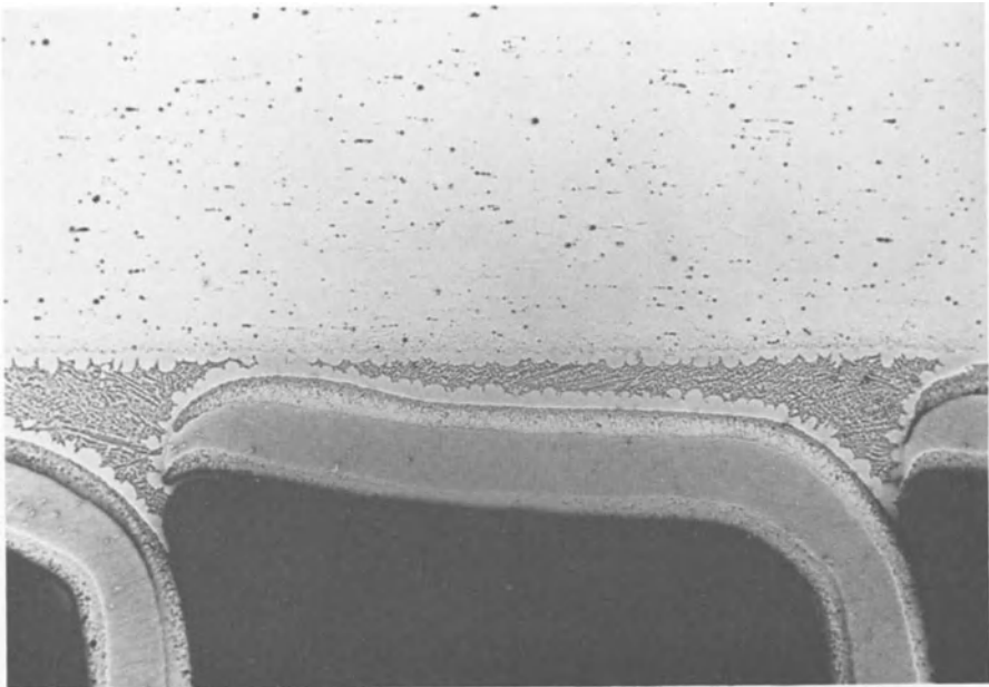
Fig. 14. Brazed high-conductivity fin showing edge protection of copper.
