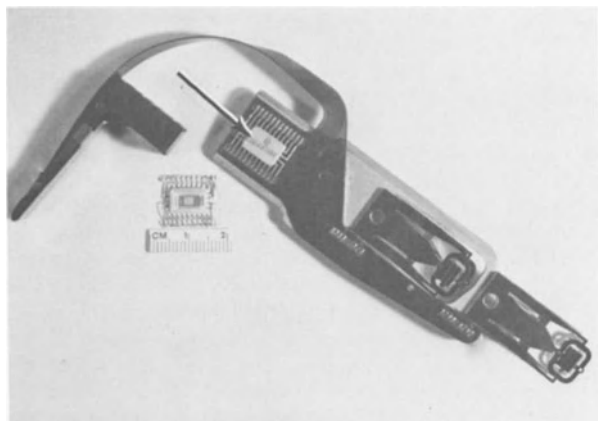
Fig. 14. An arm assembly with the integrated circuit soldered to it (see arrow). The IC shown with scale is the same type mounted on assembly arm. The top lid has been removed.
