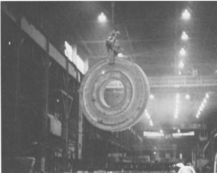
Fig. 4. Large bucket wheel forging being conveyed to quench tank. Mechanical test prolongations are located at the inner hub and outer rim.
