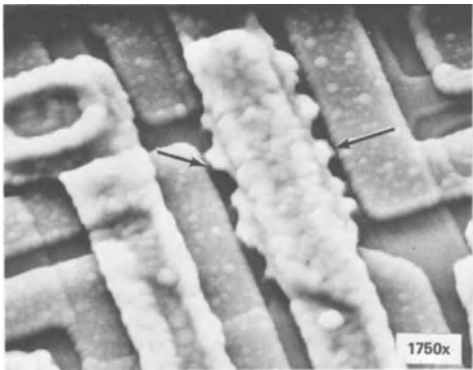
Fig. 19. Metallization that wasn't properly removed (see arrows). (Reduced 45% for reproduction.)
