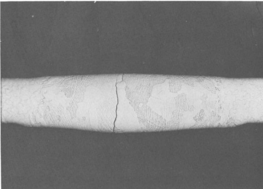
Fig. 7. Tungsten weld with intergranular cracking.
