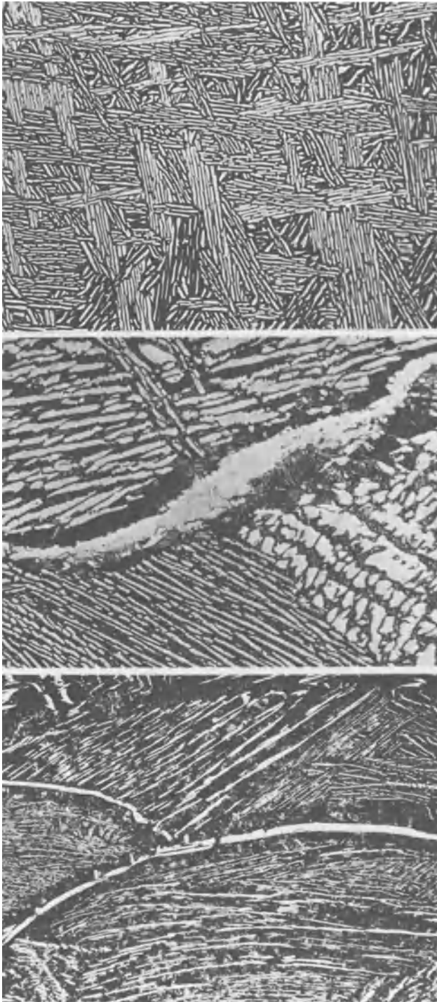
Fig. 4. Magnification .100X - Etchant: \text{NaOH}, \text{H}_2\text{H}_2\text{O}_2 . Examples of rejectable billet microstructures: A. Stringy alpha and grain boundary outlining. B. Blocky alpha and segregation at grain boundary. C. Widmanstatten structure. (Reduced 20% for reproduction.)
