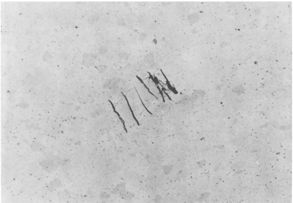
Fig. 14. Microcracks in a powder product due to surface oxidation on the powder.
