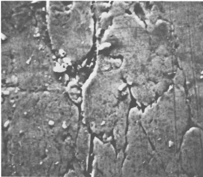
Fig. 6. SEM micrograph of the surface of EC aluminum wire, as shown from the condition of Fig. 1 with a compounded mineral oil lubricant. Drawing axis is vertical. 400X. (Reduced 10% for reproduction.)
