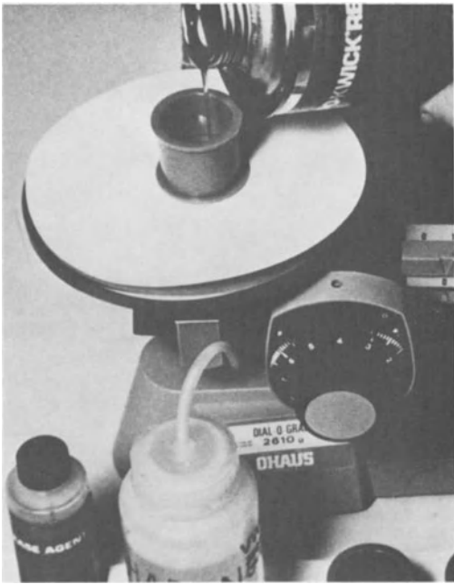
Fig. 4. The technique for encapsulating a part in epoxy.
