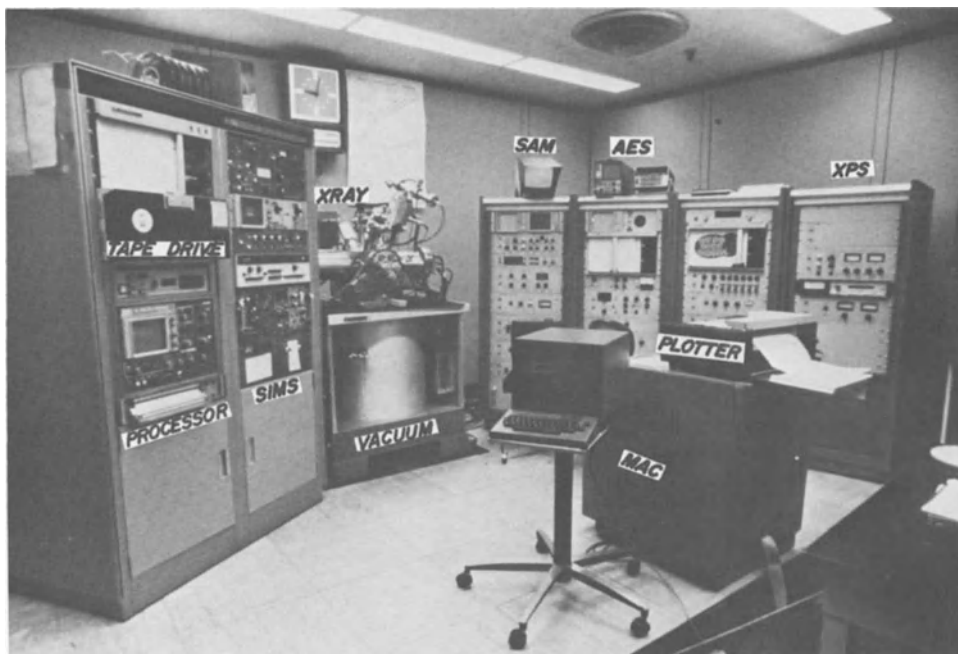
Fig. 4. Overall view of surface analysis equipment showing SIMS electronics, vacuum chamber, SAM/XPS/AES electronics, computer-plotter system.
