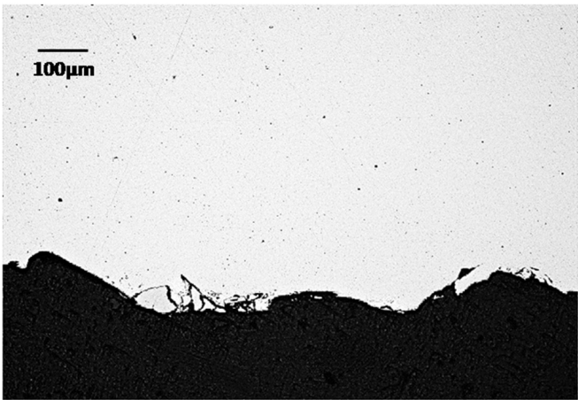
Fig. 11.1.16 Micrograph of the cage sample showing surface erosion and removal of material. Unetched.
