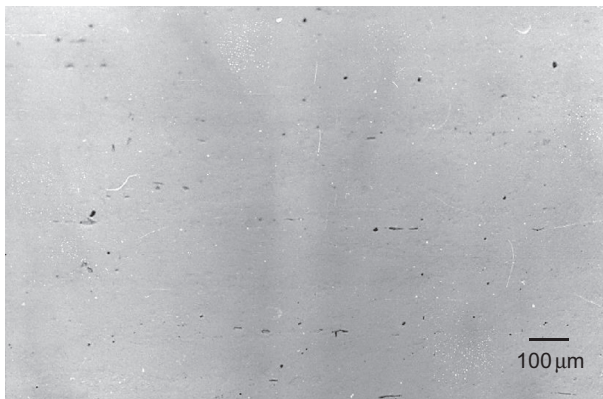
Fig. 12.3.5 Micrograph of longitudinal section of the race sample showing a number of nonmetallic inclusions. Unetched.
