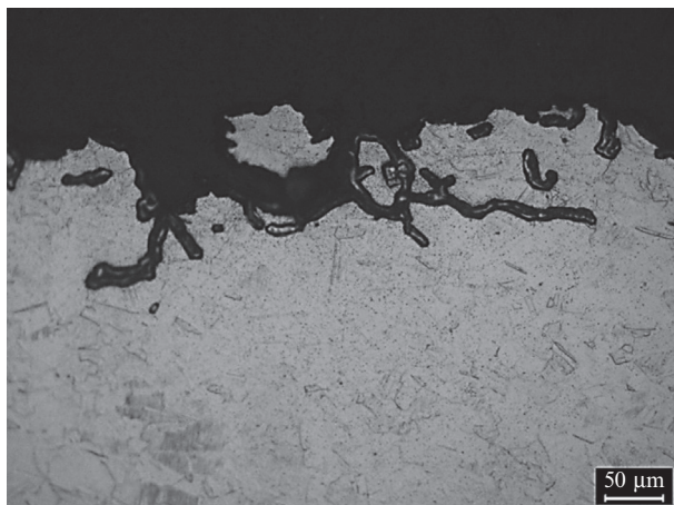
Fig. 10.4.14 Micrograph of a section perpendicular to the fracture surface of the cartridge sample showing a number of secondary intergranular branching cracks. Etchant: Acidified potassium dichromate.
