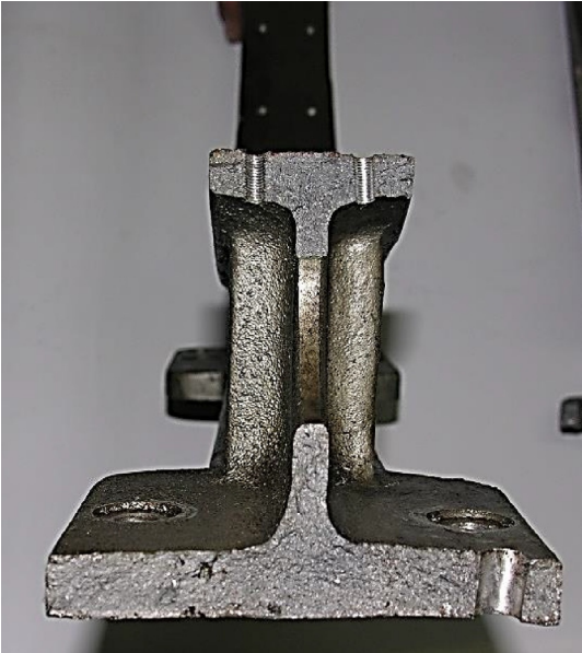
Fig. 7.3.2 Fracture surface of the failed component showing a mixed mode of granular and fibrous fracture feature.
