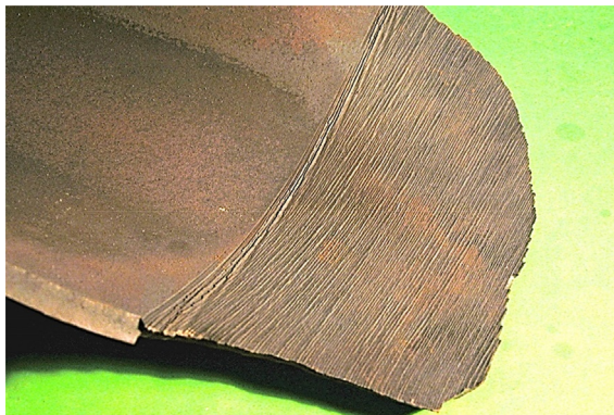
Fig. 7.2.2 Close up of the inner side of the failed part of the pipe showing deep-machined grooves especially at the junction of the grooving and the smooth region.
