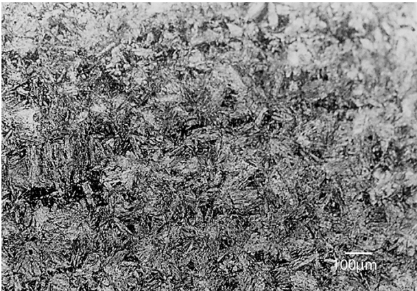
Fig. 11.4.4 Micrograph of longitudinal section of the coupling shaft showing a tempered martensite microstructure in the core. Etchant: 2% nital.
