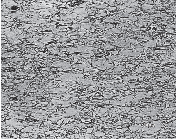
Fig. 4.4.6 Micrograph of longitudinal section of the sample showing deformed fine alpha grains. Etchant: Acidified potassium dichromate.
