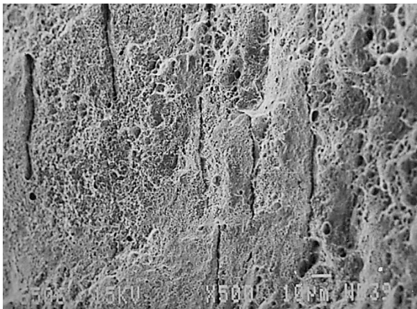
Fig. 4.4.3 SEM fractograph showing tear-like features with their longitudinal axis parallel to the direction of drawing near the origin.
