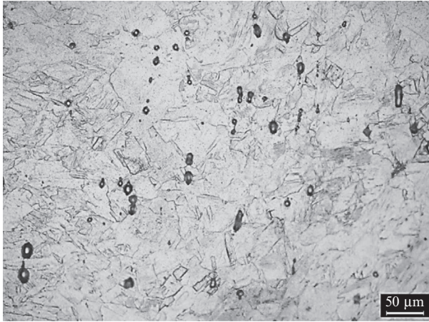
Fig. 10.4.12 Micrograph of a section from the U-bend of the cartridge sample showing equiaxed alpha grains with some strain markings and zinc sulfide inclusions. Etchant: Acidified potassium dichromate.
