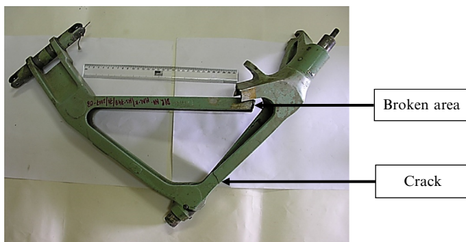
Fig. 10.3.1 The failed lever assembly in the as-received condition.
