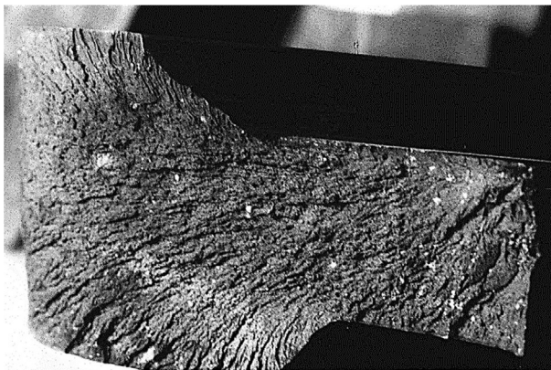
Fig. 5.7.3 Fracture surface at location 'B' showing chevron marks.
