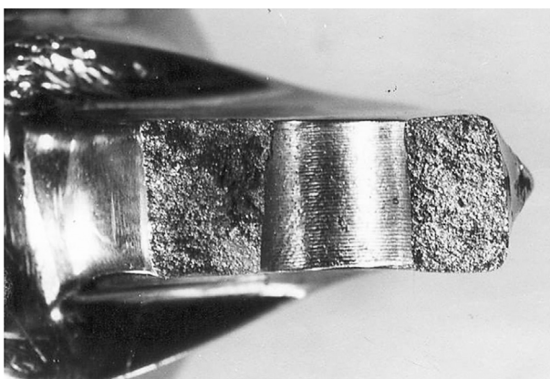
Fig. 4.1.2 Fracture surface showing a coarse and crystalline fracture.
