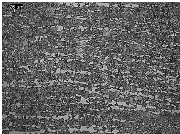
Fig. 5.3.9 Micrograph of a section of the sample showing aligned \delta -ferrite in a matrix of tempered martensite. Etchant: aqua regia.
