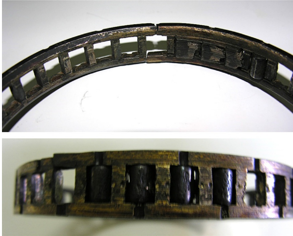
Fig. 11.1.5 Outer and inner surfaces of the cage showing surface wear and breakage.
