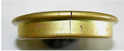
Fig. 10.4.2 Side view of a sample of the failed cartridge showing the crack.
