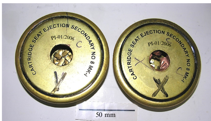
Fig. 10.4.1 Failed cartridges in the as-received condition.
