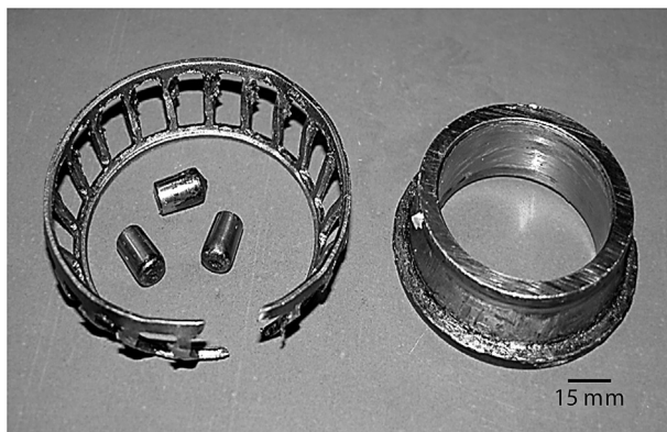
Fig. 11.3.3 The outer bearing in the as-received condition showing the inner race, the cage, and the rollers.
