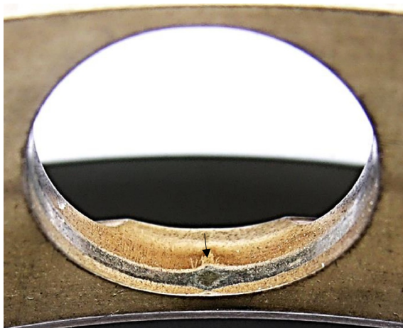
Fig. 8.4.4 Magnified image of the track mark and the dent mark with pointed ends.
