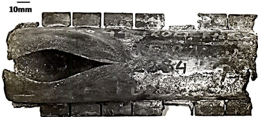
Fig. 7.4.1 Failed water wall tube in the as-received condition.
