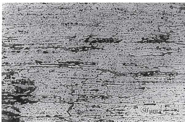
Fig. 9.4.6 Micrograph of longitudinal section of the defective tube sample showing large number of undissolved particles and grain boundary precipitation of \text{CuAl}_2 near the corroded surface. Etchant: Keller's reagent.
