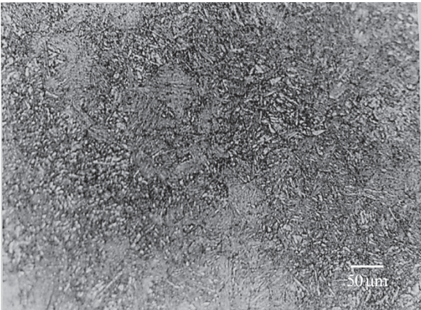
Fig. 10.1.4 Micrograph of longitudinal section of the screw showing a tempered martensite structure. Etchant: 2% nital.
