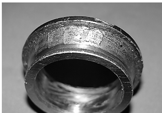
Fig. 11.3.4 The outer surface of the inner race showing dent marks corresponding to the locations of the rollers.
