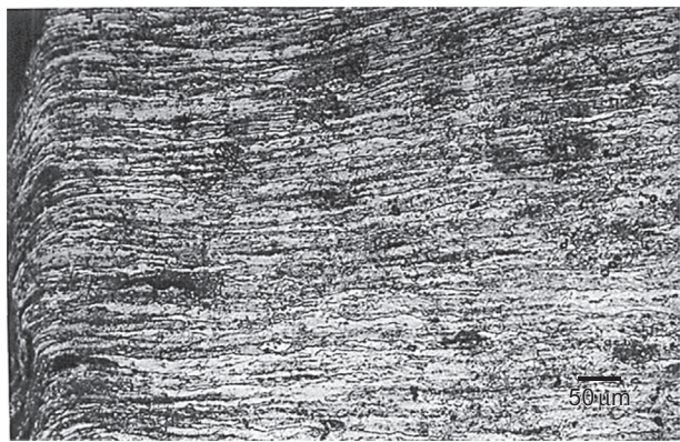
Fig. 7.4.4 Micrograph of a transverse section of the sample near the region of maximum deformation showing severely deformed ferrite and globular carbides. Etchant: 2% nital.
