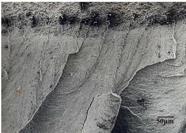
Fig. 5.2.3 SEM fractograph showing fracture initiating from the inner surface.
