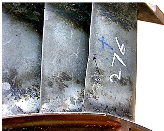
Fig. 12.5.3 Close-up view of another segment of the vanes showing cracks near the trailing edge on the convex side.
