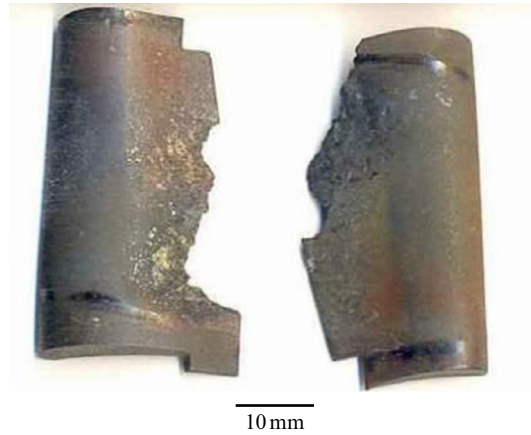
Fig. 12.2.1 Damaged vanes showing degradation and roughness on the surface of the convex side.
