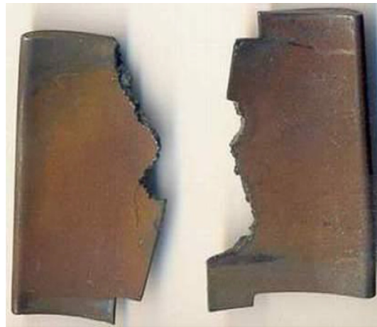
Fig. 12.2.2 Damaged vanes showing cracks and oxidation on the surface of the concave side.
