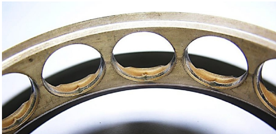
Fig. 8.4.3 The broken cage in the as-received condition showing the eroded track marks of the ball within each circular slot and the dent marks at two opposite locations.
