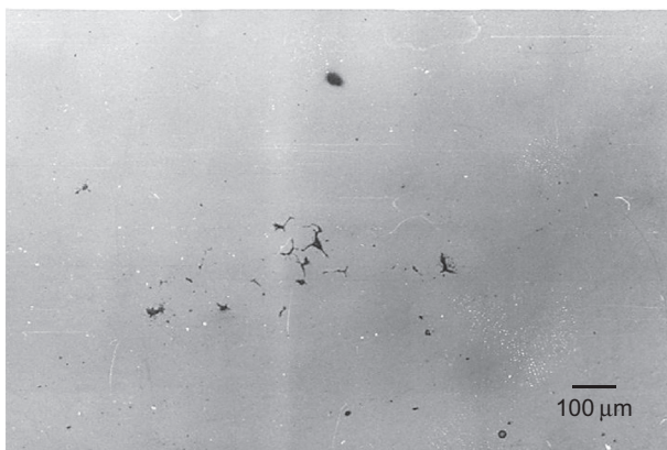
Fig. 12.3.8 Micrograph of a section of the race sample showing wedge-shaped microcavities. Unetched.
