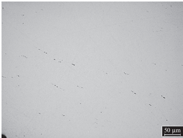
Fig. 10.4.10 Micrograph of a section from the cartridge sample showing strings of zinc sulfide inclusions. Unetched.
