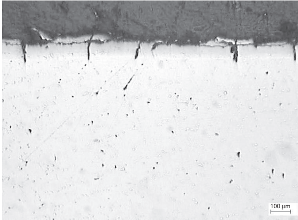
Fig. 12.2.4 Micrograph of the vane sample showing cracks on the surface coating on the convex side near the trailing edge of the aerofoil. Unetched.
