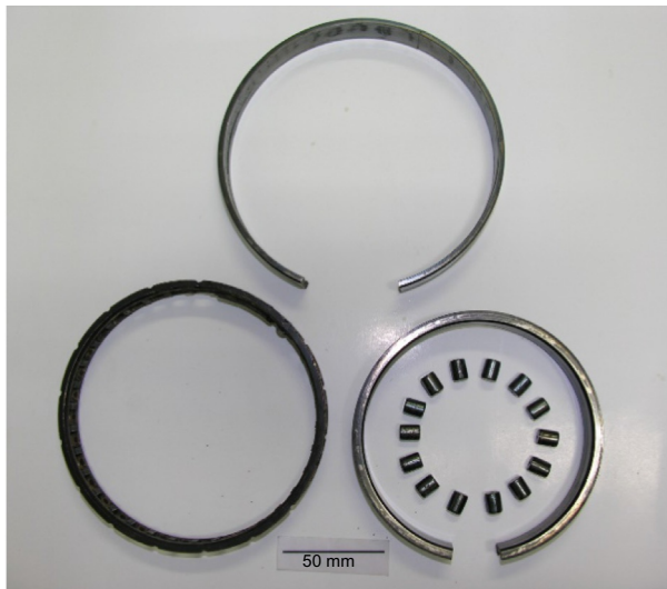
Fig. 11.1.1 Failed bearing showing the outer race, the inner race, the rollers, and the cage in the as-received condition.
