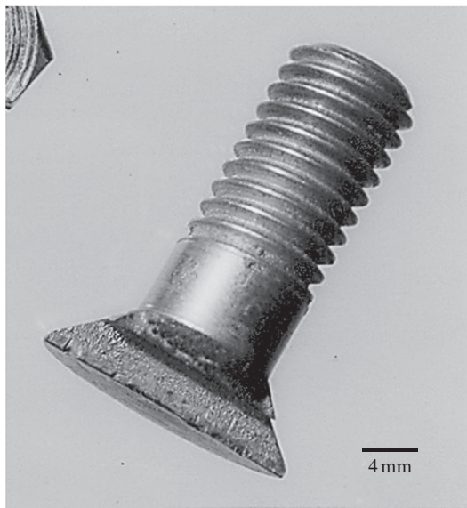
Fig. 10.1.1 The failed screw in the as-received condition.
