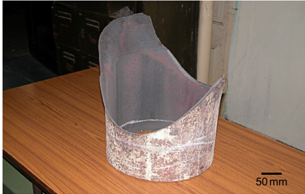
Fig. 7.2.1 The burst pipe in the as-received condition.
