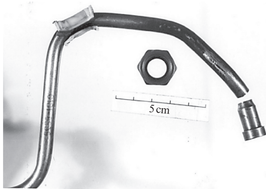
Fig. 9.1.1 The segment of the failed fuel pipe in the as-received condition.
