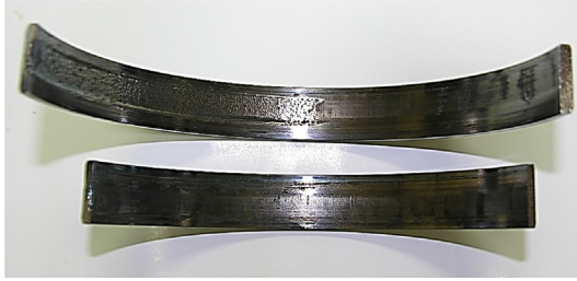
Fig. 11.1.2 Inner surface of the outer race showing the damage concentrated to one side
