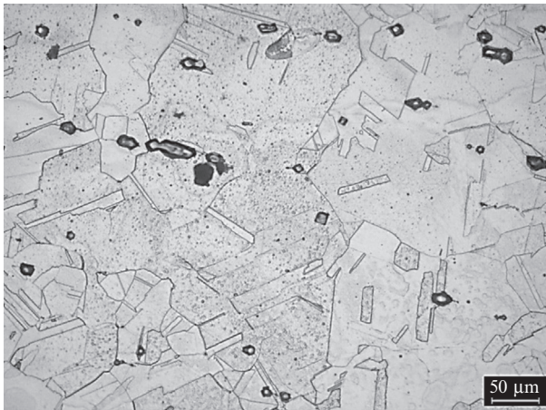
Fig. 10.4.13 Micrograph of a section from the lid of the cartridge sample showing equiaxed alpha grains with annealing twins and zinc sulfide inclusions. Etchant: Acidified potassium dichromate.
