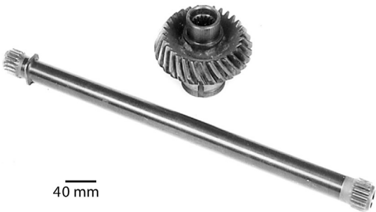
Fig. 11.4.1 The worn out coupling shaft and bevel gear in the as-received condition.
