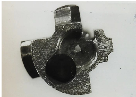
Fig. 5.6.2 Close-up view of the failed component showing cracks around the firing pin retainer hole adjacent to the extractor recess.
