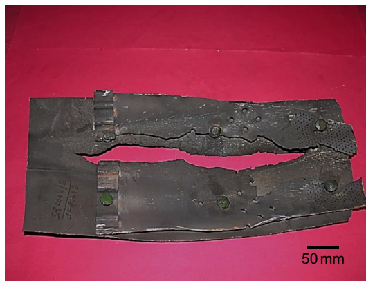
Fig. 12.4.1 Failed jet nozzle casing in the as-received condition.
