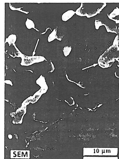
Figure 3.74 Fracture surface showing a dendritic appearance, associated with fracture of a liquid film between dendrites. This was a crack in a Waspaloy alloy immediately adjacent to an electron beam weld. The crack shows the characteristics of fracture in the pasty state, namely, the surface consisting of droplets and drawn-out peaks. (From Engel and Klingele. 10 )
