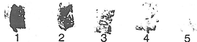
Figure 1C.2 Successive replicas (numbered 1 to 5) stripped from a rusted steel fracture surface. Note that the first replica stripped contains the most surface contaminants, while the last replica stripped is the cleanest. (Approximate size.)
