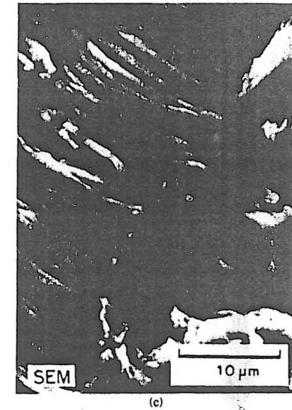
Figure 3.62 Examples of fatigue fractures showing secondary cracks associated with striations. (a) From a tantalum heat-exchanger tube. The rough surface appearance is due to secondary cracking caused by high-cycle low-amplitude fatigue. (Courtesy of M. E. Blum, FMC Corporation; adapted from Kerlins and Phillips. 9 ) (b) From steel (0.38% C, 1.19% Si, 1.23% Mn, and 0.023% P) axle broken in service. (From Henry and Horstmann. 7 ) (c) From steel containing 0.10% C, 0.27% Si, 0.43% Mn, 0.027% P, and 0.022% S. (From Henry and Horstmann. 7 )
