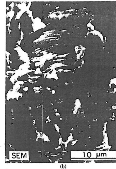
Figure 3.62 Examples of fatigue fractures showing secondary cracks associated with striations. (a) From a tantalum heat-exchanger tube. The rough surface appearance is due to secondary cracking caused by high-cycle low-amplitude fatigue. (Courtesy of M. E. Blum, FMC Corporation; adapted from Kerlins and Phillips. 9 ) (b) From steel (0.38% C, 1.19% Si, 1.23% Mn, and 0.023% P) axle broken in service. (From Henry and Horstmann. 7 ) (c) From steel containing 0.10% C, 0.27% Si, 0.43% Mn, 0.027% P, and 0.022% S. (From Henry and Horstmann. 7 )
