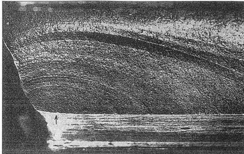
Fig. 4.8b Distinct beach marks due to fatigue, originating from the root radius zone of gear tooth ( \times 4 )
