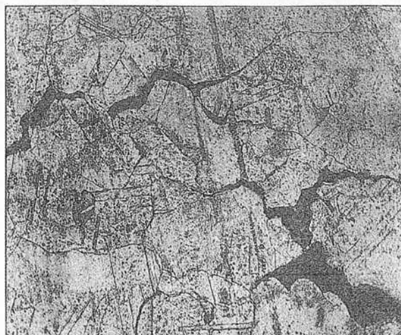
Fig. 8.112 Triple point cracks and creep voids ( \times 400 )
