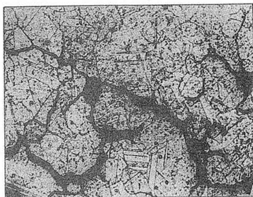
Fig. 8.109 Voids and intercrystalline fissures ( \times 100 )
