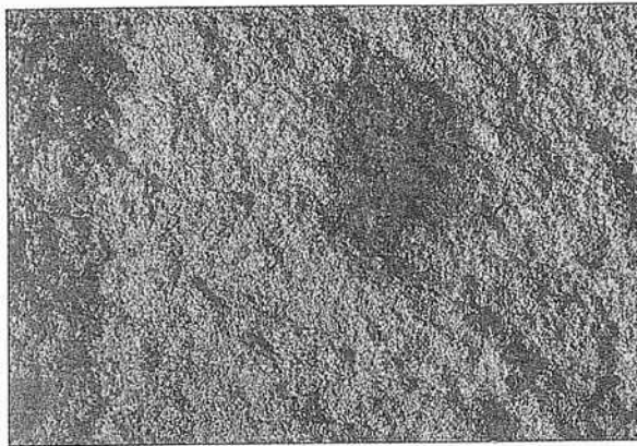
Fig. 8.76 Black zones developed in fractured surface when exposed to atmosphere, due to the presence of flux inclusions ( \times 1 )
