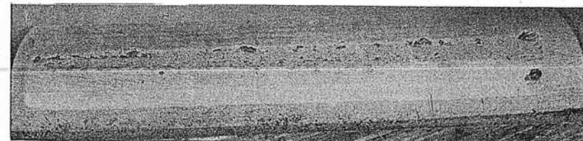
Fig. 4.14 Spalled tooth surface of a failed gear in design testing
