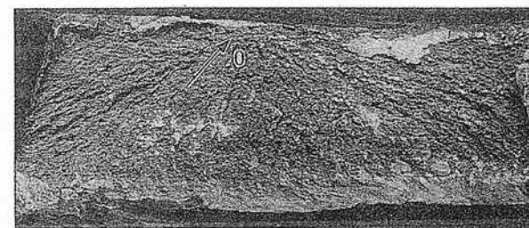
Fig. 8.14 Enlarged view of fracture 'A' in Fig. 8.12 showing 'Chevron' pattern of high velocity brittle fracture with its origin at 'O' ( \times 2 )
