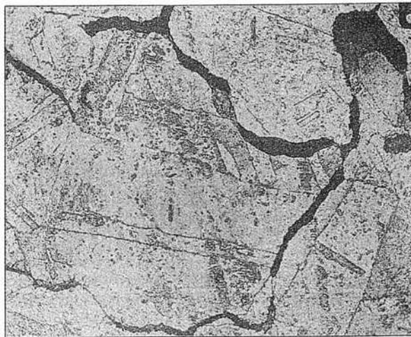
Fig. 4.29 Creep voids at the grain boundaries and cracking at triple points in the microstructure of a creep failed Cu-Cr material ( \times 400 )
