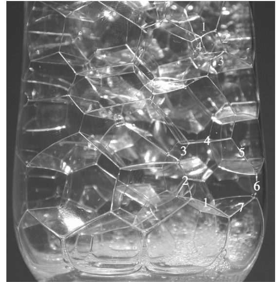
Figure 8.1(a) Soap grains simulate metal grains.
