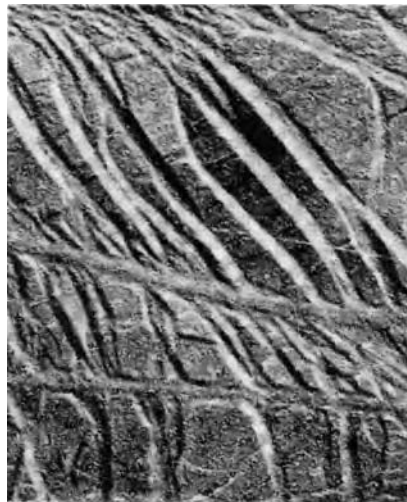
Fig. 15 Stretcher strains (Lüders bands) in rimmed 1008 steel. Source: Ref 9
