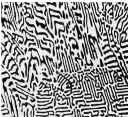
Fig. 8 Irregular “Chinese script” eutectic consisting of faceted \text{Mg}_2\text{Sn} phase (dark) in a magnesium matrix. Etched with glycol. Original magnification: 250 \times . Source: Ref 2
