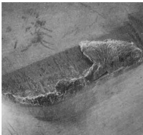
Fig. 13 Built-up edge on a cemented carbide tool. The built-up edge was produced during the low-speed machining of a nickel-base alloy. Original magnification: 20 \times . Source: Ref 7
