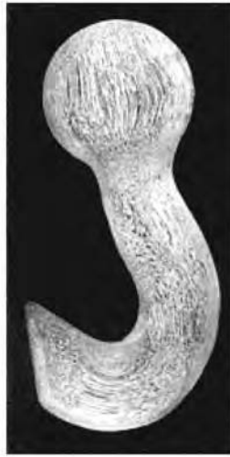
Etched 4140 Forging Showing Grain Flow
