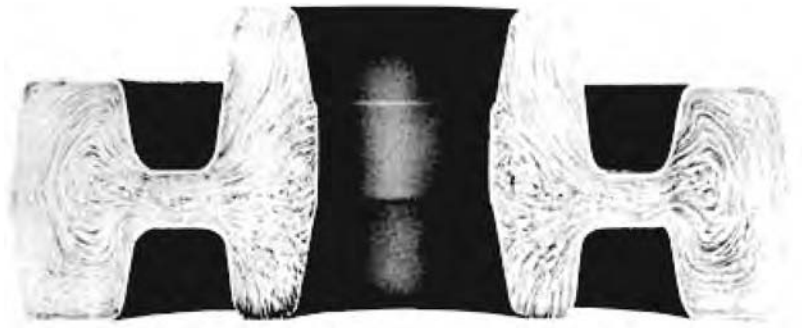
Fig. 4 Grain flow from forging. Source: Ref 5
