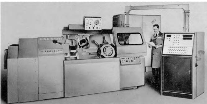
Fig. 20 A dual-turret numerically controlled turning center with 16 tool stations. Courtesy of Cincinnati Milacron. Source: Ref 9
