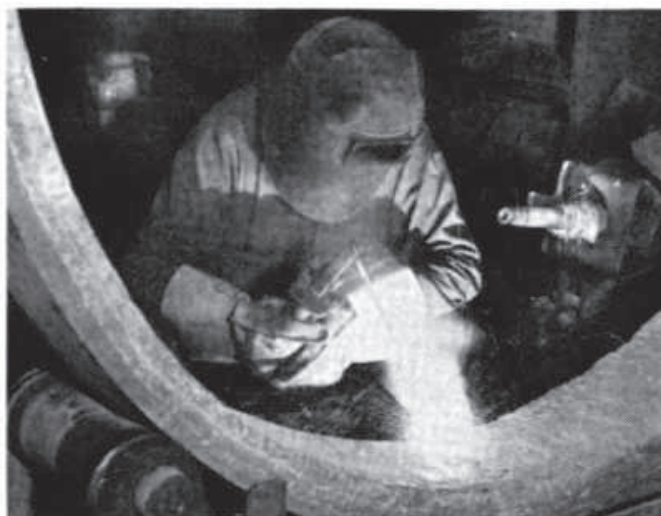
Fig. 19-9. Long-life chromium carbide hardsurfacing is deposited on large die ring worn from severe abrasion and moderate impact.
