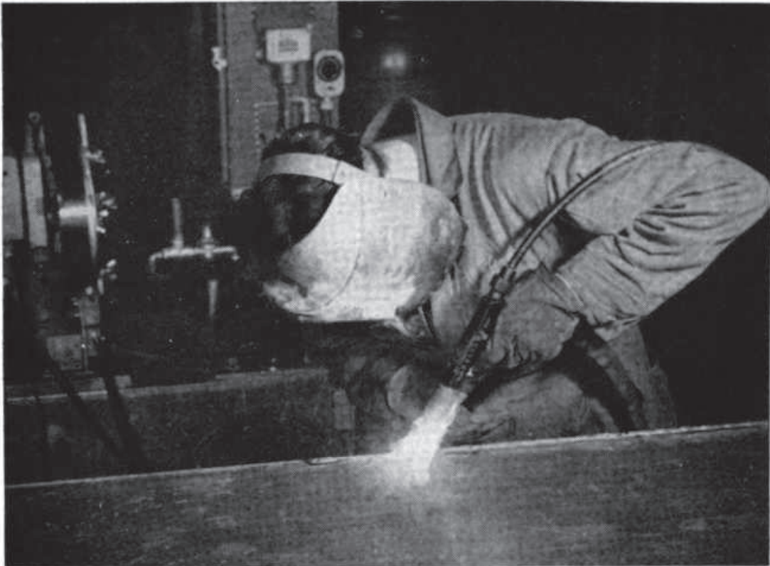
Fig. 6-4. (Above) In this semi-automatic MIG (metal inert-gas shielded-arc) welding operation, the continuous consumable electrode is fed mechanically but the gun is held and guided manually.
