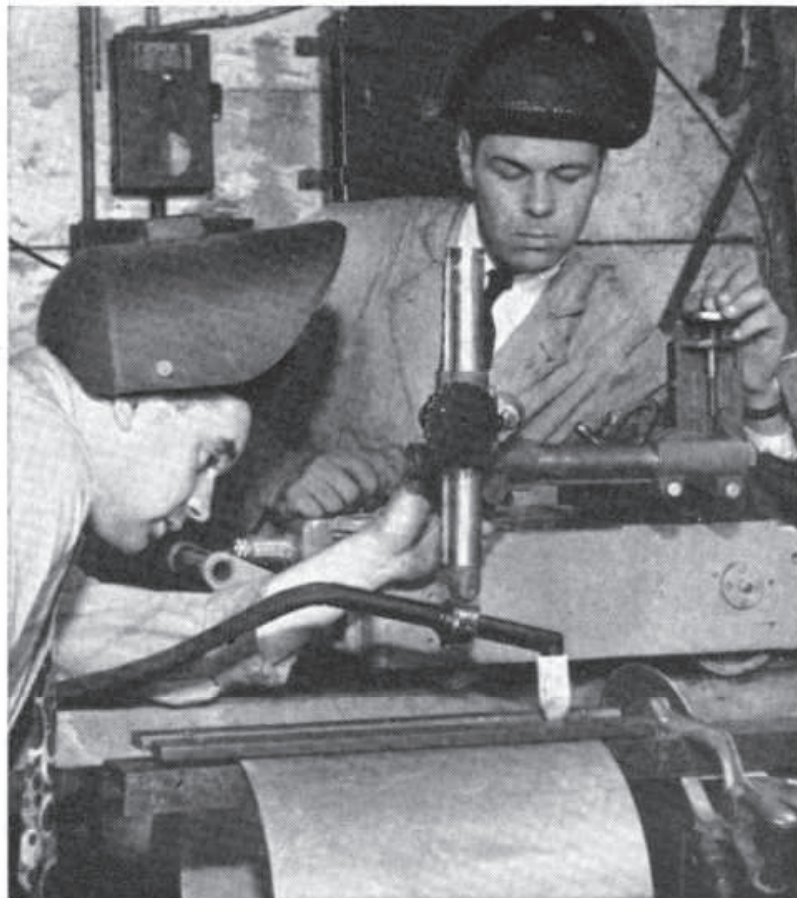
Fig. 17-1. An automatic inert-arc setup for welding aluminum containers.
