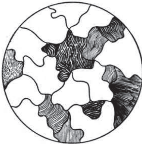
Fig. 7-10. Steel having less than 0.83% carbon has a structure composed of ferrite and pearlite.
