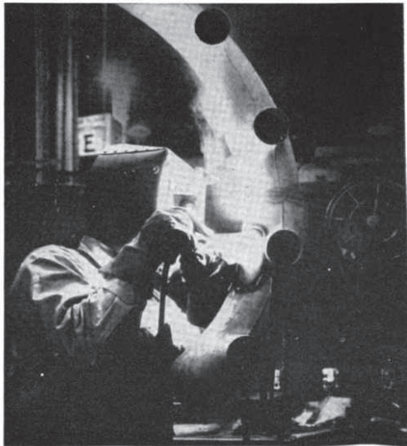
Fig. 15-2. Shielded-arc welding is used extensively in making strong, ductile joints in most grades of stainless steel.
