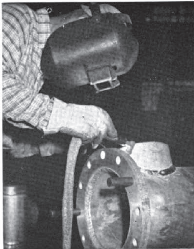
Fig. 6-5. (Right) With the TIG process, a contoured nipple is welded to an aluminum 3003 pipe header. The welding rod is held in the operator's left hand. Two passes completed this joint.
