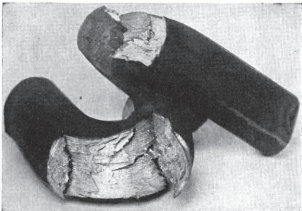
Fig. 4-9. Wrought iron is characterized by its tough, fibrous structure.
