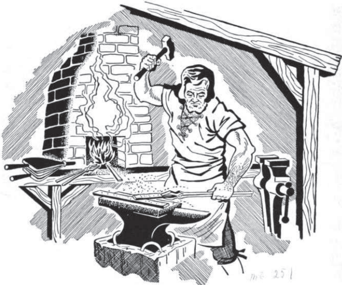
Fig. 1-1. Forging is one of our oldest crafts. From this shaping of metal by heat and hammering came the idea of forcing metal together by forge welding, a process which has become obsolete for most purposes.
