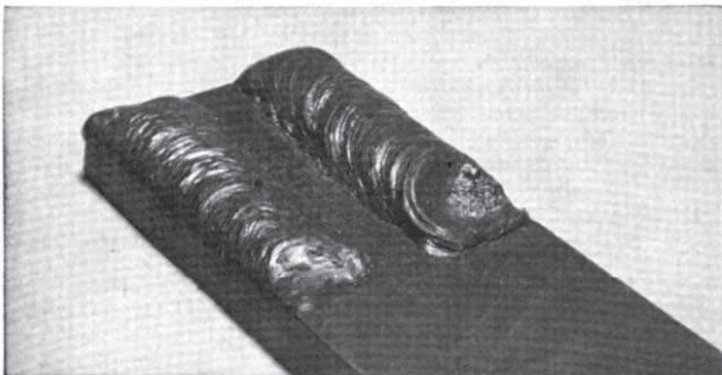
Fig. 16-5. Beads of high-manganese steel. Left, made with shielded-arc coated electrode; right, with bare metal electrode.
