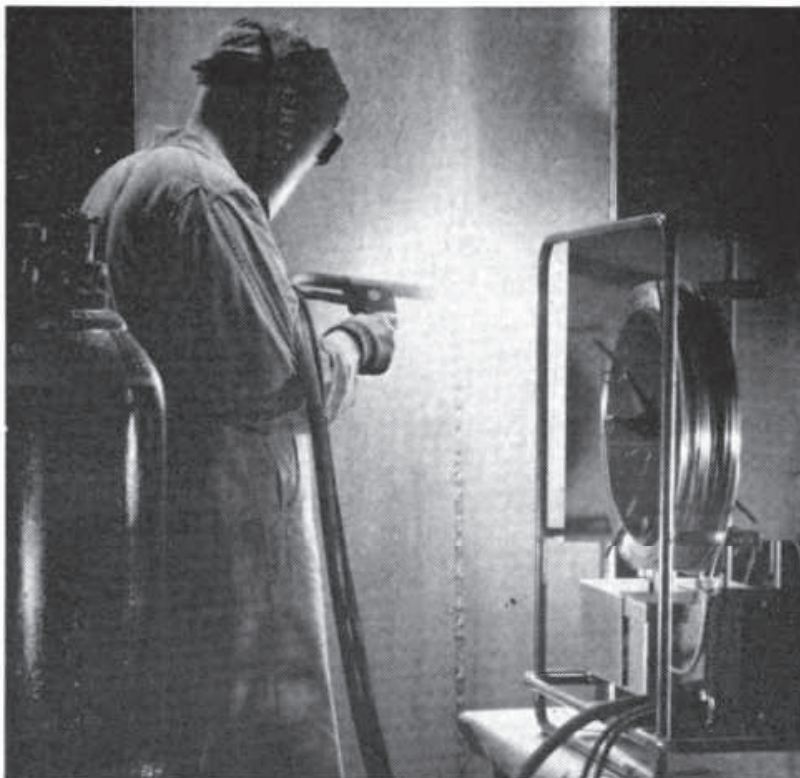
Fig. 17-2. Vertical welding aluminum by the semi-automatic inert-arc consumable electrode (MIG) process.
