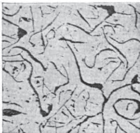
Fig. 4-6. Gray cast iron's strength is limited due to the stringer arrangement of its graphitic carbon content, 100x.
