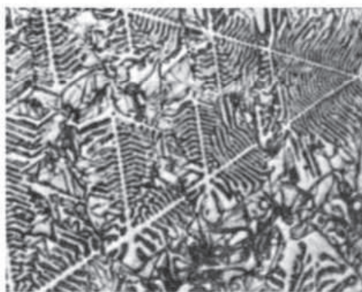
Fig. 18-4. Tungsten carbide hardsurfacing deposit viewed at 1000X.
