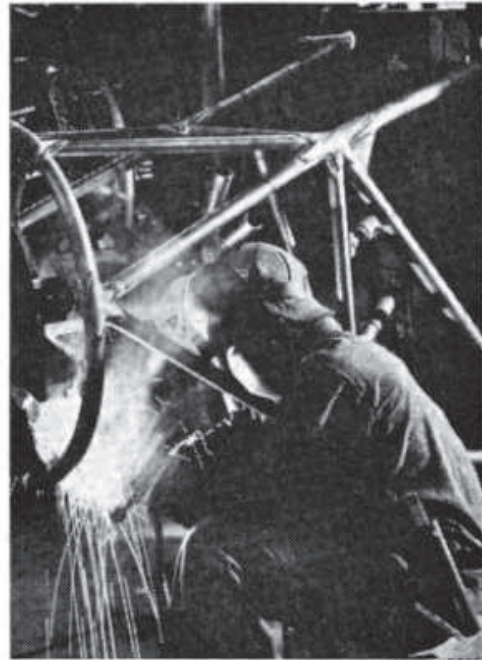
Fig. 13-9. Airplane engine mount of SAE 4130 chromium-molybdenum steel, welded with E-10013 electrode that gives a high tensile strength weld.
