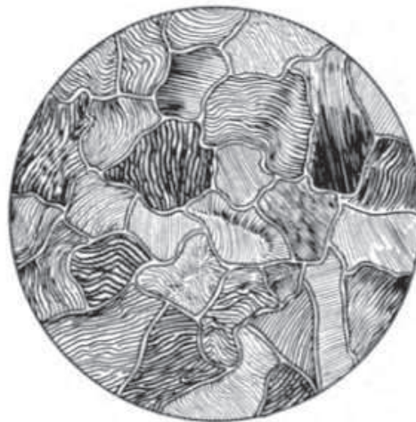
Fig. 7-11. Steel having more than 0.83% carbon has a structure of pearlite surrounded by iron carbide.
