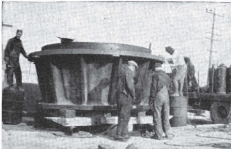
Fig. 14-3. When a large iron casting cannot be preheated, shielded-arc welding may be used to successfully repair the casting.
