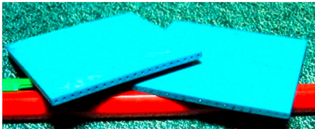
FIGURE 12.2 Composite samples. Left: Sample with holes. Right: Same sample with iron wires inside the holes.
